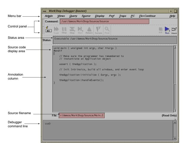
Figure 1-1 The WorkShop Debugger Main View Window
