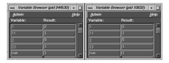
Figure 10-3 Comparing Variable Values from Two Processes
