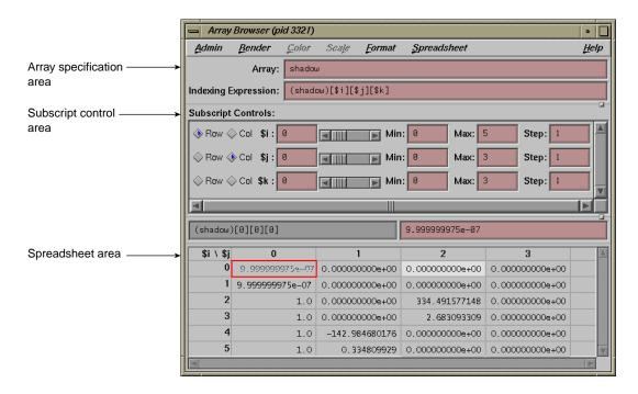
Figure 4-13 Array Browser Window for shadow Matrix
