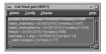
Figure 9-2 Call Stack at Boundary Overrun Warning
