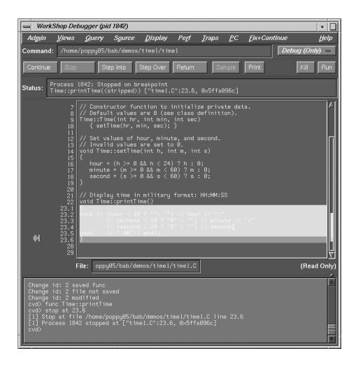
Figure 8-4 Stopping after Breakpoints in Redefined Code
