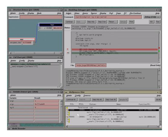
Figure 10-5 Reaching the MPI application breakpoint screen display
