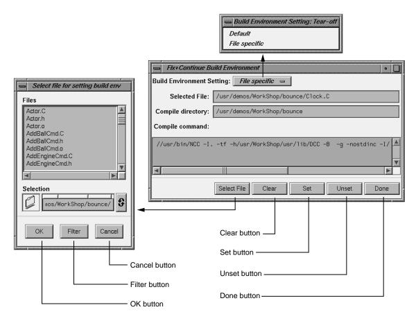
Figure A-63 Fix+Continue Build Environment Window
