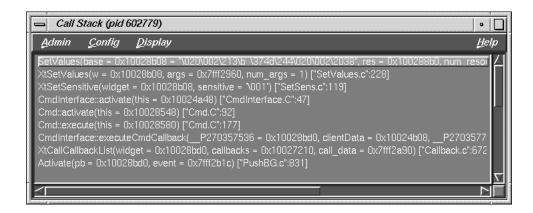
Figure 11-8 Breakpoint Results Displayed by the Call Stack
