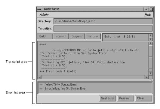
Figure B-2 Build View Window with Typical Data
