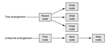
Figure A-47 Tree and Linked List Arrangements of Structures
