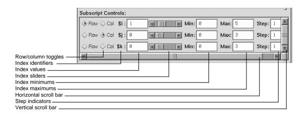
Figure 4-14 Subscript Controls Panel in Array Browser Window
