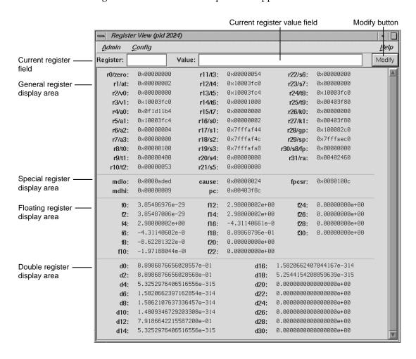
Figure A-58 The Register View Window
