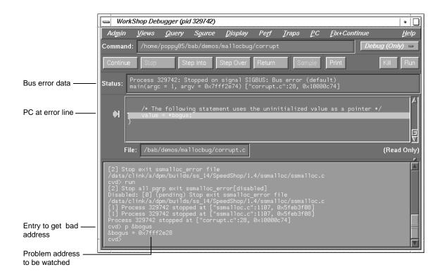
Figure 9-3 Main View at Bus Error
