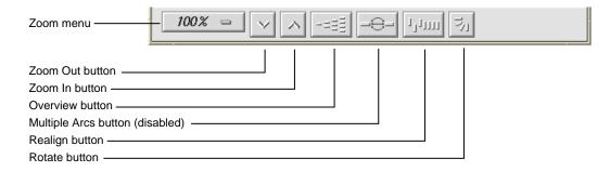
Figure A-6 Build Graph Control Area
