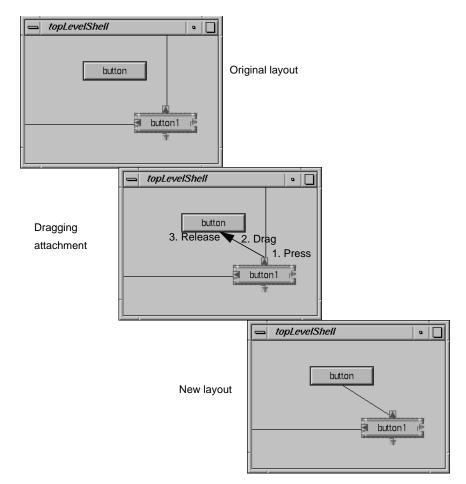
Figure 3-20 Drawing an Attachment
