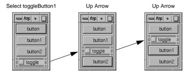
Figure 1-7 Repositioning a Widget in a RowColumn
