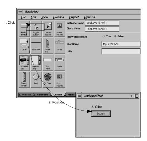
Figure 1-4 Creating a Pushbutton as a Child of a Bulletin Board
