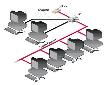
Figure 1-1 Ethernet Network Attachment
