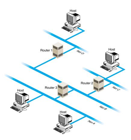
Figure 3-1 Network With Multicast Routers
