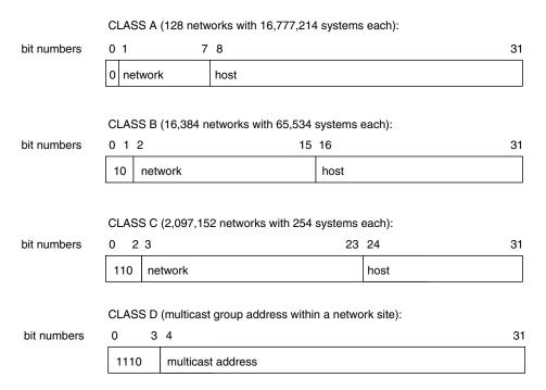
Figure 2-2 Format of Internet Protocol (IP) Addresses
