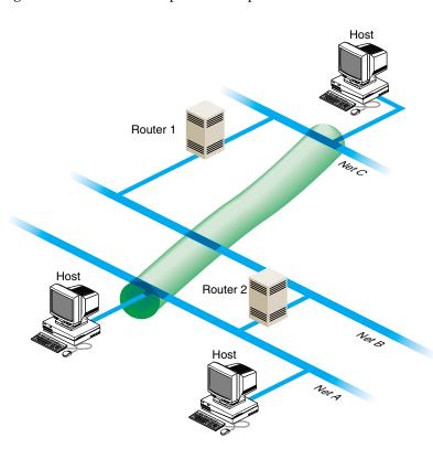
Figure 3-2 A Tunnel Between Networks A and C
