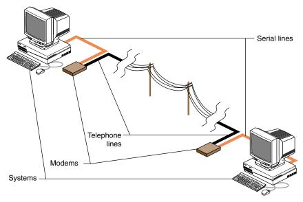
Figure 1-2 Serial Line Network
