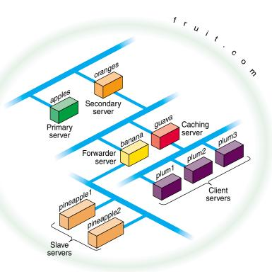
Figure 6-2 Example BIND Configuration
