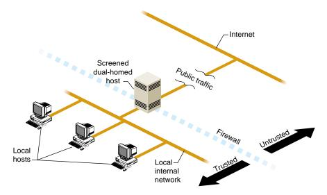
Figure 5-1 A Simple Firewall Environment
