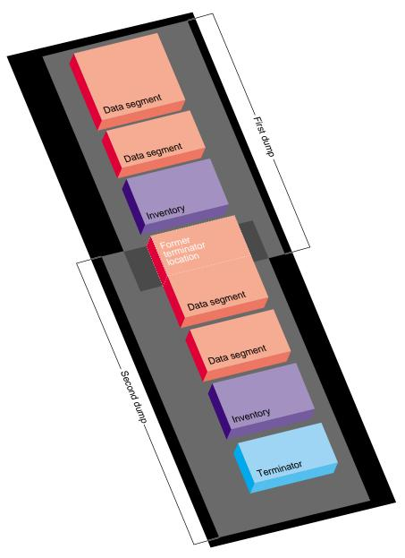
Figure 2-3 Multiple Dumps on Single Media Object
