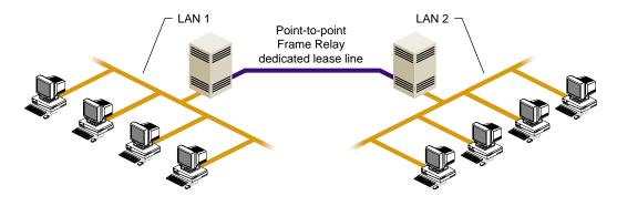
Figure 1-2 Point-to-Point LAN Connection Using Frame Relay
