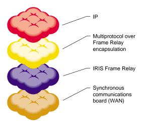
Figure 1-1 Frame Relay in the Communications Hierarchy
