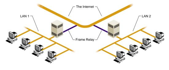
Figure 1-3 Internet Connection Using Frame Relay
