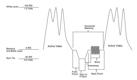
Figure Gl-11 shows a composite video signal without setup.
