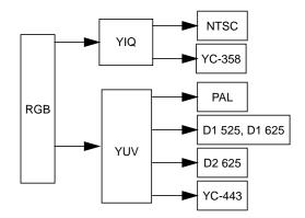
Figure A-2 Relationships Between Color-encoding Methods and Video Formats
