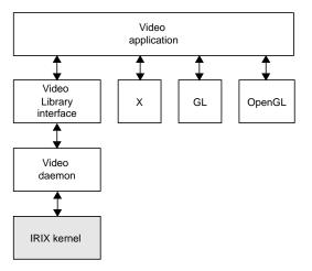
Figure 1-1 diagrams the interaction between the VL, the video daemon, the kernel, the hardware, and the X Window System server.
