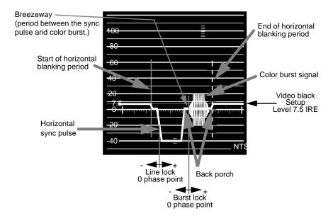
Figure GI-5 Horizontal Blanking Interval
