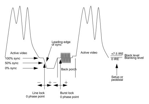
Figure A-3 Composite Video Waveform
