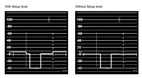
Figure GI-6 Waveform Monitor Readings with and without Setup
