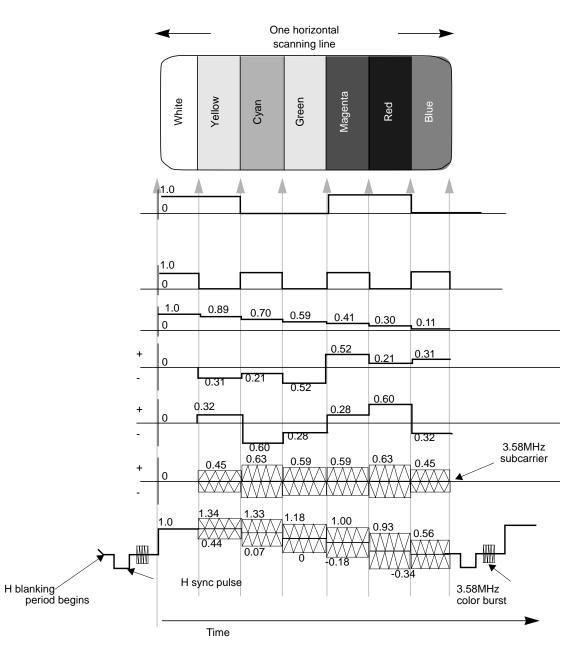
Figure GI-3 Component Video Signals
