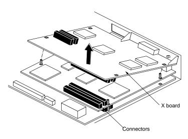
Figure 2-6 Disconnecting the X Board From the Z Board
