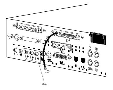
Figure 3-16 Attaching the Label Over the Audio Ports
