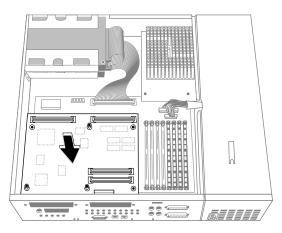
Figure 2-14 Positioning the Graphics Board Over the System Board
