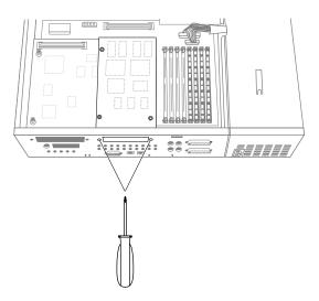
Figure 1-7 Removing the Screws From the GIO Board Connector
