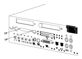
Figure 2-20 Securing the Z Board to the Rear of the Workstation
