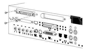
2. On the rear of the workstation, remove the two screws that secure the X board to the chassis as shown in Figure 2-5.
