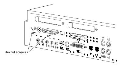
Figure 2-1 Removing the Hexnut Screws From the Rear Panel
