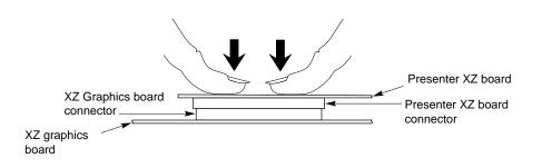
Figure 3-14 Seating the Presenter 1280 XZ Board's Connectors
