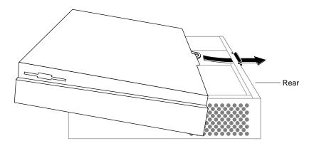
Figure 3-18 Replacing the Top Cover on the Indy Workstation
