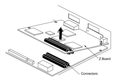
Figure 2-9 Disconnecting the Z Board From the System Board
