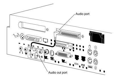
Figure 3-8 Connecting the Audio Cable
