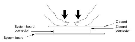
Figure 2-19 Seating the Z Board's Connectors
