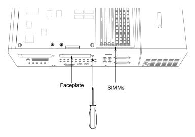
Figure 3-9 Removing the Faceplate From the GIO Option Port
