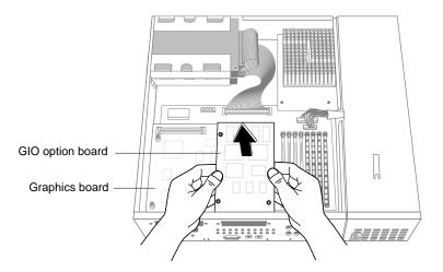
Figure 1-9 Disconnecting the GIO Option Board
