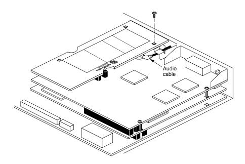
Figure 3-15 Inserting the Screw on the Presenter 1280 XZ Board
