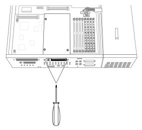
Figure 4-2 Removing the External Screws
