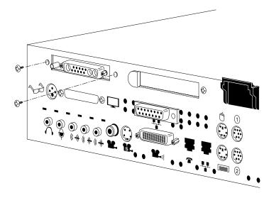
Figure 2-24 Securing the X Board to the Rear of the Workstation
