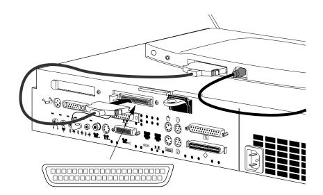
Figure 3-19 Connecting the Presenter 1280 Interface Cable: Indy Graphics
