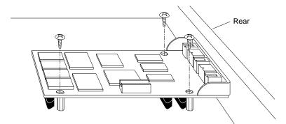
Figure 1-8 Removing the Screws From the GIO option Board
