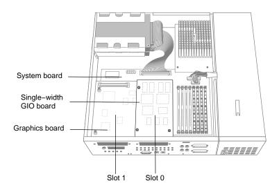
Figure 1-6 Indy Workstation With Single-Width GIO Option Board
