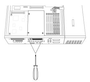
Figure 3-5 Inserting the Screws on the Rear Panel
