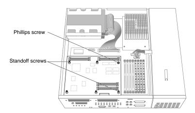
Figure 2-17 Inserting the Screws on the Graphics Board
