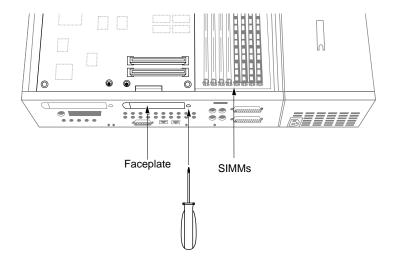
Figure 3-1 Removing the Faceplate From the GIO Option Port
