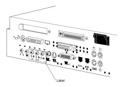
Figure 3-7 Attaching the Label Over the Audio Ports
