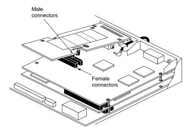
Figure 4-7 Removing the Presenter 1280 XZ 1280 Board
