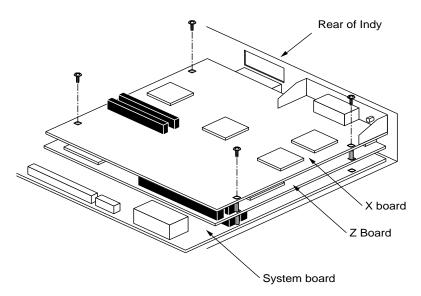
Figure 2-25 Inserting the Screws on the X Board
