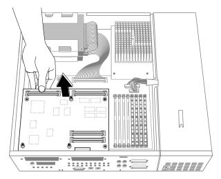
Figure 2-3 Disconnecting the Graphics Board From the System Board
