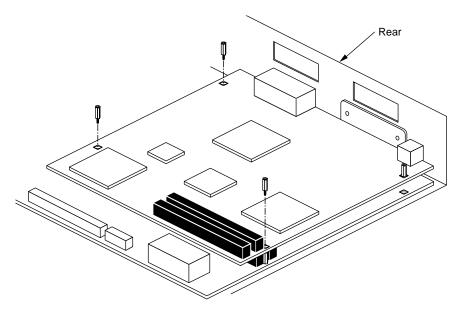
Figure 2-21 Inserting the Standoff Screws on the Z Board
