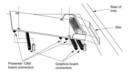
Figure 3-3 Positioning the Presenter 1280 Board Over the Graphics Board
