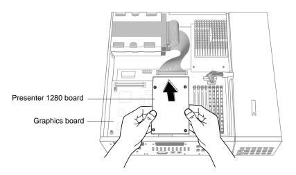
Figure 4-4Removing the Presenter 1280 Board
