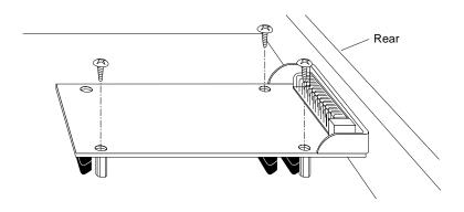
Figure 4-3 Removing the Screws from the Presenter 1280 Board
