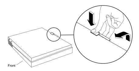
Figure 1-5 Removing the Top Cover From the Indy Workstation
