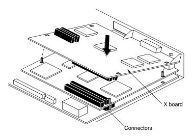
Figure 2-22 Positioning the X Board Over the Z Board
