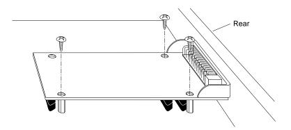
Figure 3-6 Securing the Presenter 1280 Board
