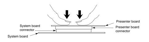
Figure 3-4 Seating the Presenter 1280 Board's Connectors
