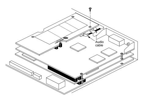
Figure 4-6 Removing the Screw From the Presenter 1280 XZ Board
