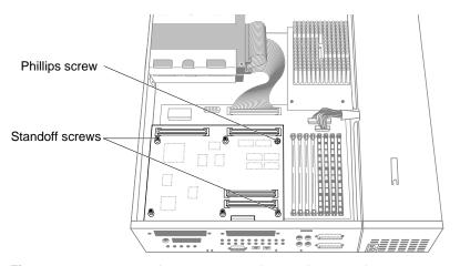
Figure 2-2 Removing the Screws From the Graphics Board
