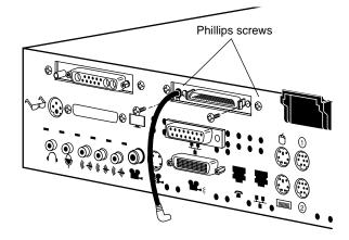
Figure 3-11 Inserting the Screws on the Exterior of the Bracket
