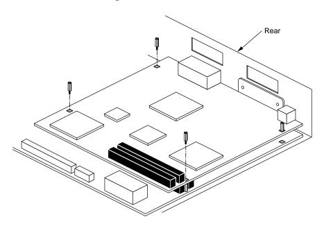
Figure 2-7 Removing the Standoff Screws From the Z Board
