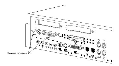
Figure 2-16 Replacing the Screws on the Backplane
