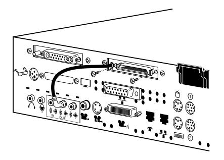
Figure 3-17 Attaching the External Screws
