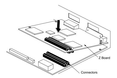
Figure 2-18 Positioning the Z Board Over the System Board
