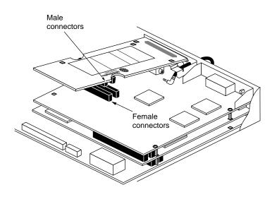
Figure 3-13 Positioning the Presenter 1280 XZ Board
