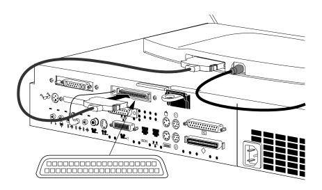
Figure 3-20 Connecting the Presenter 1280 Interface Cable: Indy XZ Graphics
