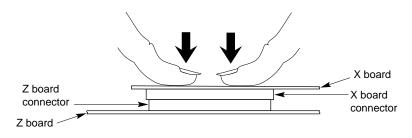
Figure 2-23 Seating the X Board's Connectors
