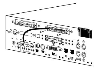
Figure 4-5 Removing the Audio Cable and the External Screws
