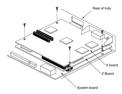
Figure 2-4 Removing the Screws From the X Board
