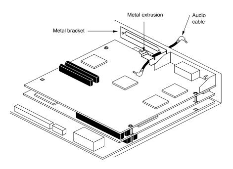
Figure 3-10 Installing the Metal Bracket
