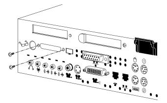
Figure 2-8 Removing the Exterior Screws For the Z Board
