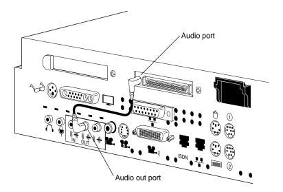
Figure 4-1 Removing the Audio Cable
