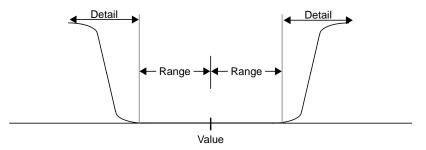
Figure 7-10 shows the relationships between value, range, and detail (transition) for a single channel (for example, A).
