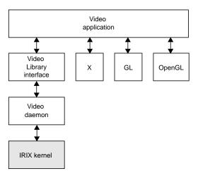
Figure 1-1 VL System Components
