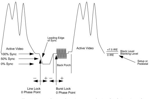
Figure GI-10 Video Waveform: Composite Video Signal With Setup (Typical NTSC)
