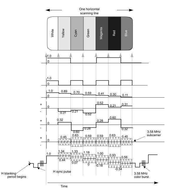
Figure GI-3 Component Video Signals
