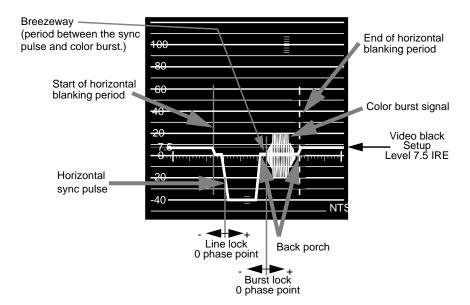
Figure GI-5 Horizontal Blanking Interval
