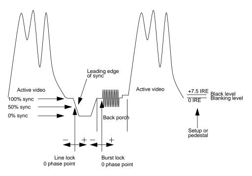
Figure A-3 Composite Video Waveform
