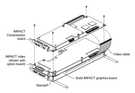
Figure 3-7 Solid IMPACT Graphics with IMPACT Video and Compression Boards
