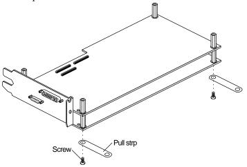
**Figure 3-3** Removing the Pull Straps
