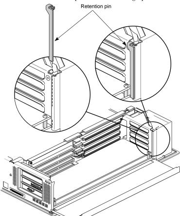
3. Remove the retention pin that secures the graphics board set (Figure 2-8).
