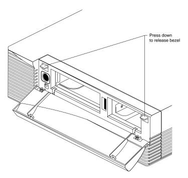
**Figure 2-3** Bezel on the Indigo<sup>2</sup> IMPACT Chassis
