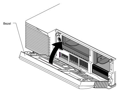
Figure 4-7 Replacing the Bezel
