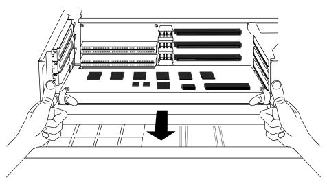
**Figure 2-10** Removing the Graphics Board Set
