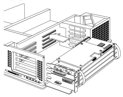
Figure 4-1 Aligning the Board Set with the Chassis
