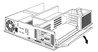
Figure 2-7 Opening the Metal Panel
