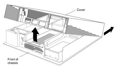
**Figure 2-6** Removing the Cover
