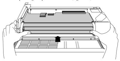
**Figure 4-2** Inserting the Board Set into the Chassis
