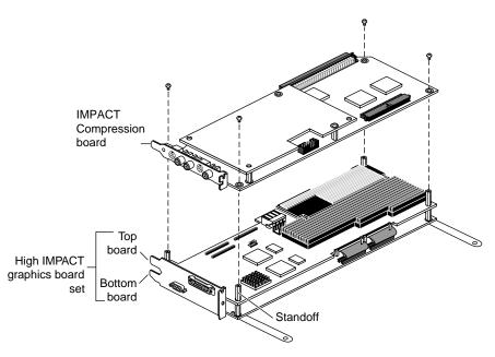
Figure 3-5 High IMPACT Graphics with IMPACT Compression
