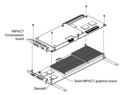
Figure 3-8 Solid IMPACT Graphics with IMPACT Compression
