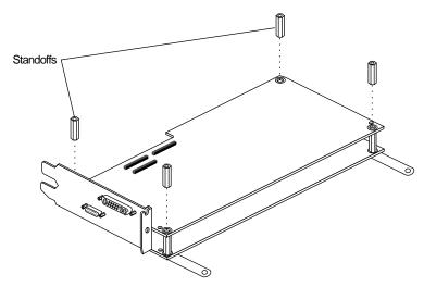
Figure 3-2 Installing the Standoffs
