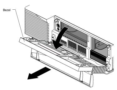
Figure 2-4 Removing the Bezel
