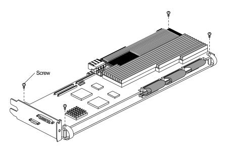
Figure 3-1 Removing Graphics Board Set Screws
