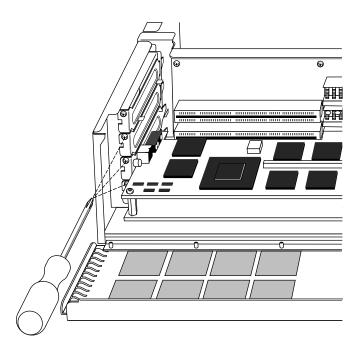
**Figure 2-9** Removing the Slot Cover Screws and Slot Cover
