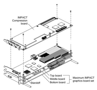
Figure 3-6 Maximum IMPACT Graphics with IMPACT Compression
