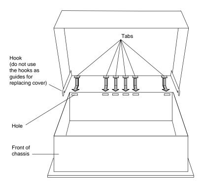
Figure 4-6 Replacing the Cover
