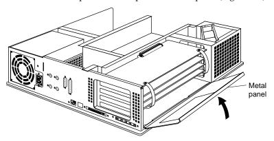
Figure 4-5 Closing the Metal Panel
