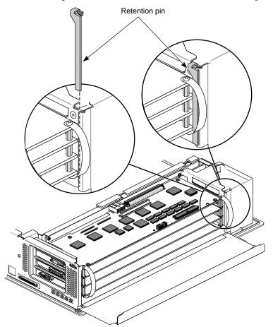
4. Insert the pin that secures the board set to the chassis (Figure 4-4).
