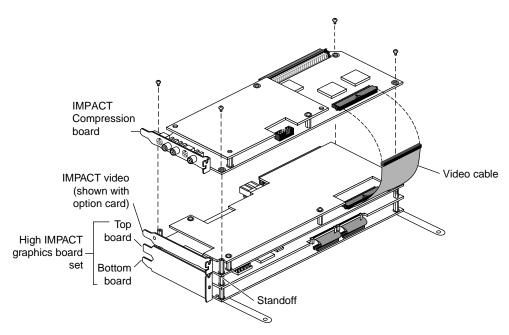
Figure 3-4 High IMPACT with IMPACT Video and IMPACT Compression
