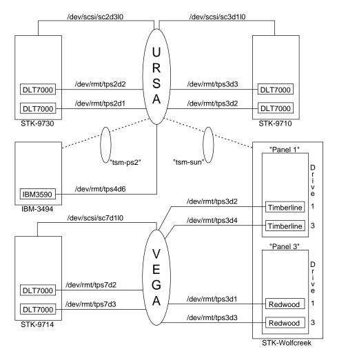
Figure 2-2 Local-and-Remote OpenVault Configuration
