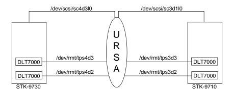
Figure 2-1 Local-Only OpenVault Configuration
