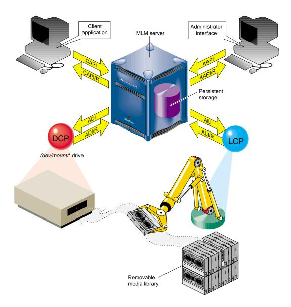
Figure 1-1 OpenVault Architecture
