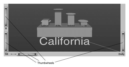
Figure 4-10 Tree Visualizer's Thumbwheels
