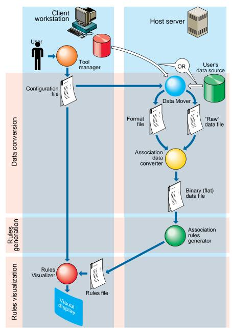
Figure 8-1 Execution Sequence of the Rules Visualizer
