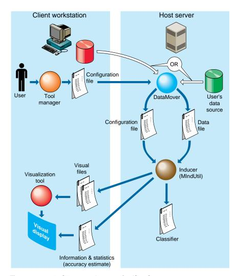
Figure 9-6 Tool Execution Sequence for Classifiers
