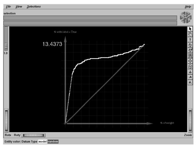
Figure 9-13 Lift Curve for the Churn Dataset
