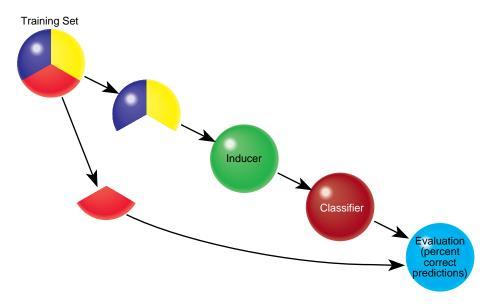
Figure 9-10 Estimating the Classifier's Accuracy
