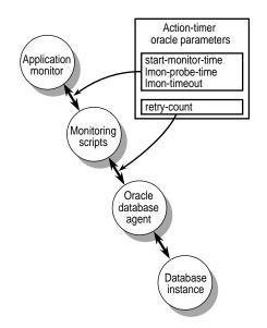
Figure 3-2 Monitoring Configuration Parameters in the Action-Timer Oracle Block
