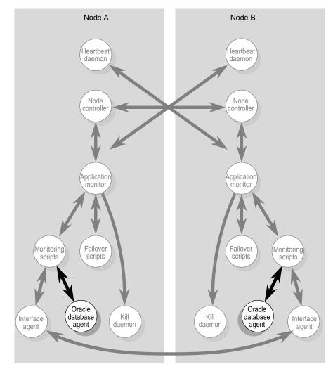
Figure 1-1 Oracle Database Agent Component in IRIS FailSafe
