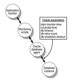
Figure 3-1 Monitoring Frequency Configuration Parameters in Oracle Blocks
