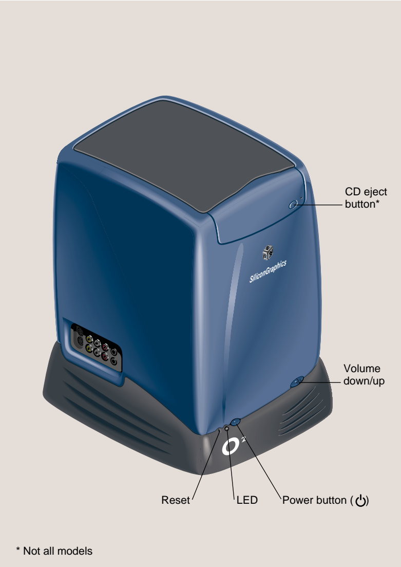
Figure 1-1 Front View of the O2 Workstation
