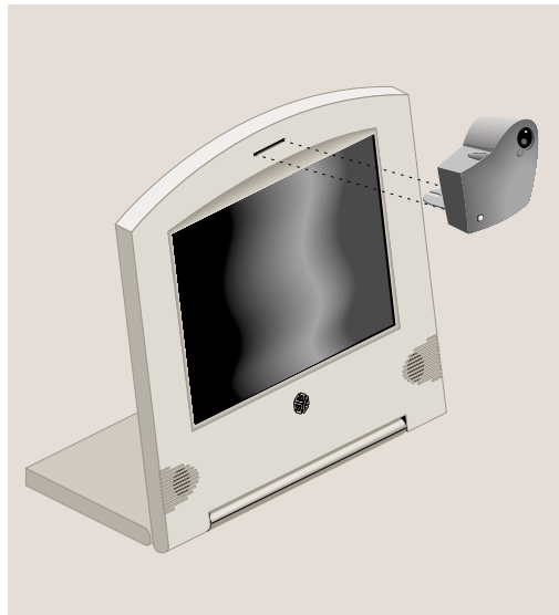
Figure 1-17 Setting Up the Camera on Presenter 1280
