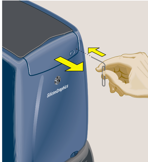
Figure 5-44 Opening the CD-ROM Drive
