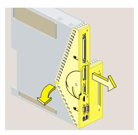
**Figure 2-33** Removing the Face Plate From the System Module
