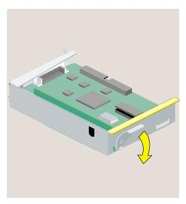
**Figure 2-17** Returning the Lever to its Starting Position
