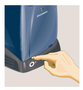
**Figure 3-18** Turning Off the Workstation
