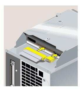
**Figure 5-53** Reconnecting the SCSI and Power Cables
