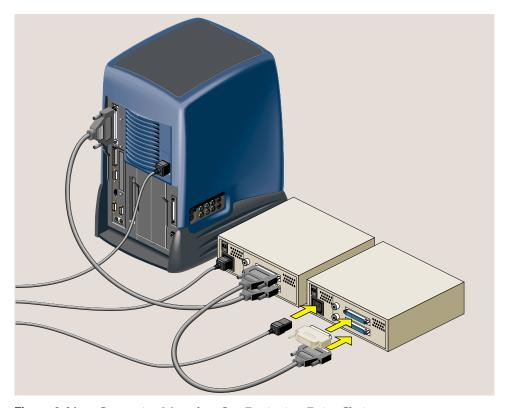
**Figure 3-21** Connecting More than One Device in a Daisy Chain
