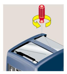
**Figure 5-48** Removing the Three Phillips Screws
