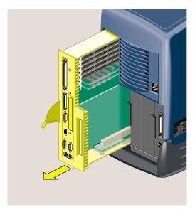
**Figure 2-4** Remove the System Module From the Chassis
