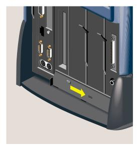
Figure 1-19 Sliding the Lockbar
