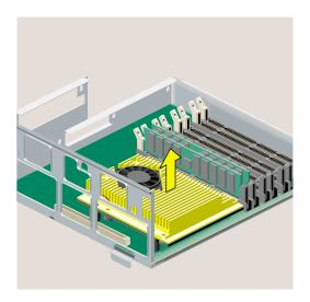
Figure 5-14 Removing the R10000 CPU Module
