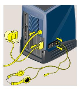
**Figure 5-28** Removing the Cables From the Audio-Visual Module
