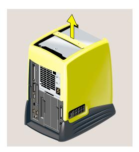
**Figure 5-49** Removing the Outer Cover
