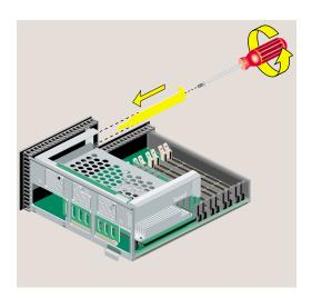
**Figure 2-28** Replacing the Filler Panel and Screw
