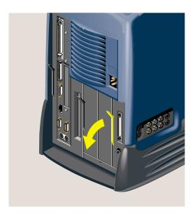
**Figure 5-29** Releasing the Audio-Visual Module
