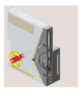
**Figure 5-18** Replacing Two Screws on the Underside
