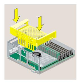
Figure 2-44 Replacing the R10000 PCI Tray in the System Module
