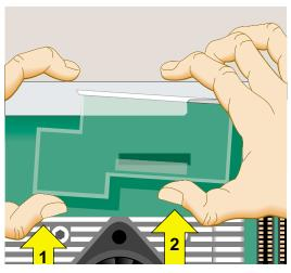
Figure 2-38 Aligning the Option Board
