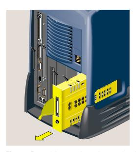
**Figure 3-5** Sliding Out the Audio-Visual Module
