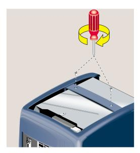
**Figure 5-57** Securing the Outer Cover
