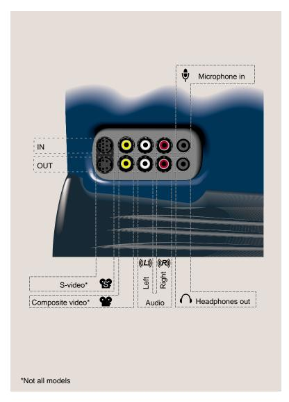
Figure 1-4 Side Panel Audio and Video Ports
