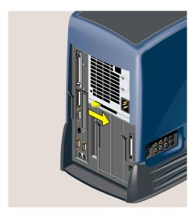
**Figure 5-38** Releasing the Power Supply
