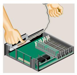
**Figure 5-3** Attaching the Wrist Strap
