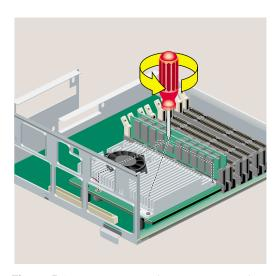
**Figure 5-13** Removing the Screws From the R10000 CPU Module
