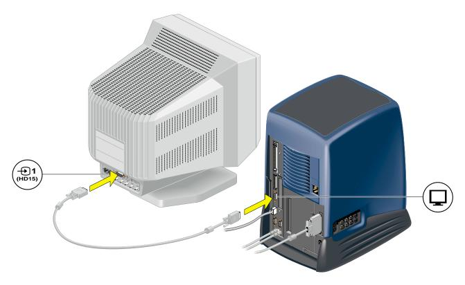
**Figure 1-8** Connecting the Monitor to the Workstation
