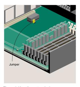
Figure 4-10 Removing the Jumper
