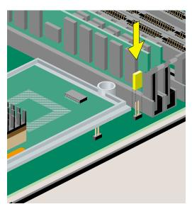
Figure 4-11 Installing the Jumper
