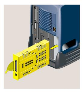
**Figure 3-9** Reinstalling the Audio-Visual Module in the Chassis
