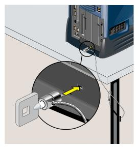
Figure 1-20 Locking the O2 Workstation
