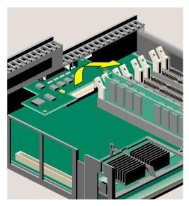
Figure 2-49 Removing the Display Adapter Board
