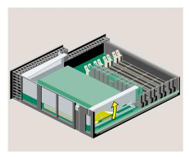
Figure 2-20 Releasing the PCI Tray
