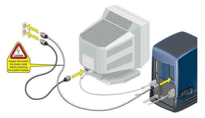
**Figure 1-9** Connecting the Power Cables to the Monitor and to the Workstation
