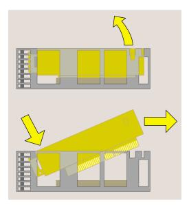
**Figure 2-14** Removing the PCI Tray
