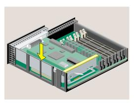
Figure 5-8 PCI Tray Seated Correctly
