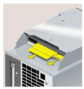
**Figure 5-52** Disconnecting the SCSI and Power Cables
