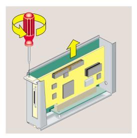
**Figure 2-22** Removing the Screw and the PCI Board
