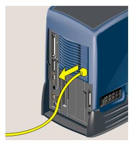
**Figure 2-2** Disconnecting the Power Cables
