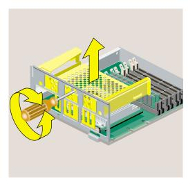
**Figure 5-11** Releasing the PCI tray From the System Module
