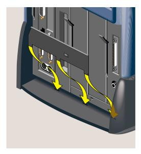
Figure 1-18 Attaching the Lockbar to the Workstation
