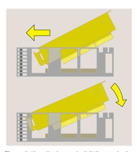
**Figure 2-42** Replacing the PCI Tray in the System Module
