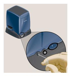
Figure 4-5 Pressing the Reset Button
