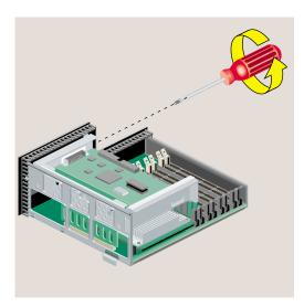
Figure 2-26 Securing the PCI Board
