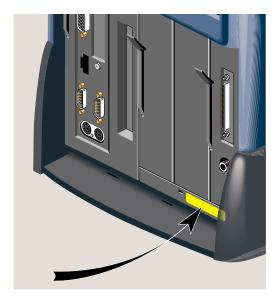
**Figure 1-21** Locating the Serial Number On the Rear
