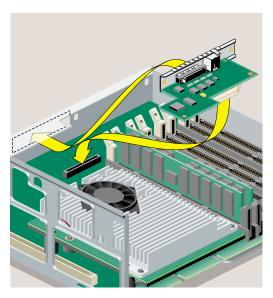
Figure 2-37 Positioning the Option Board
