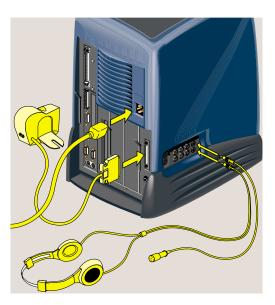
Figure 5-33 Reconnecting the Audio -Visual Cables
