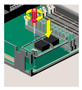
**Figure 5-6** Installing the Replacement CPU Module
