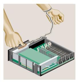
**Figure 2-11** Attaching the Wrist Strap
