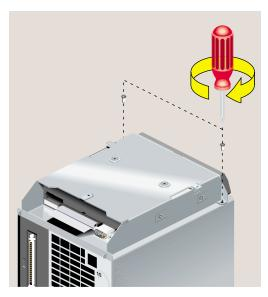
**Figure 5-55** Securing the CD-ROM Drive
