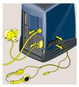
**Figure 3-3** Disconnecting the Power Cable and Other Cables
