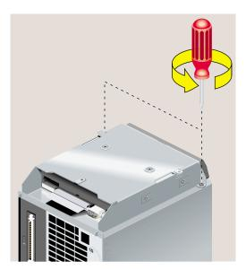
**Figure 5-50** Removing the Screws From the CD-ROM Drive
