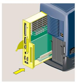
**Figure 2-51** Reinstalling the System Module in the Chassis
