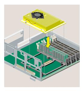
**Figure 5-15** Securing the R10000 CPU Module
