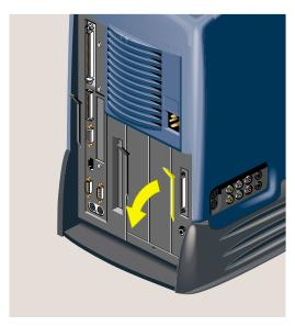
Figure 3-4 Releasing the Audio-Visual Module
