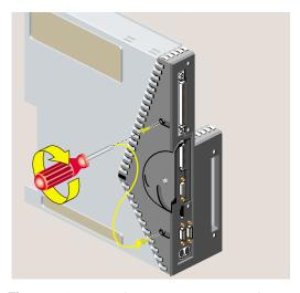
**Figure 2-46** Replacing Two Screws on the Face Plate
