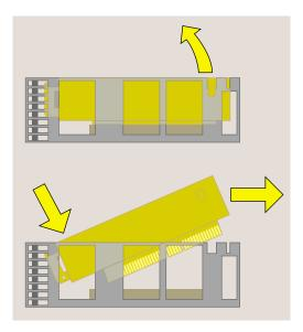
Figure 5-2 Removing the PCI Tray
