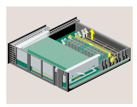
Figure 2-12 Removing the Memory Module
