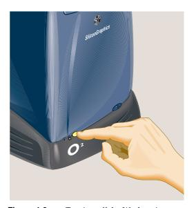
**Figure 4-8** Turning off the Workstation
