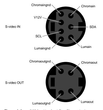
**Figure A-2** S-Video (Analog ) Port Pinout Assignments
