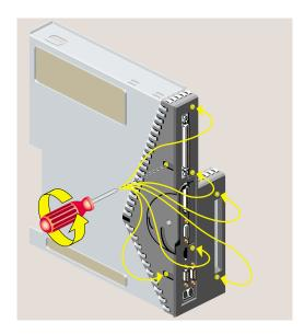
**Figure 5-9** Removing Seven Screws From the Face Plate
