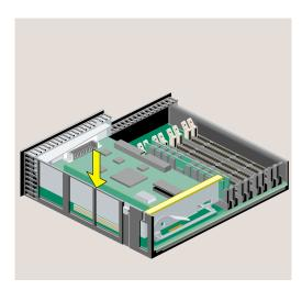
Figure 2-43 PCI Tray Seated Correctly
