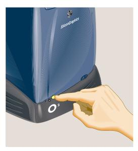
**Figure 5-35** Turning Off the Workstation
