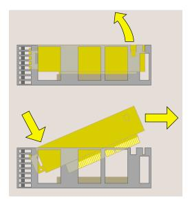
**Figure 2-31** Removing the PCI Tray
