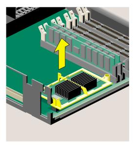
Figure 5-5 Removing the R5000 CPU Module
