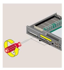
Figure 2-36 Removing the I/O Filler Panel
