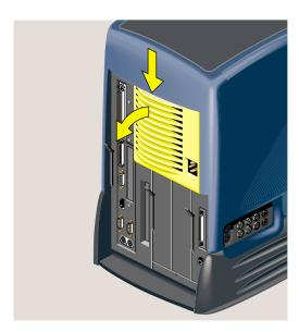
**Figure 5-37** Removing the Bezel From the Power Supply
