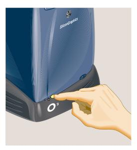
**Figure 5-34** Turning on the Workstation
