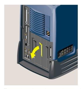
**Figure 3-14** Releasing the Optional Drive Module
