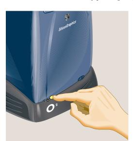
1. Turn off the workstation by pressing the power button on the front (Figure 2-1).
