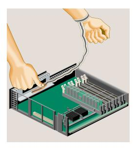
Figure 4-9 Attaching the Wrist Strap
