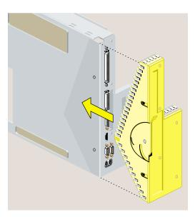
**Figure 5-17** Replacing the Face Plate
