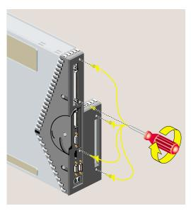
**Figure 5-19** Replacing Five Screws on the Face Plate
