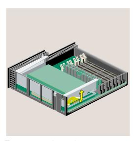
Figure 2-30 Releasing the PCI Tray
