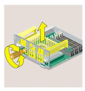
**Figure 2-34** Removing the PCI Tray From the R10000 System Module
