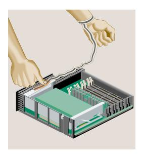
**Figure 2-6** Attaching the Wrist Strap
