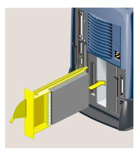
**Figure 5-24** Installing the Replacement System Drive Module
