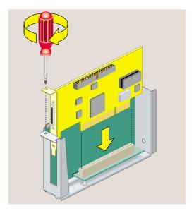
Figure 2-16 Installing the PCI Board
