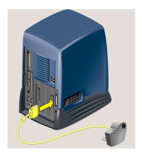
**Figure 1-13** Connecting the O2Cam to the Workstation
