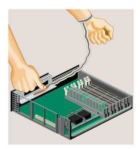
**Figure 2-35** Attaching the Wrist Strap
