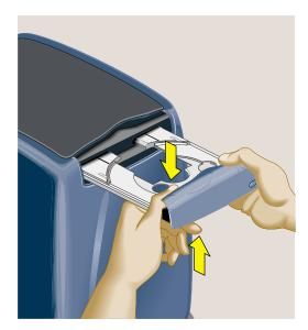
**Figure 5-45** Removing the CD-ROM Drive Face Plate
