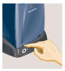
Figure 3-13 Turning Off the Workstation
