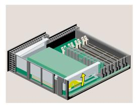
Figure 2-13 Releasing the PCI Tray
