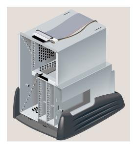
**Figure 5-62** The Stripped Down Workstation Chassis
