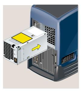
**Figure 5-40** Installing the Replacement Power Supply
