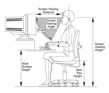
**Figure 6-1** Basic Parameters of Visual Display Terminal Workstation Adjustment (Adapted From ANSI/HFS 100-1988)
