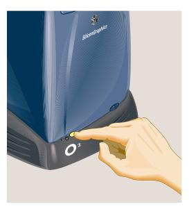
Figure 3-1 Turning Off the Workstation
