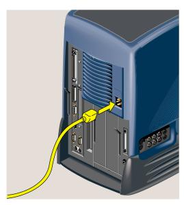
**Figure 5-43** Reconnecting the Power Cable
