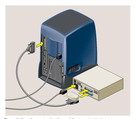
**Figure 3-19** Connecting One External Device to the Workstation
