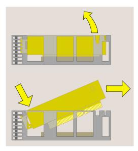
Figure 2-21 Removing the PCI Tray
