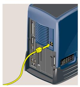
**Figure 5-61** Reconnecting the Power Cable
