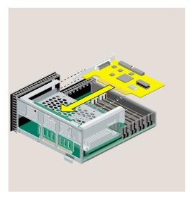
Figure 2-25 Installing the PCI Board on the R10000 Workstation
