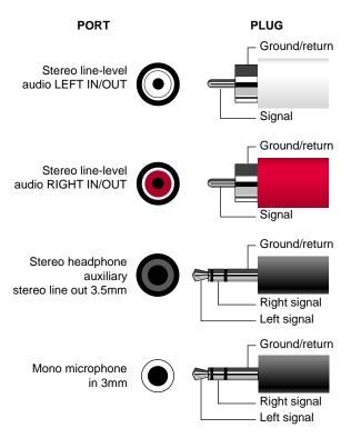
Figure A-1 Audio Ports Pinout Assignments
