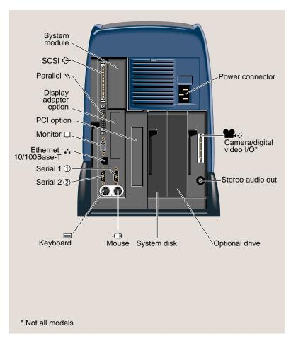
Figure 1-2 Rear View of the O2 R5000 Workstation
