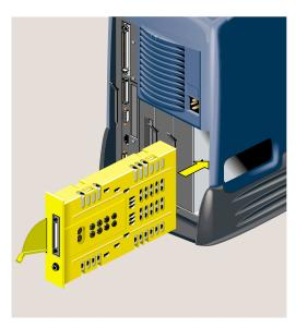
Figure 5-31 Installing the Replacement Audio-Visual Module
