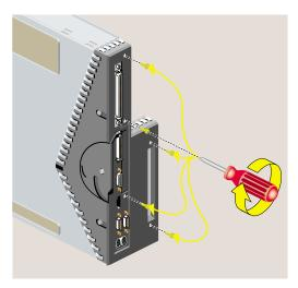
**Figure 2-47** Replacing Five Screws on the Face Plate
