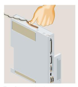
Figure 5-12 Attaching the Wrist Strap
