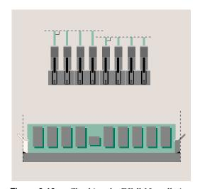
**Figure 2-10** Checking the DIMM Installation
