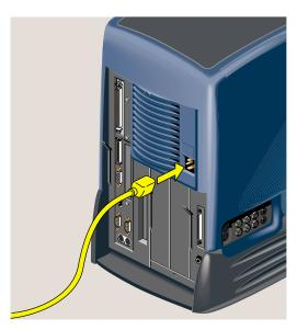
**Figure 5-26** Reconnecting the Power Cable
