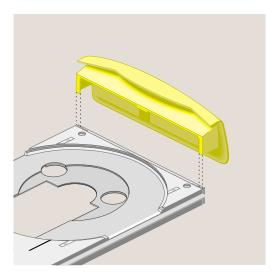
**Figure 5-60** Replacing the CD-ROM Face Plate
