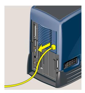
**Figure 5-36** Removing the Power Cable
