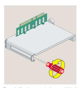
Figure 2-15 Removing the Screw and Filler Panel
