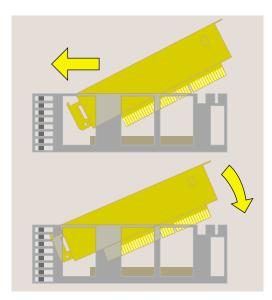
**Figure 2-18** Replacing the PCI Tray in the System Module
