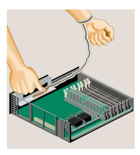
Figure 2-48 Attaching the Wrist Strap
