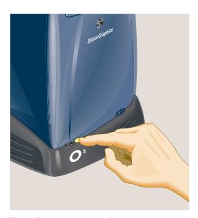
**Figure 5-27** Turning Off the Workstation
