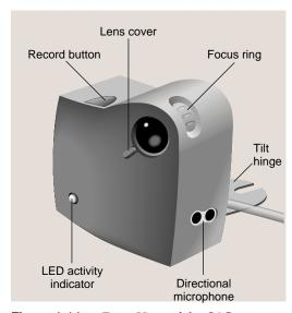
Figure 1-14 Front View of the O2Cam
