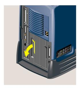
**Figure 5-22** Releasing the Drive Tray
