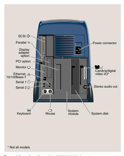
Figure 1-3 Rear View of the O2 R10000 Workstation
