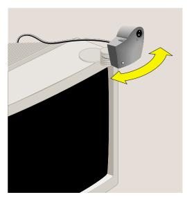
**Figure 1-16** Setting Up the O2Cam on Your Monitor
