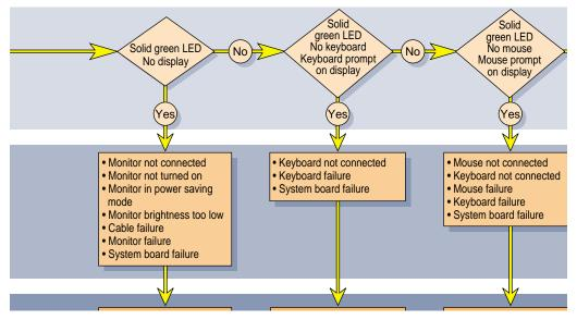
Figure 4-2 Diagnostic Flow Chart #2 (Expand the Window to View)
