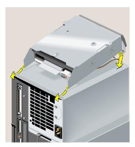
Figure 5-54 Installing the Replacement CD-ROM Drive
