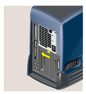
**Figure 5-41** Locking the Power Supply in Place
