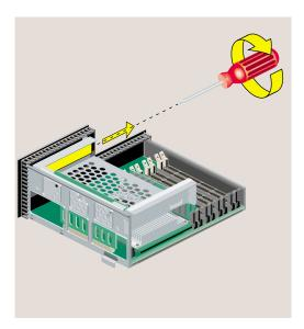
**Figure 2-24** Removing the Screw and Filler Panel
