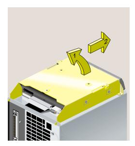
**Figure 5-51** Removing the CD-ROM Drive
