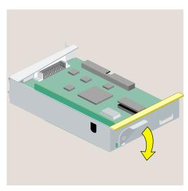
**Figure 2-41** Returning the Lever to its Starting Position
