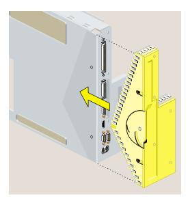
Figure 2-45 Replacing the Face Plate
