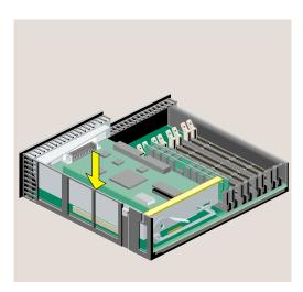
Figure 2-19 PCI Tray Seated Correctly
