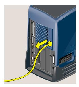
**Figure 5-21** Removing the Power Cables
