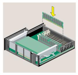
**Figure 2-9** Installing the Memory Modules
