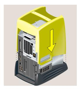
**Figure 5-56** Replacing the Outer Cover
