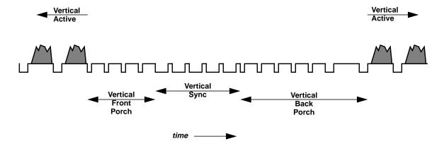
Figure 3-9 Vertical Blanking Region of Commercial Sync Format
