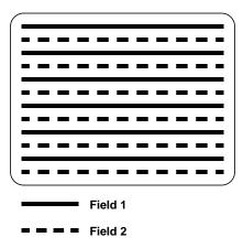
Figure 3-11 Interlaced Format Line Layout
