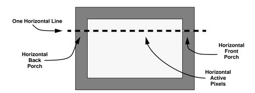
Figure 3-5 Detail of Horizontal Line in Screen Orientation
