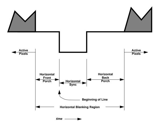
Figure 3-4 Detail of Horizontal Blanking Region
