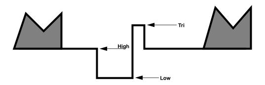
Figure 3-10 Different Levels of Sync
