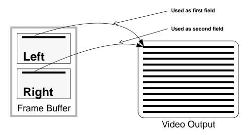
Figure 3-13 Full-Screen Stereo Line Layout
