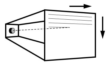
**Figure 3-2** Painting the Screen With a CRT
