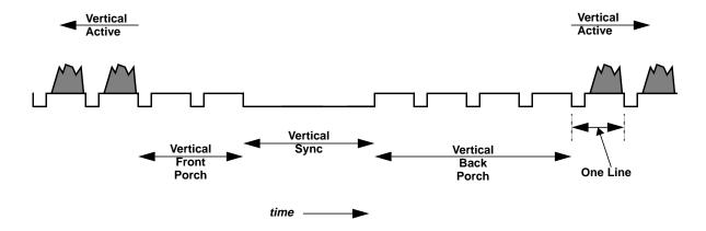
Figure 3-8 A Typical Vertical Blanking Region
