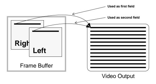
Figure 3-12 Per-Window Stereo Line Layout
