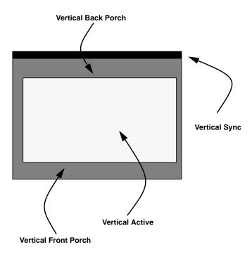
Figure 3-7 Detail of Vertical Regions in Screen Orientation
