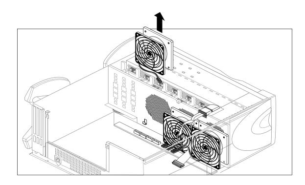
3. Lift the fan out of the system, as shown in Figure 9-4.
