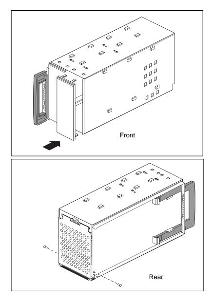
Figure 7-10 Replacing the Front Blanking Plate and Rear Access Plate
