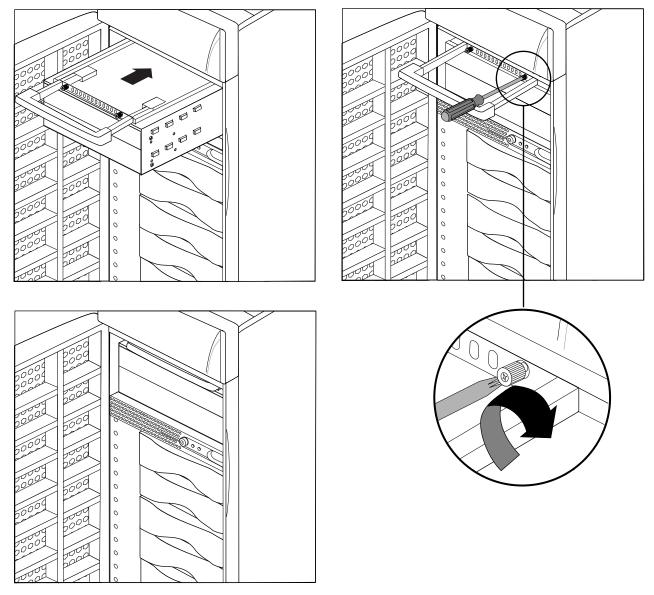
7. Slide the carrier into the system, secure it with the captive screws, and push in the retractable handle. See Figure 2-13.
