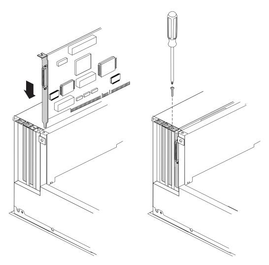
Figure 6-4 Inserting a PCI Option Board
