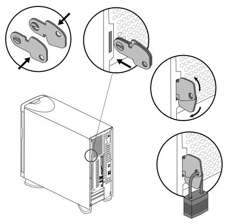
Figure 4-11 Locking the Chassis With the Locking Tabs
