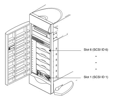
Figure 7-15 How the 3.5-inch Drives are Numbered in Origin200
