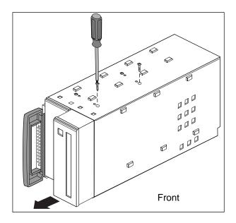
Figure 7-9 Removing A Drive From the Peripheral Carrier
