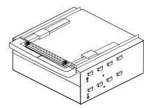
Figure 7-2 5.25-Inch Peripheral Carrier
