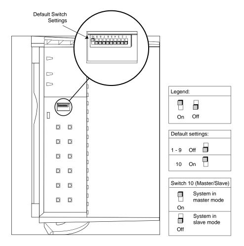
3. Locate the MSC DIP switch, as shown in Figure 2-18.
