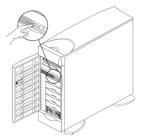
2. At the front of the system, press the power button, as shown in Figure 4-3.
