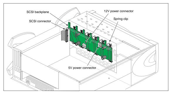
Figure 9-2Cable Connections and Spring Clips On the SCSI Backplane
