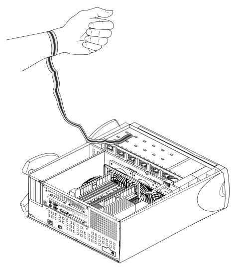
Figure 6-1 Attaching A Grounding Wrist Strap
