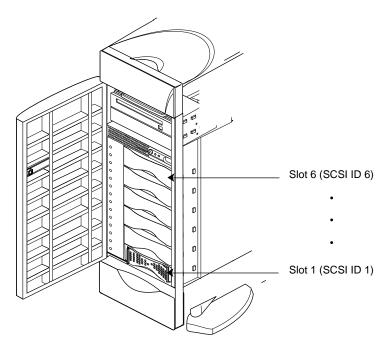
Figure 7-12 The 3.5-Inch Drive Bay and Correspondence of SCSI IDs to Drive Sots
