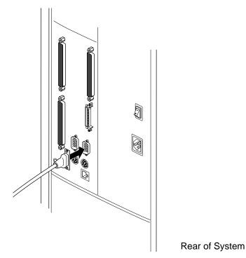
Figure 2-15 Attaching the Serial Cable
