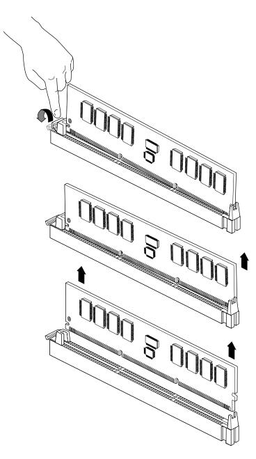
Figure 5-8 Removing DIMMs
