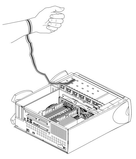
4. Attach a grounding strap to your wrist. Figure 5-5 shows an example of a disposable grounding strap.
