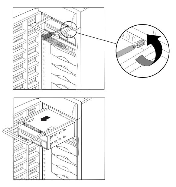
Figure 7-7Removing the Peripheral Carrier
