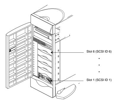
Figure 7-18 How the 3.5-inch Drives are Numbered in Origin200
