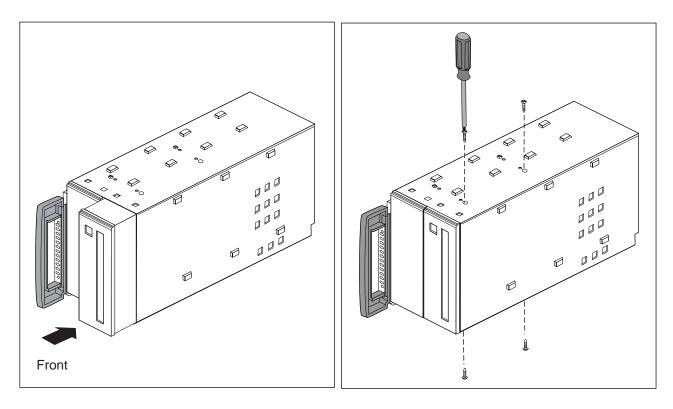
Figure 2-9 Inserting a 5.25-Inch Drive in the Peripheral Carrier
