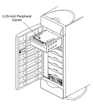
**Figure 1-8** Origin200 5.25-inch Peripheral Carrier and Drive Bay
