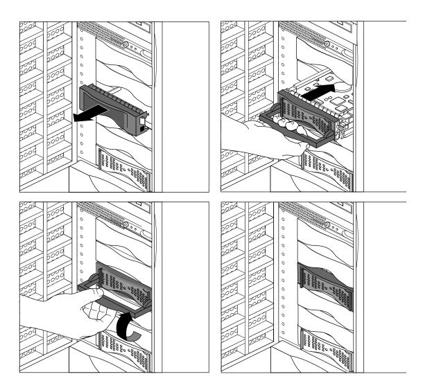
Figure 7-16 Installing a 3.5-inch Peripheral in Origin200
