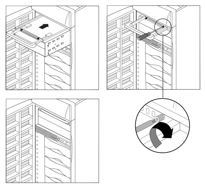
6. Slide the carrier into the system and secure it with the two captive screws. See Figure 7-11.
