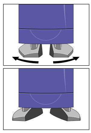
Figure 4-12 Adjusting the Feet
