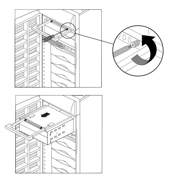
Figure 7-3Removing the 5.25-Inch Peripheral Carrier
