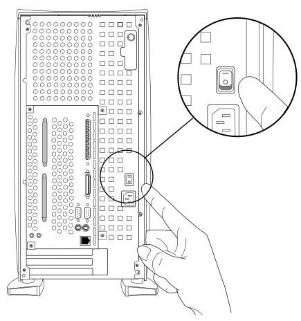
Figure 2-21 Turning On the Master Power Switch
