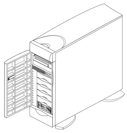
Figure 7-17 Opening the Front Door of Origin200
