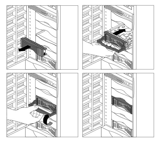
Figure 2-6Installing 3.5-Inch Drives in Origin200
