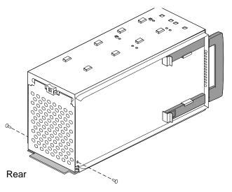
Figure 2-12 Replacing the Rear Access Plate on the Peripheral Carrier
