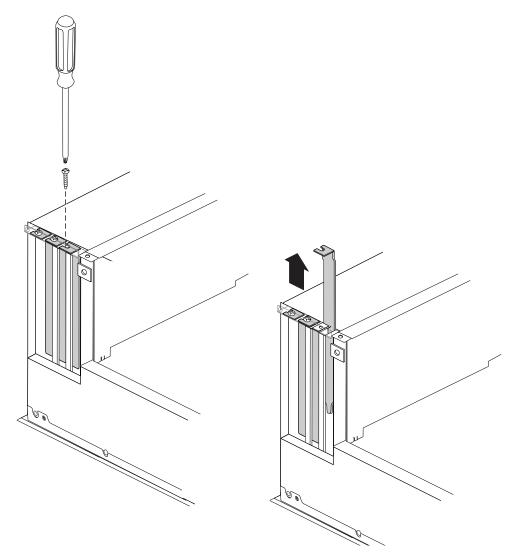
Figure 6-3 Removing a PCI Slot Blanking Plate
