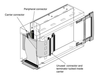
Figure 2-11 Attaching the SCSI Cable to a 5.25-Inch Drive
