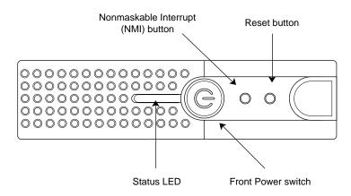
Figure 4-1 The Origin200 Front Panel
