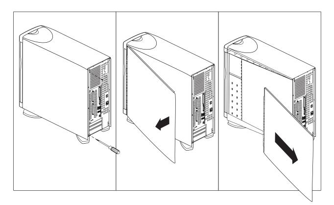
Figure 2-16 Removing the Side Panel of the Second (Slave) Module
