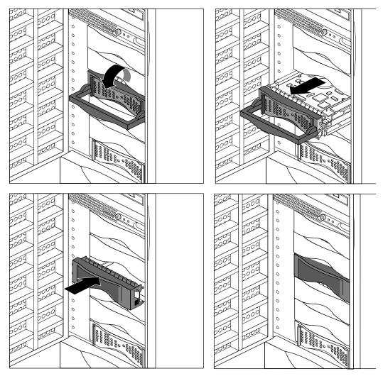
Figure 7-19Removing a 3.5-inch Drive from Origin200
