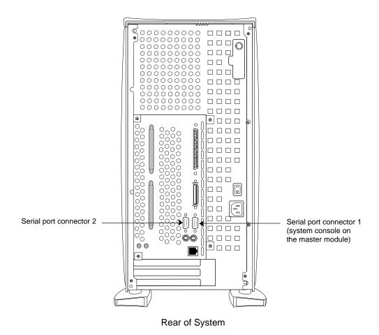
Figure 7-20 Location of the Serial Port Connectors on Origin200
