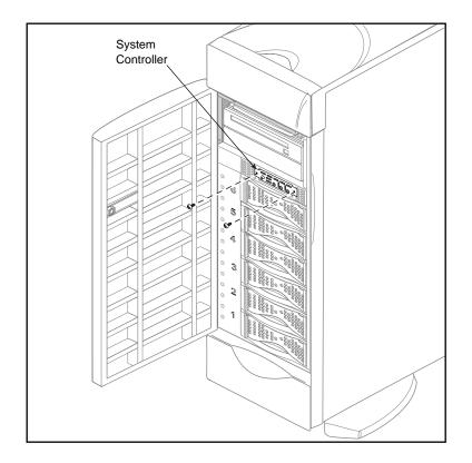
Figure 9-6 Removing the System Controller Assembly From the Chassis
