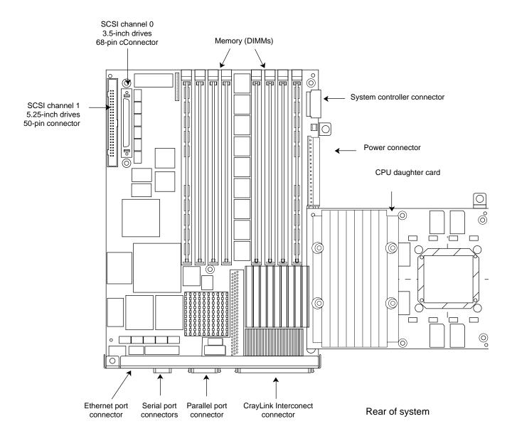
Figure 1-5 The Origin200 Main System Board and CPU Daughter Card
