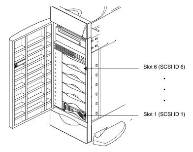
Figure 2-5 SCSI Drive ID Numbering for 3.5-Inch Drives
