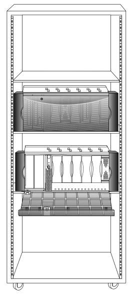
Figure 1-3Two-module Origin200 Server in a Rack
