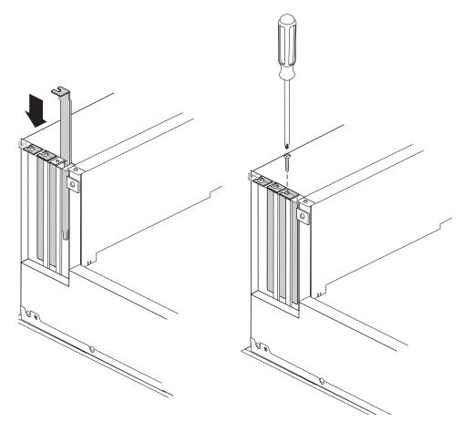
Figure 6-7 Replacing a PCI Option Blanking Plate and Screw
