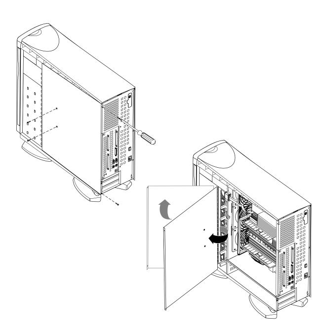
Figure 4-10 Opening the Chassis Access Door, Tower Origin200
