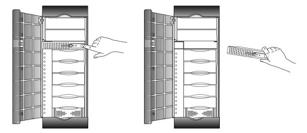
Figure 9-5 Removing the Front Bezel Crossbar
