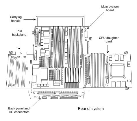
Figure 1-4Logic Carrier Assembly
