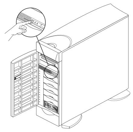
Figure 4-4Turning Off the Front Power Switch
