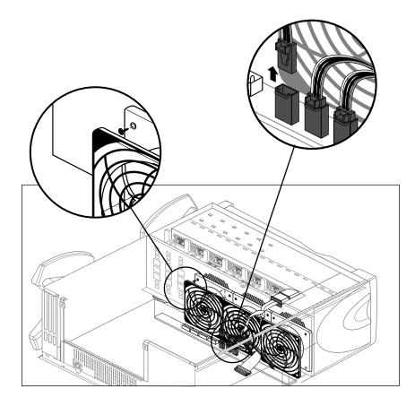
Figure 9-3Disconnecting the Fan and Fan Power Cable (Other Components Removed For<br/>Clarity)
