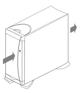
Figure 1-10 Air Flow Through Origin200
