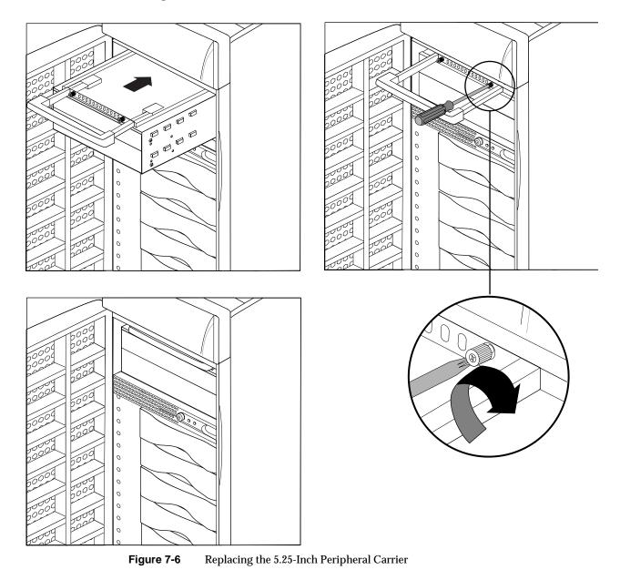
6. Slide the carrier into the system and secure it with the two captive screws. See Figure 7-6.
