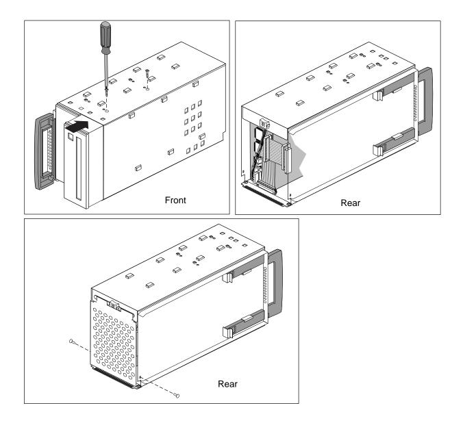
Figure 7-5 Installing a 5.25-Inch Drive in the Peripheral Carrier
