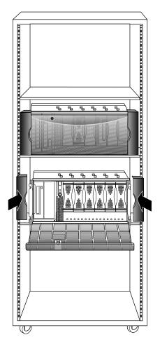
Figure 3-5 Attaching the Plastic End Caps to a Rackmounted Server
