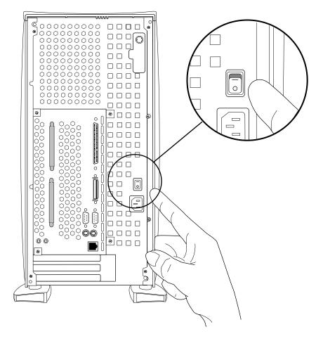
Figure 4-5 Turning Off the Master Power Switch
