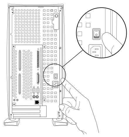
Figure 4-2 Turning On the Master Power Switch
