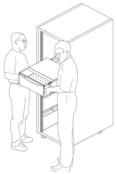
Figure 3-4 Lifting the Origin200 Server Into a Rack
