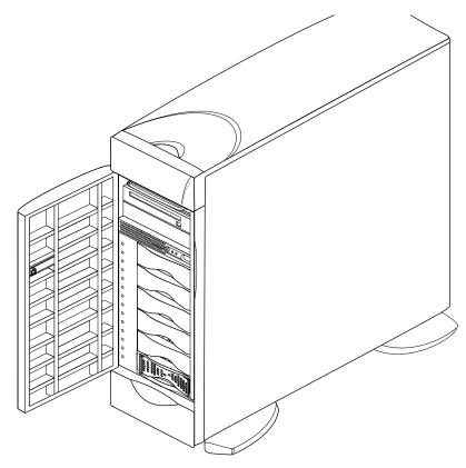
Figure 7-14Opening the Front Door of Origin200
