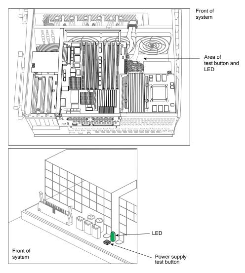
Figure 8-2 Location of the Power Supply Test Button and LED
