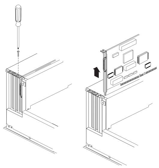
Figure 6-6 Removing a PCI Option Board Screw and Board
