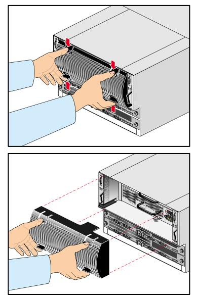
Figure 4-5Removing the Disk Module Fan Assembly
