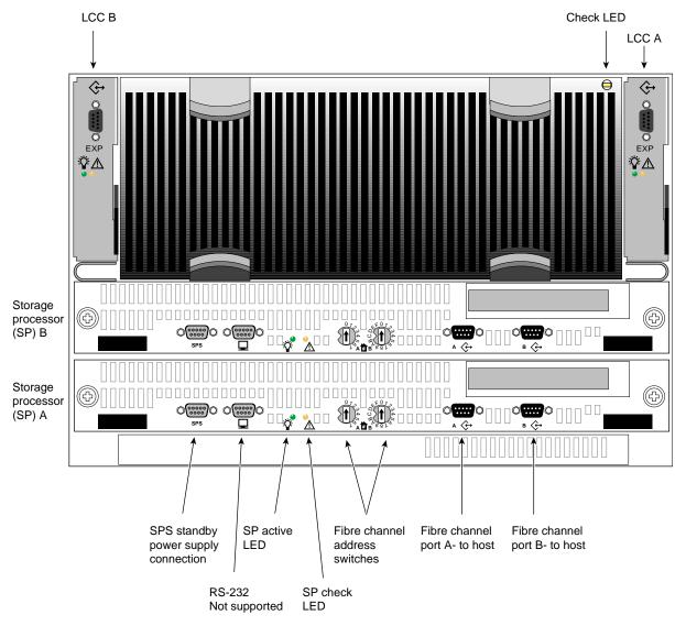
Figure 3-10 Storage Processor Connectors
