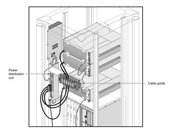
**Figure 1-12** Fibre Vault Enclosures in an Origin Rack (Rear View)
