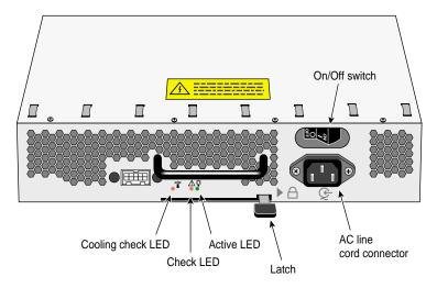
Figure 3-7 Power Supply Features
