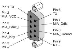
Figure 1-4 XIO Board Connector Pin Assignments
