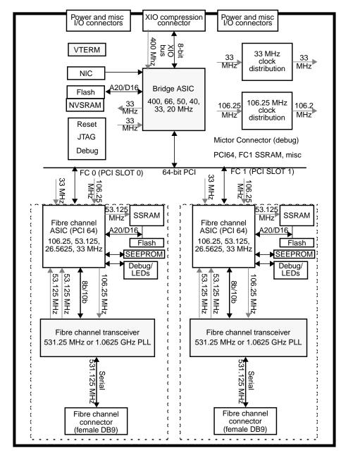
Figure 1-5 Fibre Channel XIO Card Block Diagram
