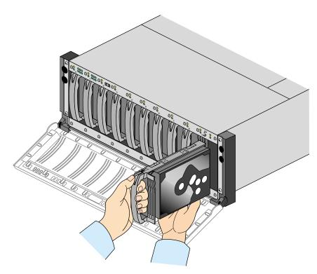
Figure 4-1 The Disk Module
