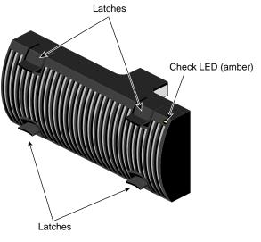
Figure 3-6 Fan Assembly Features
