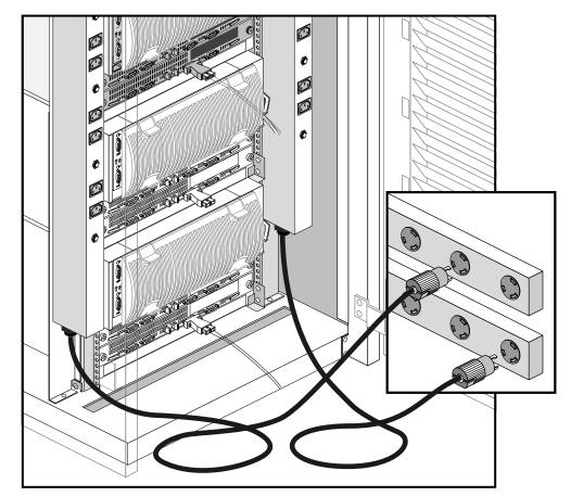
Figure 3-16 Disconnecting Rack Power Cables
