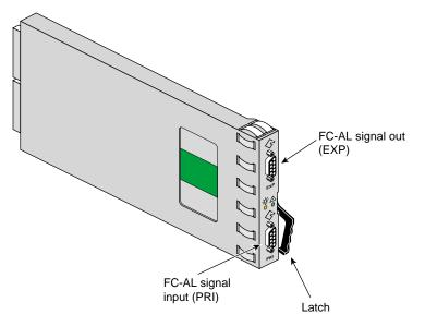
Figure 3-5 FibreVault Link Controller Card (LCC)
