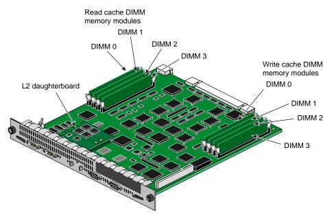
Figure 3-11 Storage Processor Board Components
