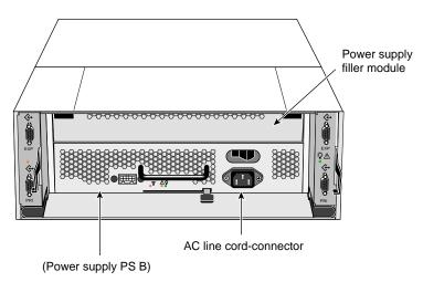
Figure 3-3 shows a rear view of the rackmount FibreVault components (fan module removed).
