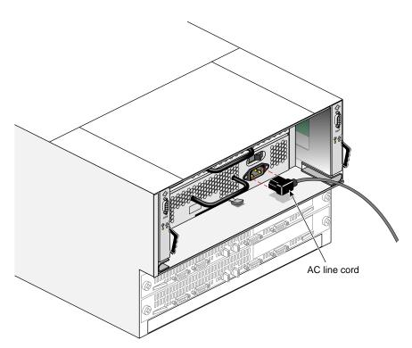
Figure 4-8Power Supply Power Cord
