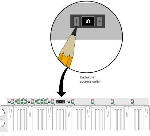
Figure 4-2 Setting the FibreVault ID
