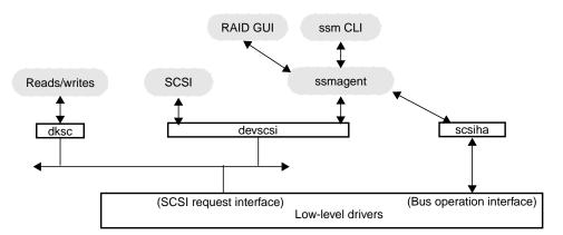
Figure 1-13 Fibre Channel Software Interface
