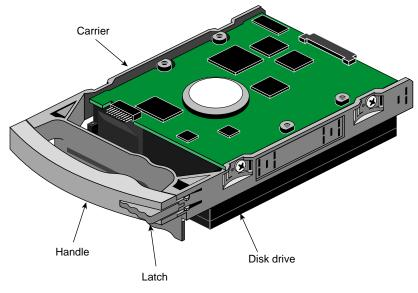
Figure 1-7 shows features of the FC-AL disk module.
