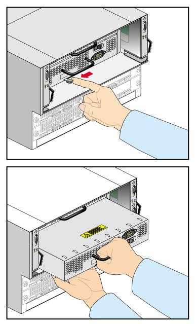
Figure 4-12Removing an Existing Fibre Channel RAID Power Supply or Filler Panel
