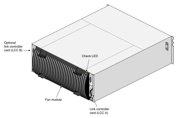
Figure 3-1 FibreVault Back View with Fan Module
