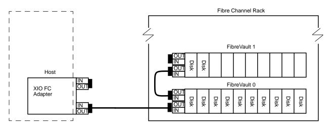
Figure 3-13 diagrams a typical FC storage subsystem.
