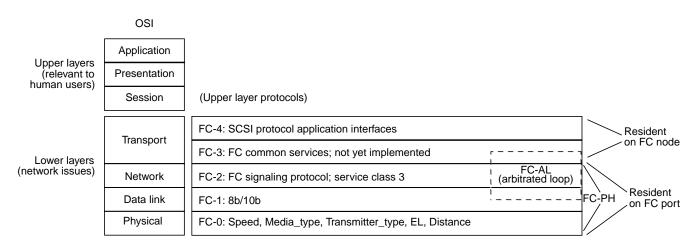
Figure 2-3 Fibre Channel Layers and OSI Layers
