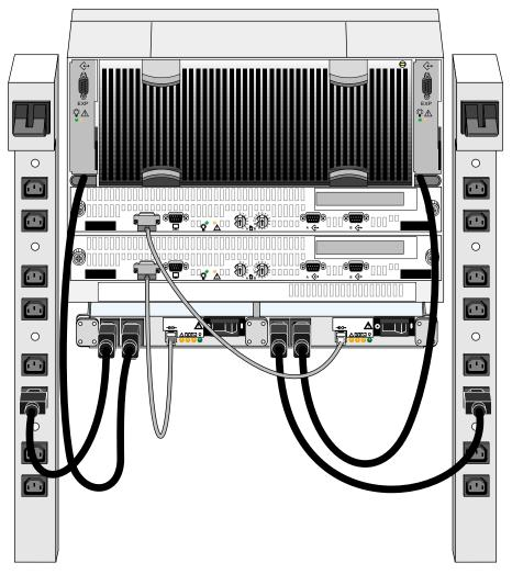
Figure 3-15 Two Rackmounted SPS Examples With Cabling (Rear View)
