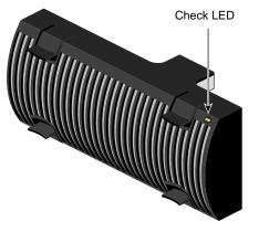
Figure 4-6 Fan Assembly Status LED Orientation
