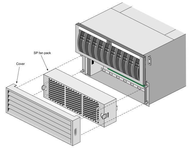
Figure 3-12 illustrates the fibre channel RAID storage processor (SP) fan module.
