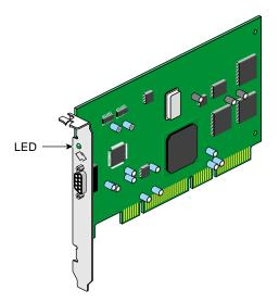
Figure 1-3 Fibre Channel PCI Interface Board
