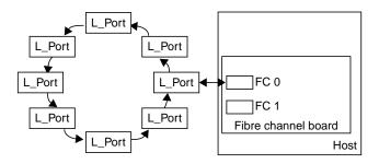
Figure 2-1 Fibre Channel Arbitrated Loop (FC-AL)
