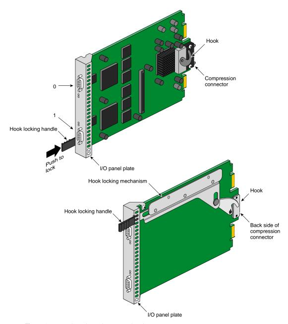
Figure 1-2 Fibre Channel XIO Board and Connectors
