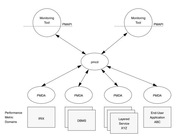
Figure 1-1 PCP Global Process Architecture
