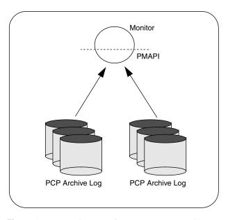
Figure 1-3 Architecture for Retrospective Analysis
