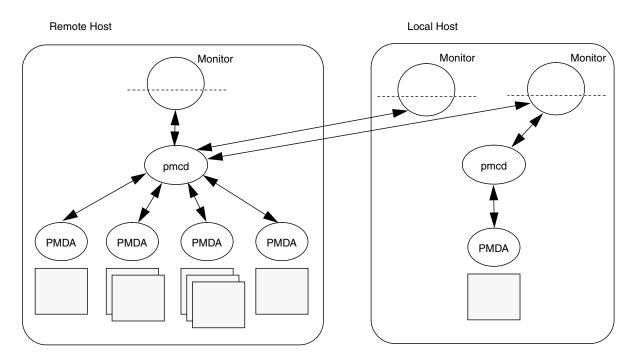
Figure 1-2 Process Structure for Distributed Operation
