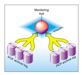
**Figure 1-3** Architecture for Retrospective Analysis
