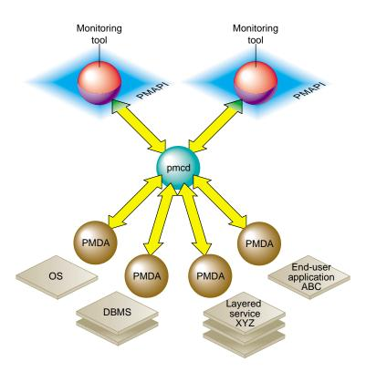
Figure 1-1 PCP Global Process Architecture
