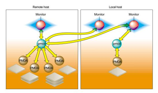
Figure 1-2 Process Structure for Distributed Operation
