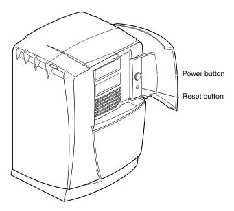
Figure 9-12 Pressing the Reset Button
