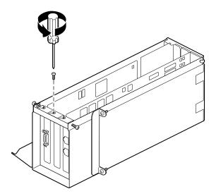
Figure 4-14 Removing the Blank I/O Panel Screw
