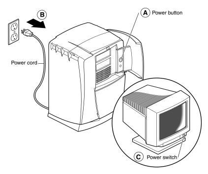
**Figure 3-1** Powering Off the OCTANE Workstation
