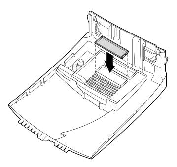
Figure 7-13 Pushing the Blank Panel Free
