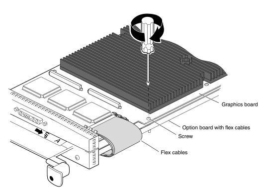
**Figure 5-16** Replacing the Graphics Board Screw
