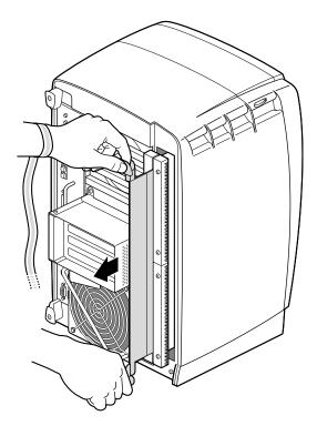
Figure 5-7 Releasing the XIO Module
