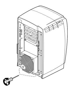
**Figure 3-7** Inserting and Tightening the Screws
