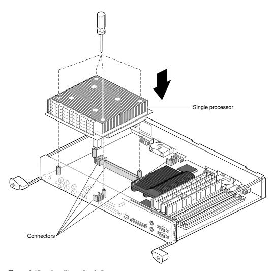
Figure 2-15 Installing a Single Processor
