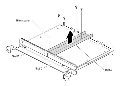
**Figure 5-21** Removing the Baffle
