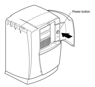
Figure 1-18 Powering On the OCTANE Workstation
