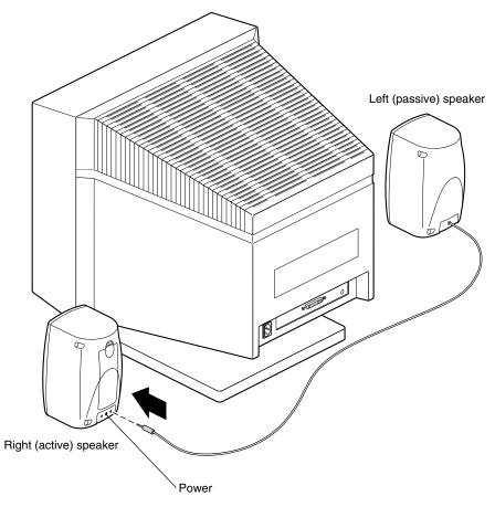
**Figure 1-7** Attaching the Speaker-to-Speaker Cable
