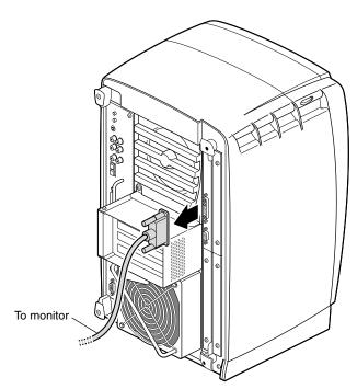
**Figure 5-3** Removing the Monitor Cable
