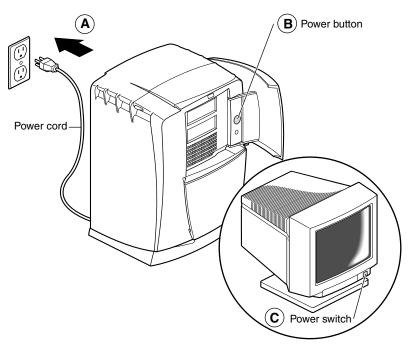
**Figure 3-8** Powering On the OCTANE Workstation
