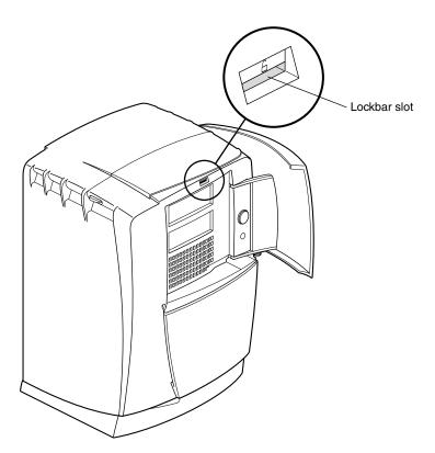
Figure 1-16 Locating the Lockbar Slot
