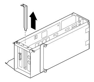
Figure 4-15 Removing the Blank I/O Panel
