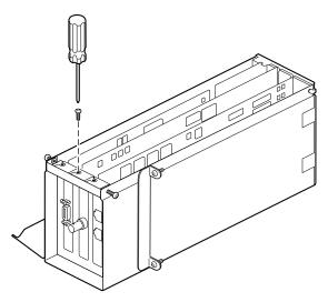
Figure 4-29 Removing the Screw
