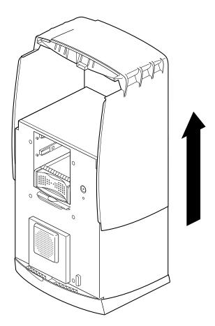
Figure 7-31 Sliding the Front Cover Forward
