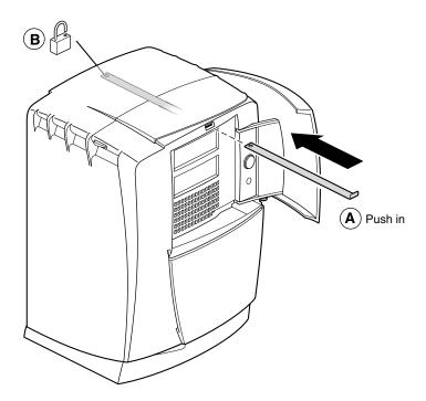
**Figure 1-17** Inserting the Lockbar
