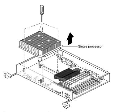
Figure 2-11 Removing the Single Processor
