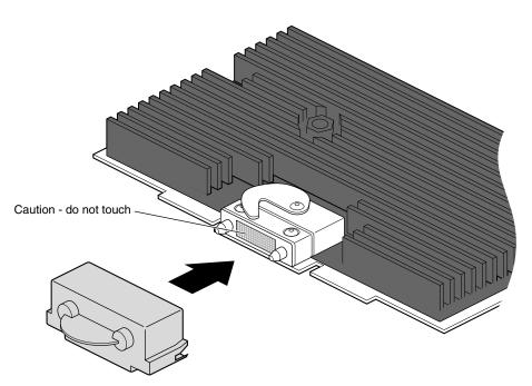
**Figure 5-12** Placing the Cap on the XIO Compression Connector
