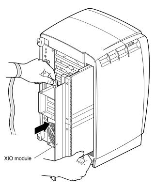
Figure 5-41 Inserting the XIO Module
