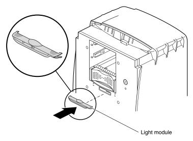
Figure 7-21 Inserting the Light Module
