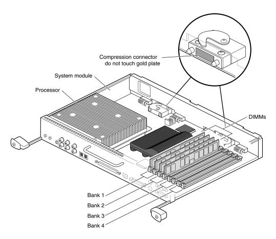
Figure 2-18 Locating DIMMs on the System Module
