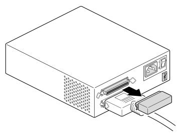
**Figure 6-3** Removing the Terminator From the Last Device on the Daisy Chain
