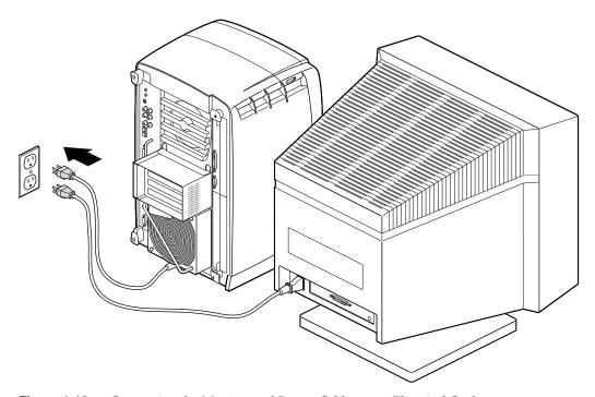
Figure 1-12 Connecting the Monitor and Power Cables to an Electrical Outlet
