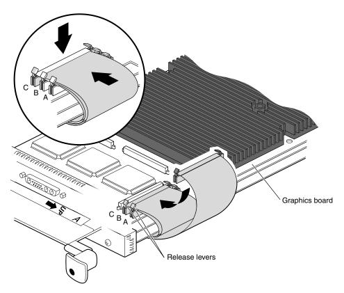
**Figure 5-24** Attaching the Flex Cables to the Graphics Board
