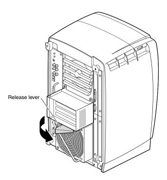
**Figure 4-8** Opening the Release Lever
