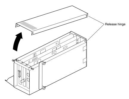
Figure 4-12 Opening and Removing the PCI Module Door
