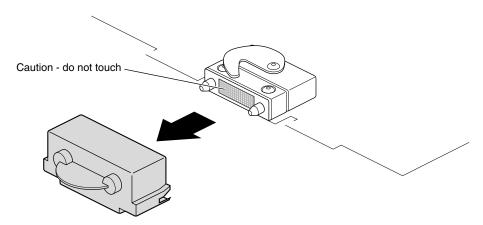
**Figure 2-21** Removing the Compression Connector Cap
