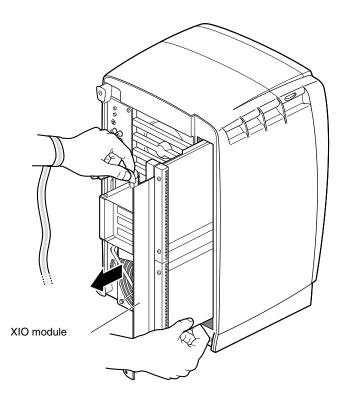
Figure 5-8 Removing the XIO Module
