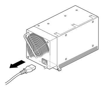
**Figure 3-4** Removing the Power Supply Cable
