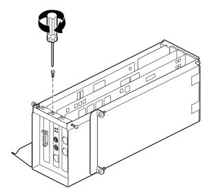
Figure 4-17 Inserting the Board Screw
