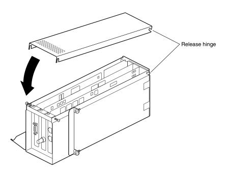
Figure 4-27 Reconnecting the PCI Module Door
