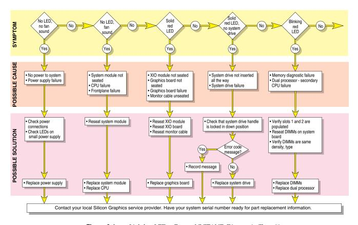
Figure 9-1 Lightbar LEDs - Front of OCTANE, Diagnostic Chart #1
