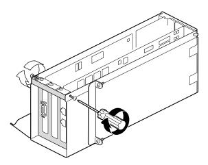
**Figure 4-36** Inserting the I/O Door Screws
