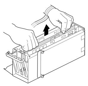
Figure 4-34 Removing a PCI Board
