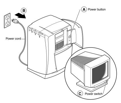
**Figure 7-1** Powering Off the OCTANE Workstation and the Monitor
