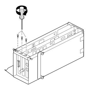
**Figure 4-26** Replacing the I/O Panel Screw
