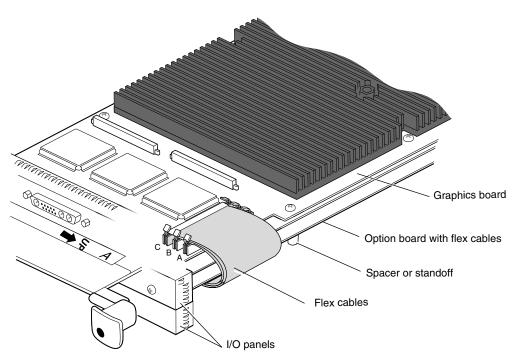
**Figure 5-25** Identifying Parts for the Cable Guard Installation
