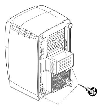
**Figure 2-25** Replacing the System Module Screws
