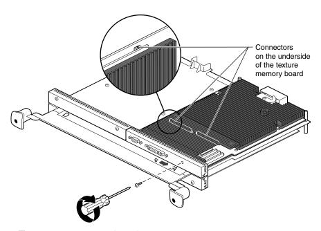
Figure 5-35 Inserting the Nylon Screw
