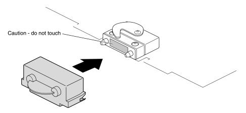
**Figure 2-10** Placing the Compression Cap on the Compression Connector
