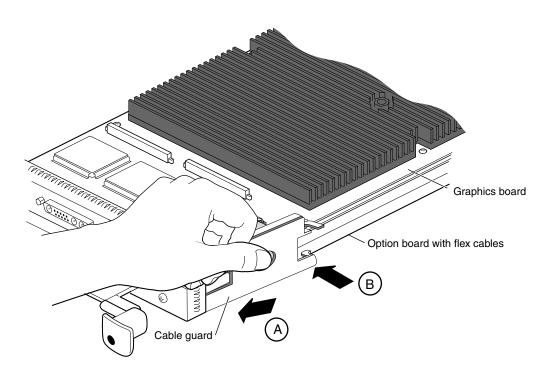
**Figure 5-27** Sliding the Cable Guard Under the I/O Panels
