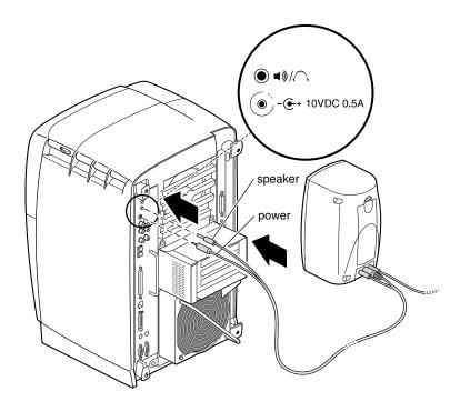
**Figure 1-9** Connecting the Speaker and Power Cables
