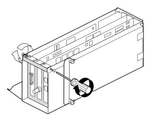
**Figure 4-25** Inserting and Tightening the I/O Door Screws
