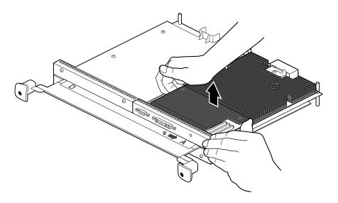
**Figure 5-37** Releasing the Texture Memory Option Board From the Graphics Board
