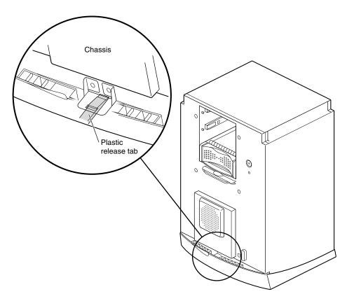
**Figure 7-32** Locating the Release Slots
