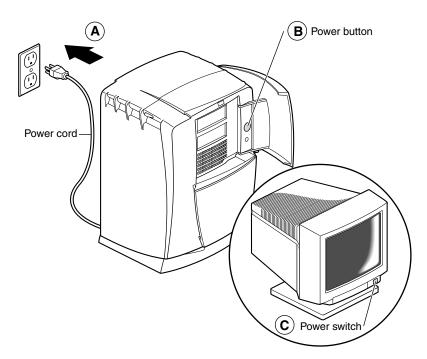
Figure 4-48 Replacing the Power Cord and Turning On the OCTANE Workstation
