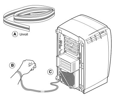
**Figure 4-5** Attaching the Wrist Strap to the Chassis
