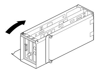
Figure 4-35 Closing the I/O Door
