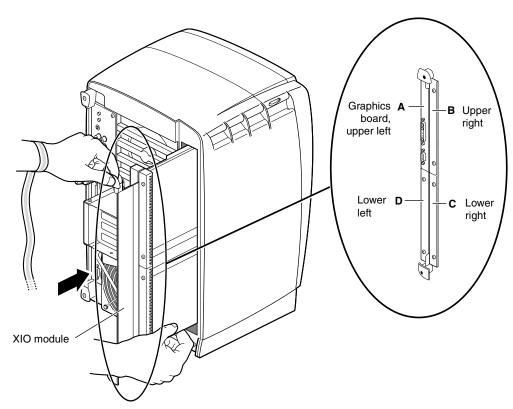
Figure 5-40 Replacing the XIO Module
