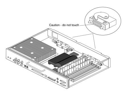
**Figure 2-9** Locating the Compression Connectors
