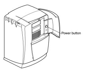
**Figure 1-23** Powering Off the OCTANE Workstation
