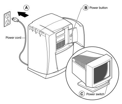
**Figure 6-9** Powering On the OCTANE Workstation
