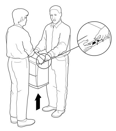
Figure 1-4 Lifting the OCTANE Workstation
