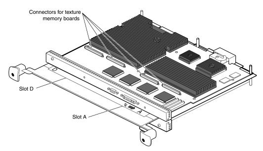
**Figure 5-33** Locating the Connectors for the Texture Memory Option Board on the OCTANE/SSI Graphics Board
