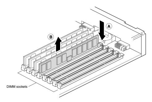
Figure 2-19 Removing a DIMM
