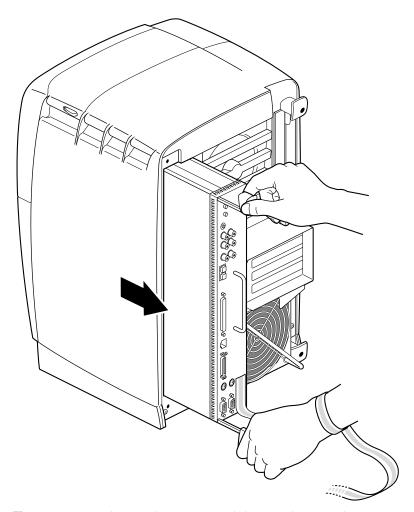
**Figure 2-7** Releasing the System Module From the Frontplane
