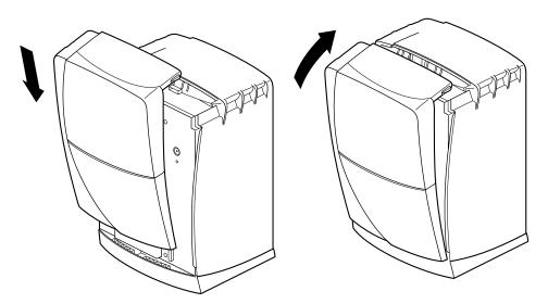
**Figure 7-36** Replacing the Bezel
