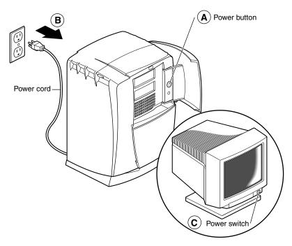
**Figure 4-3** Powering Off the OCTANE Workstation
