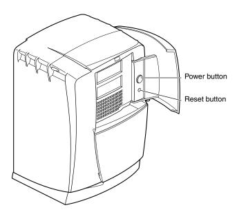
Figure 9-6 Pressing the Reset Button
