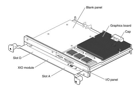
Figure 5-9 Placing the XIO Module on Its Side
