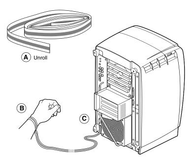
**Figure 2-4** Attaching the Wrist Strap to the Chassis
