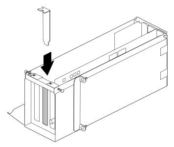
Figure 4-37 Inserting the I/O Blank Panel
