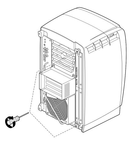
**Figure 5-42** Replacing the XIO Module Screws
