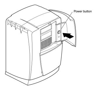
**Figure 1-15** Powering On the OCTANE Workstation
