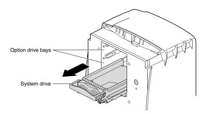
**Figure 7-16** Removing the System Drive
