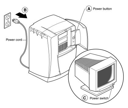
**Figure 6-2** Powering Off the OCTANE Workstation
