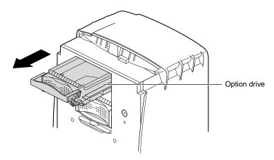
Figure 7-12 Sliding Out the Option Drive
