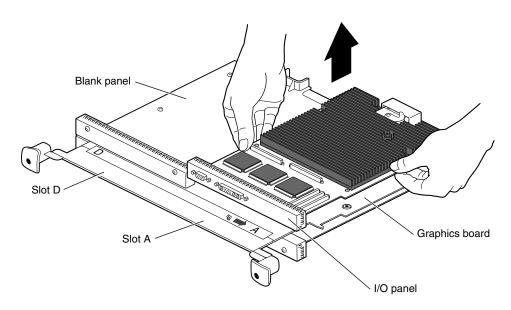
Figure 5-20 Removing the Graphics Board
