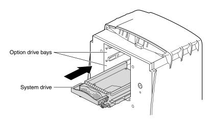
Figure 7-17 Inserting the New Drive
