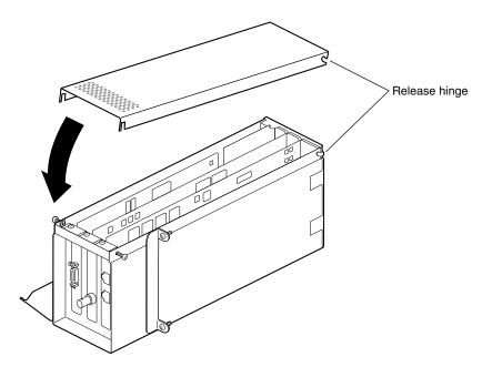
Figure 4-18 Placing the Door on the PCI Module
