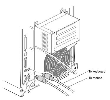
Figure 6-19 Disconnecting the Mouse and Keyboard
