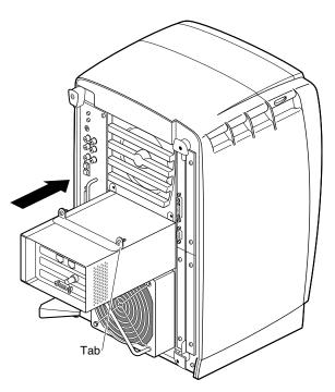
**Figure 4-44** Replacing the PCI Module
