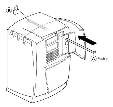
Figure 2-28 Installing the Lockbar
