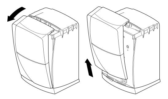
Figure 7-5 Removing the Bezel
