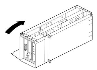
Figure 4-24 Closing the I/O Door
