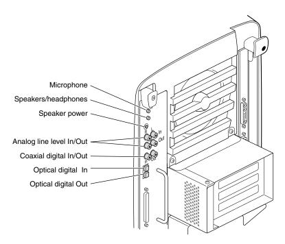
**Figure 6-14** Audio Ports on the System Module
