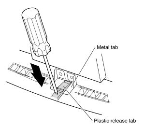
**Figure 7-33** Releasing the Plastic Base
