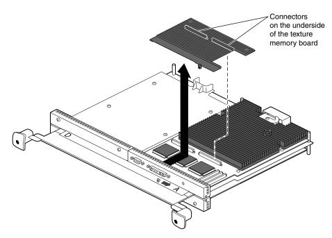
Figure 5-38 Removing the Texture Memory Option Board
