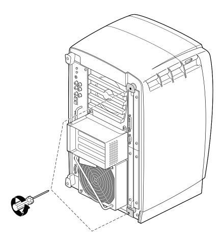
**Figure 5-6** Removing the XIO Module Screws
