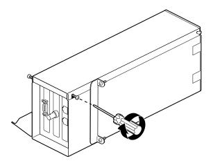
Figure 4-19 Tightening the PCI Module Door Screws
