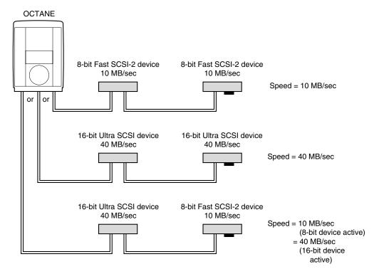
**Figure 6-5** Comparing Speed of Daisy-Chained Devices
