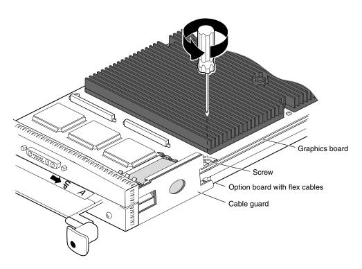
Figure 5-13 Removing the Standoff Screw
