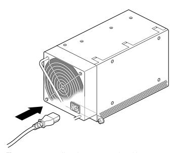
**Figure 3-5** Installing the Power Supply Cable
