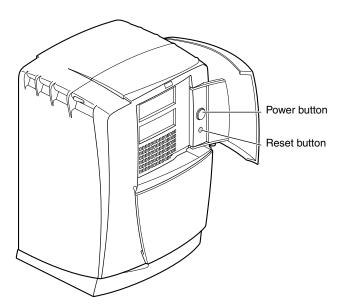
Figure 9-11 Pressing the Power Button
