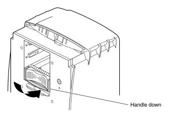
Figure 7-18 Locking the System Drive
