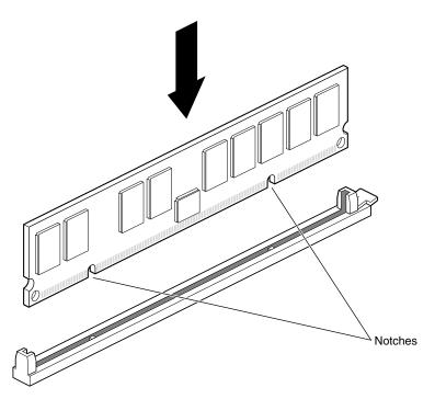
**Figure 2-20** Locating the Notches on a DIMM
