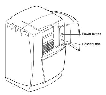
Figure 1-26 Pressing the Power Button
