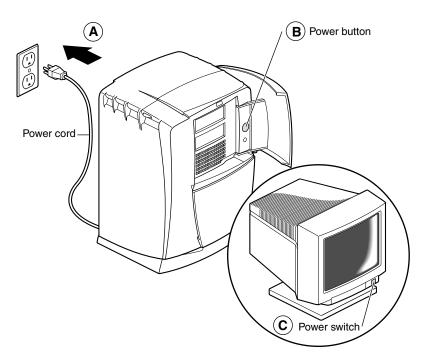
**Figure 6-20** Powering On the OCTANE Workstation
