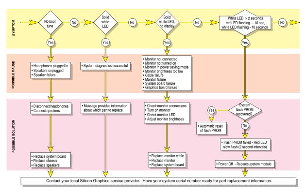
Figure 9-2 Lightbar LEDs - Front of OCTANE, Diagnostic Chart #2
