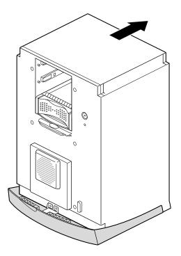
Figure 7-34 Sliding the Chassis Backward
