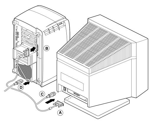
Figure 1-11 Connecting the Monitor and Power Cables
