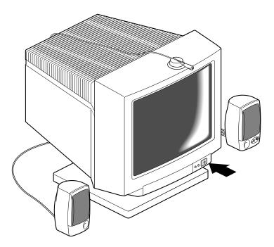
**Figure 1-13** Powering On the Monitor
