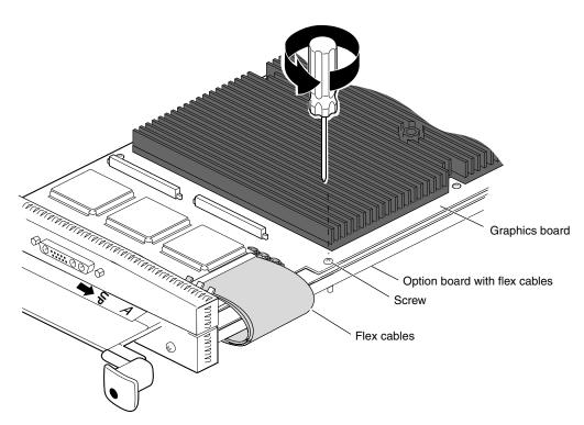
**Figure 5-26** Removing the Screw From the Graphics Board
