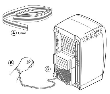
Figure 5-4 Attaching the Wrist Strap
