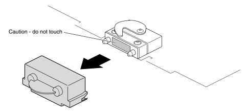
**Figure 4-43** Removing the Cap From the Compression Connector
