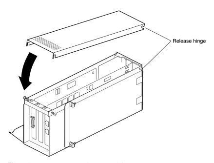
Figure 4-39 Reconnecting the PCI Module Door
