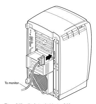
**Figure 5-43** Replacing the Monitor Cable
