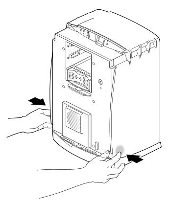
**Figure 7-30** Releasing the Plastic Top Cover
