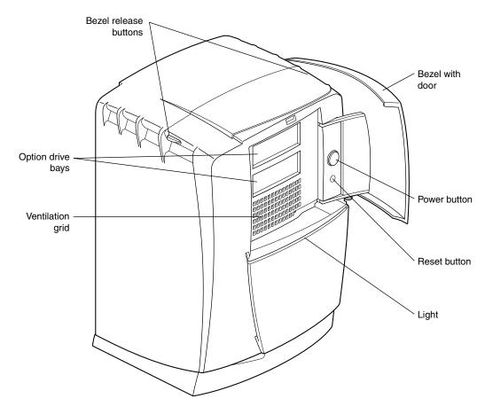
Figure 1-1 Front View of the OCTANE Workstation
