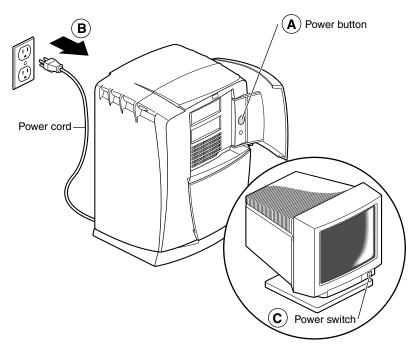
**Figure 2-1** Powering Off the OCTANE Workstation
