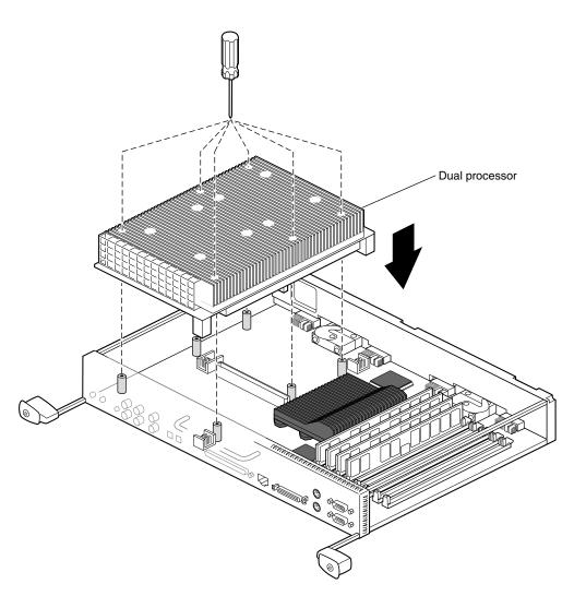
**Figure 2-16** Installing the Dual Processor
