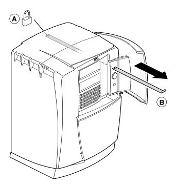
Figure 2-2 Removing the Lockbar
