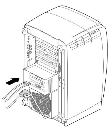
**Figure 4-47** Replacing the PCI Cables
