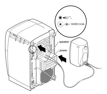
**Figure 6-18** Attaching the Speaker Cables to the OCTANE Workstation
