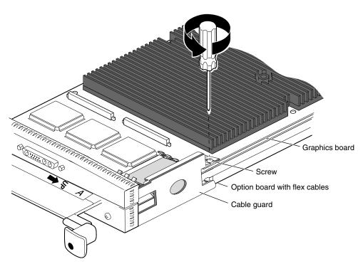
**Figure 5-29** Attaching the Screw to Anchor the Cable Guard
