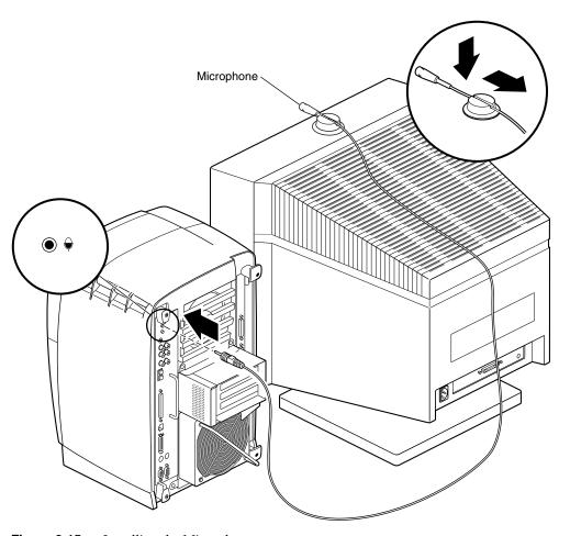
Figure 6-15 Installing the Microphone
