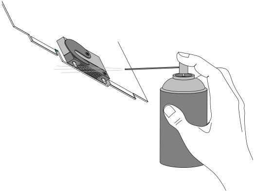
**Figure B-2** Spraying the Compression Connector
