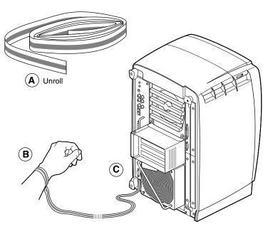
Figure 7-22 Attaching the Wrist Strap
