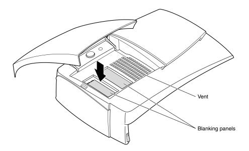
Figure 7-10 Pushing the Blank Panel Free
