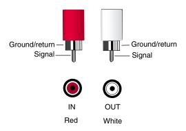
The port (jack) pinout for the coaxial digital ports and plugs are shown above.
