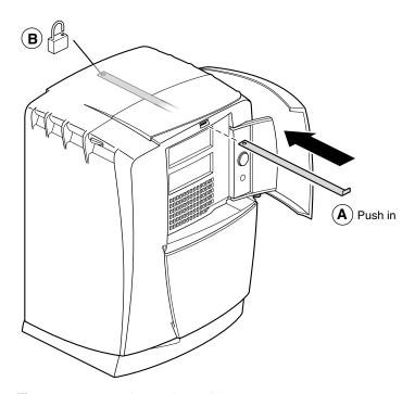
Figure 7-37 Replacing the Lockbar
