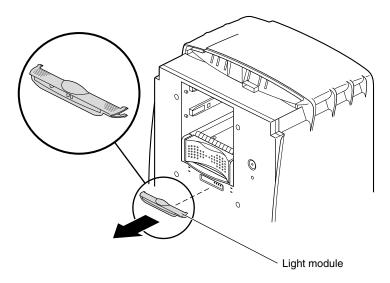
Figure 7-20 Removing the Light Module
