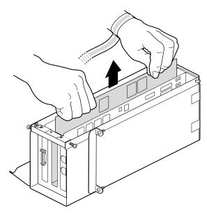
Figure 4-30 Extracting the PCI Board
