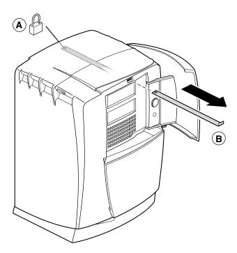
Figure 7-3 Unlocking and Removing the Lockbar
