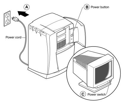
**Figure 2-27** Powering On the OCTANE Workstation
