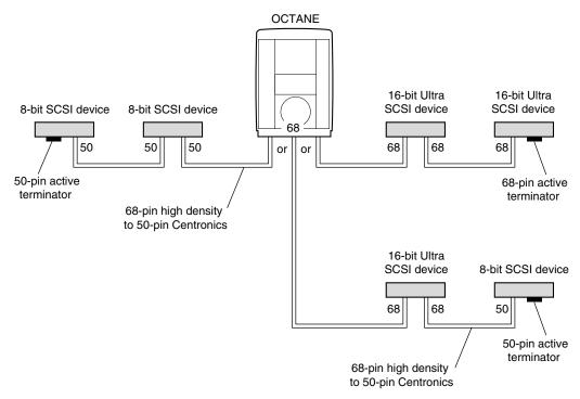
Figure 6-4 Using the Correct Cables Between Devices and/or the OCTANE Workstation
