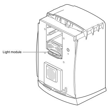
Figure 7-19 Locating the Light Module
