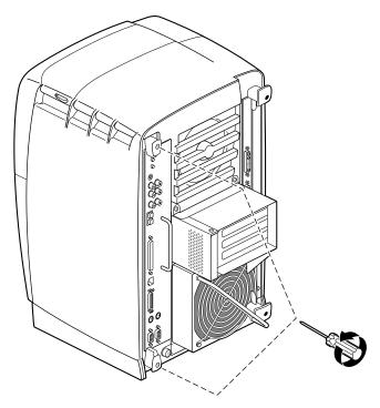
Figure 2-5 Removing the System Module Screws
