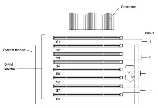
Figure 2-17 Identifying DIMM Sockets and DIMM Banks
