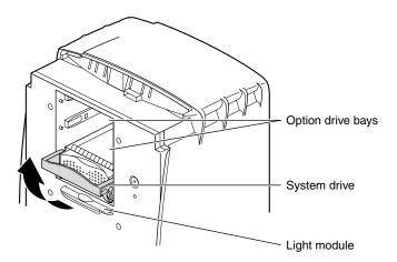
Figure 7-15 Unlocking the System Drive
