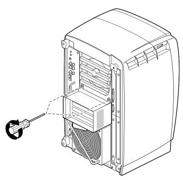
**Figure 4-7** Removing the Screws From the PCI Module
