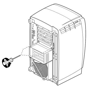
Figure 4-46 Replacing the PCI Screws
