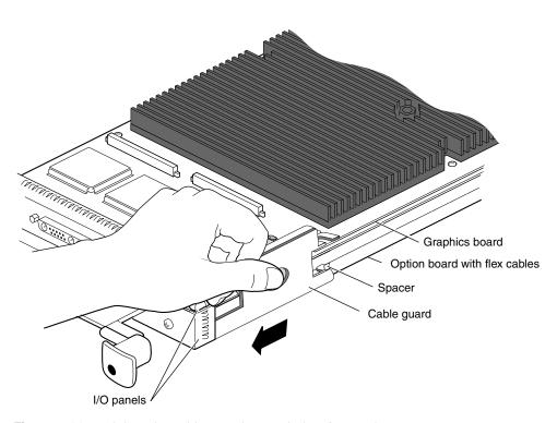
**Figure 5-14** Sliding the Cable Guard Beneath the I/O Panel
