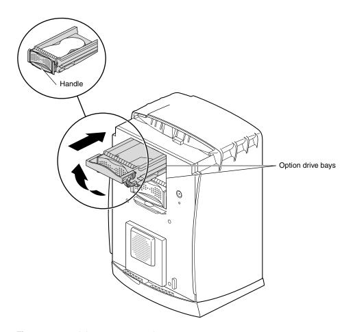
Figure 7-7 Sliding In an Optional Drive
