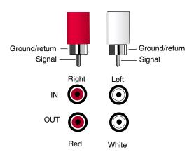
The pinouts for the analog audio ports and plugs are shown above.
