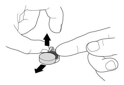
**Figure 7-25** Sliding Out the System Identification Module
