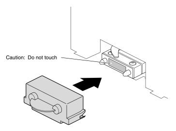
**Figure 4-10** Installing a Cap on the Compression Connector
