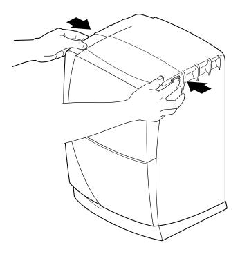
Figure 7-4 Pressing the Bezel Release Buttons
