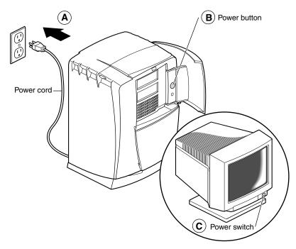
**Figure 5-44** Powering On the OCTANE Workstation
