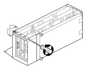
**Figure 4-32** Removing the I/O Door Screws
