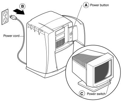
**Figure 5-2** Powering Off the OCTANE Workstation
