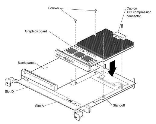
Figure 5-22 Replacing the Screws
