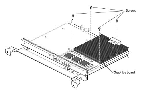
Figure 5-19 Removing the Screws From the XIO Board
