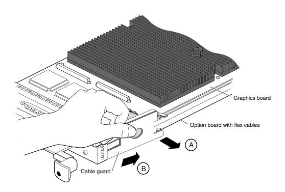
**Figure 5-15** Removing the Cable Guard
