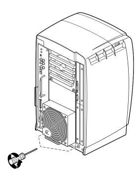
**Figure 3-2** Removing the Screws That Hold the Power Supply to the Chassis
