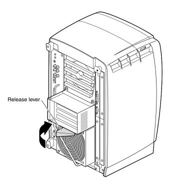
Figure 4-45 Closing the Release Lever
