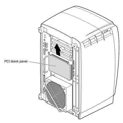
Figure 4-42 Removing the Blank Panel
