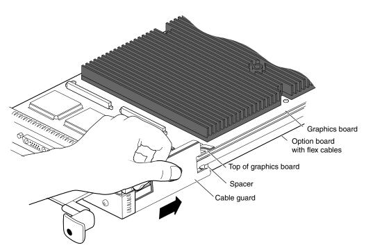
Figure 5-28 Sliding the Cable Guard Behind the Standoff
