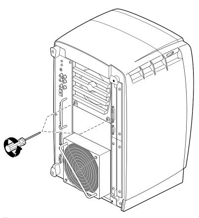
**Figure 4-41** Removing the Screws From the Blank Panel
