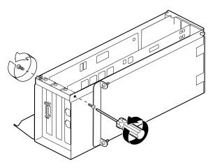
Figure 4-21 Removing the PCI Module Door Screws
