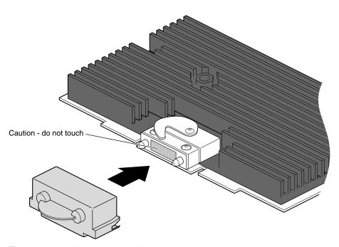
**Figure 5-10** Placing a Cap on the XIO Compression Connector
