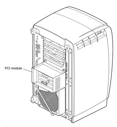
Figure 4-2 Workstation With the Optional PCI Module
