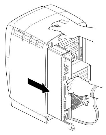
**Figure 2-8** Removing the System Module From the Chassis
