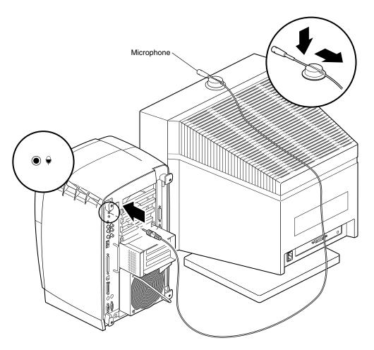
**Figure 1-10** Attaching the Microphone
