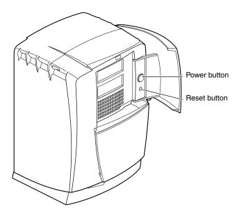
Figure 1-25 Pressing the Reset Button
