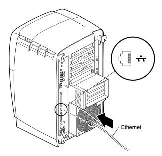
**Figure 1-6** Attaching the Ethernet Cable
