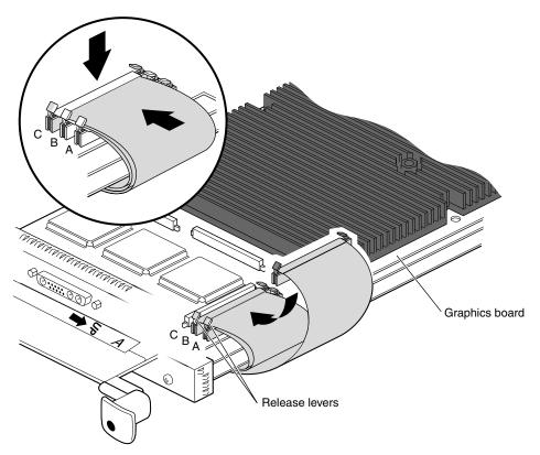
**Figure 5-23** Attaching the Option Board Flex Cables to the Graphics Board
