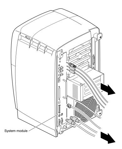
**Figure 2-3** Removing the Cables From the System Module
