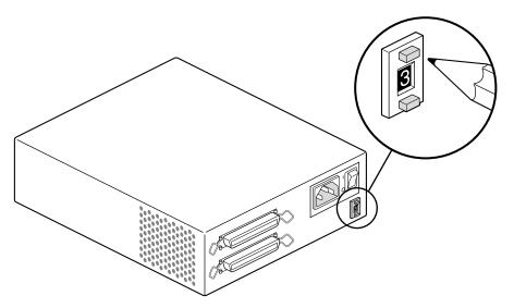
Figure 6-1 Manually Setting the SCSI Address
