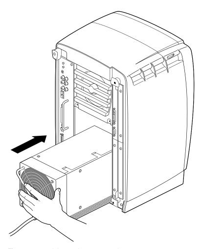
Figure 3-6 Sliding In the Power Supply
