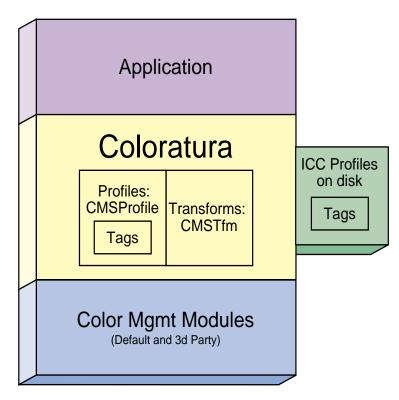
Figure 1-1 Components of a Color-Management Application
