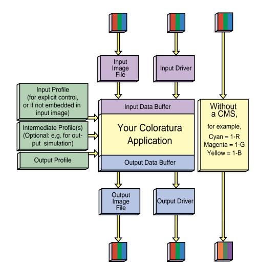
Figure 1-2 Data Flow for a Typical Color-Management Application
