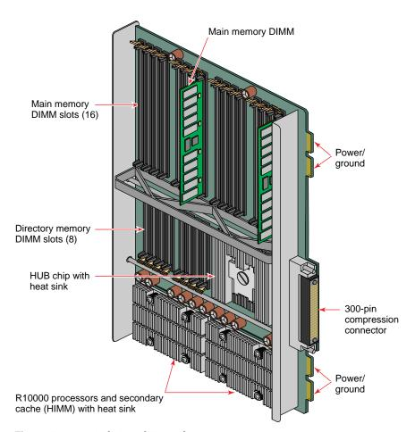
Figure 1-2 Node Board Example
