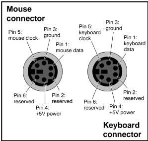
Figure 4-11 Keyboard and Mouse Locations and Pinouts
