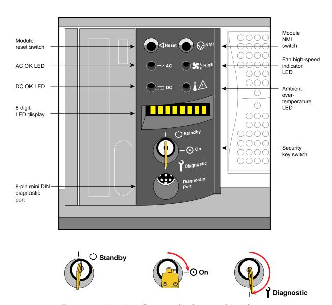
Figure 3-6 System Controller Keyswitch and Front-Panel Controls
