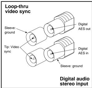
Figure 4-15 Loopthrough and Digital Audio Connectors
