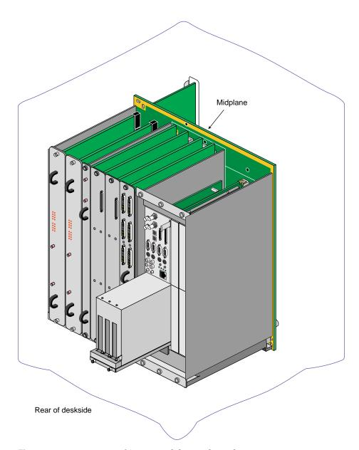
Figure 2-2 Rear View of System Midplane and Boards
