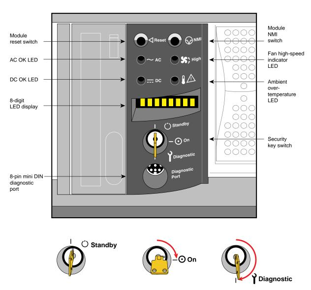
Figure 6-2 Controller Status Panel and Switches
