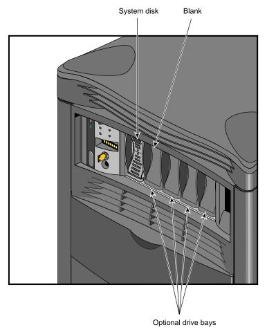
Figure 3-4 Deskside System Internal Drive Bays
