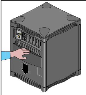
**Figure 2-3** Opening the Front of the Onyx2 Deskside System
