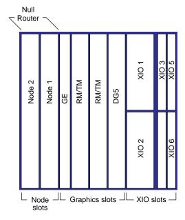
Figure 1-4 System Board Locations Diagram
