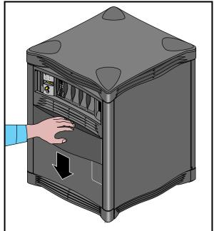
Figure 3-1 Opening and Closing the Sliding Front Panel
