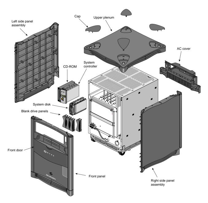
Figure 2-1 Deskside System Components
