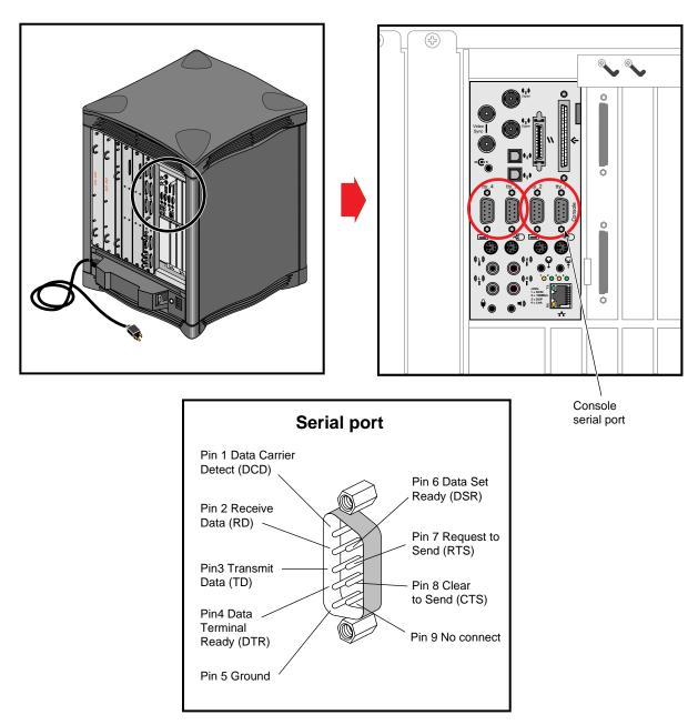
Figure 4-13 RS-232/RS-422 Serial Connectors
