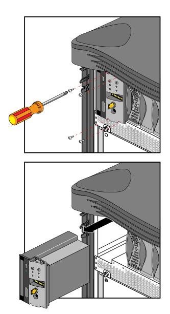
Figure 5-3 Install or Replace the System Controller or CD-ROM Drive
