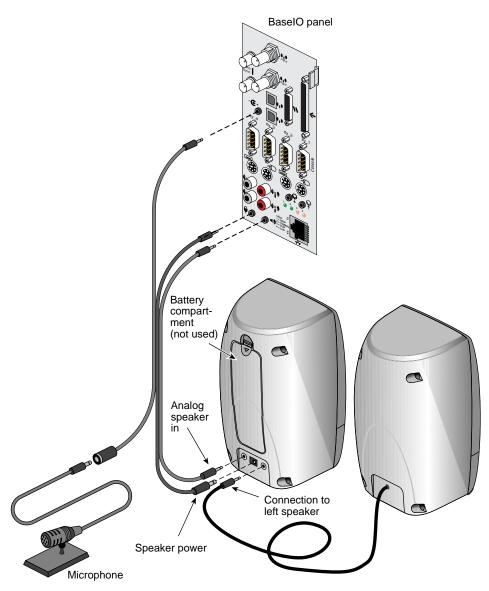
Figure 4-18 Speaker and Microphone Connections to the BaseIO
