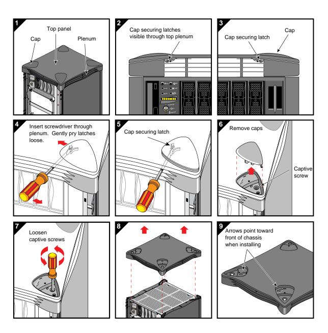
Figure 3-3 Removing the Top Plastic Panel
