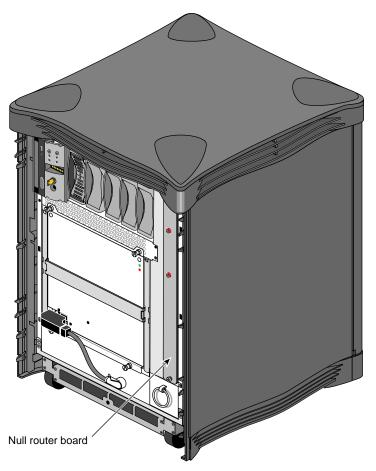
Figure 2-6 Null-Router Board Location
