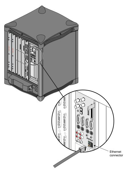
Figure 3-5 Connecting an Ethernet Cable
