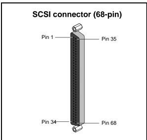
Figure 4-16 68-Pin Single-Ended SCSI Connector
