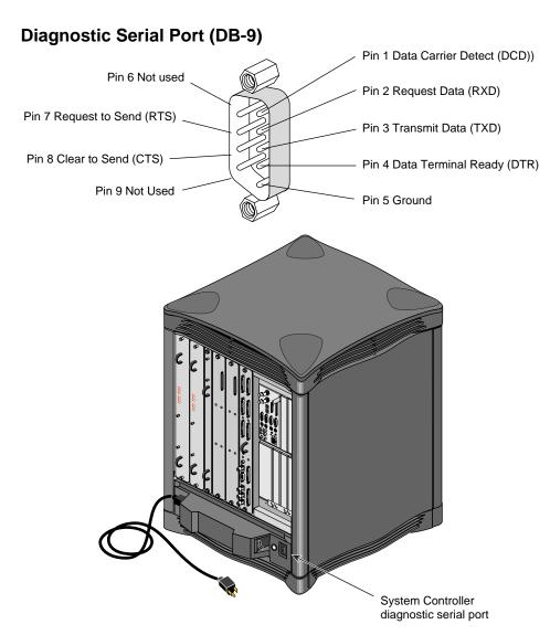
Figure 6-3 System Controller Rear Serial Console Connector
