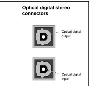
Figure 4-14 Optical Digital Audio Interface
