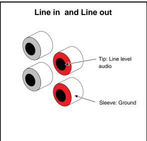
Figure 4-12 Analog Stereo Port Locations
