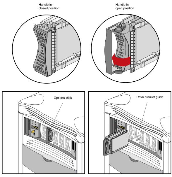
Figure 5-2 Removing a Data Disk Drive Module
