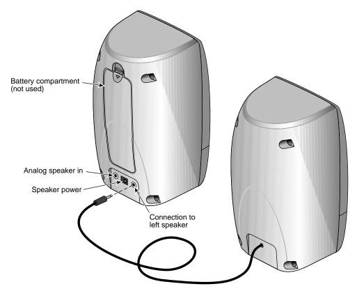
Figure 4-17 Cable Connection Locations on the Speakers
