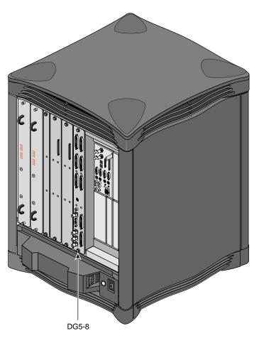
Figure 4-1 shows connectors on the DG5-8 option board with the VIO5H daughterboard.
