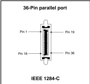
Figure 4-10 Parallel Printer Port Location
