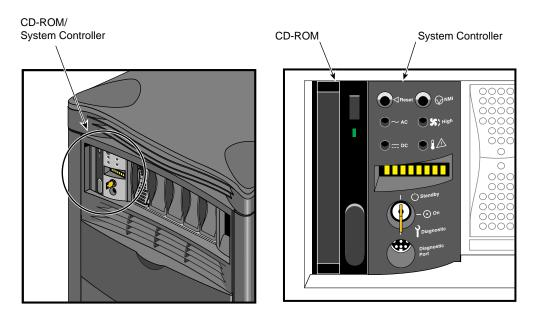
Figure 6-1 System Controller Interface Location
