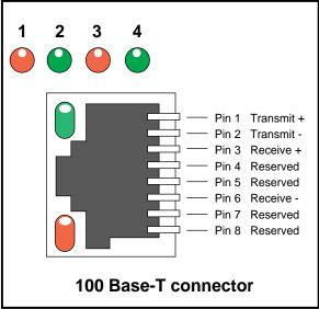
Figure 4-9 10/100 Base-T Ethernet Connector
