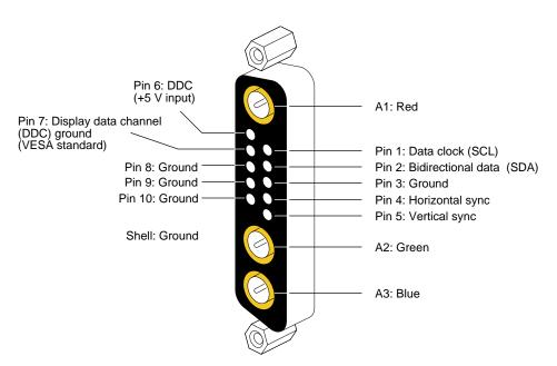
Figure 4-4 DG5/VIO5H 13W3 Connector Pinout
