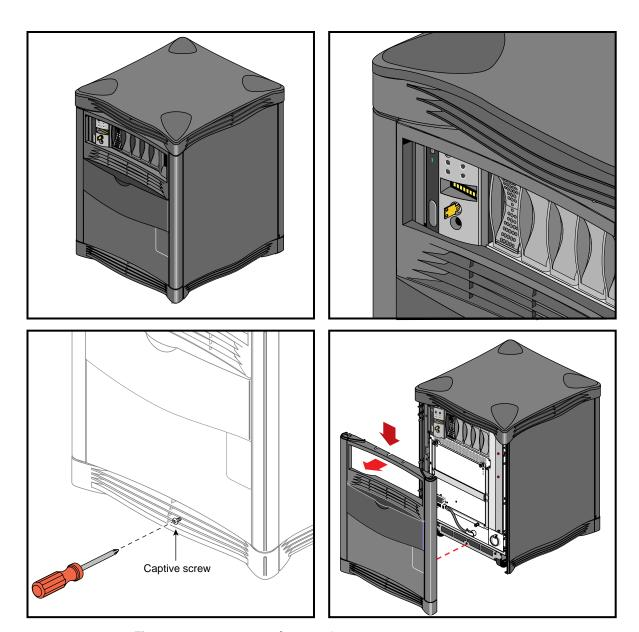
Figure 3-2 Removing the Front Cover
