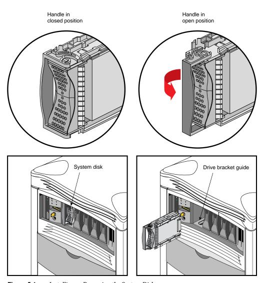
Figure 5-1 Installing or Removing the System Disk
