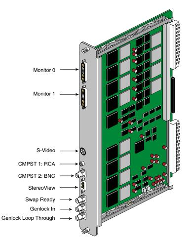
Figure 4-2 DG5 Graphics Panel Connections (Without Options)
