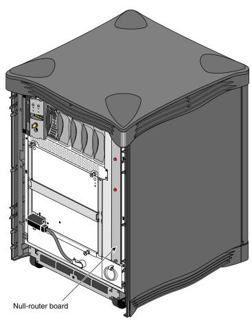
Figure 2-7 Null-Router Board Location
