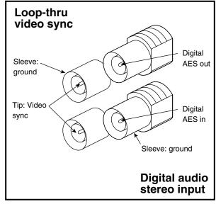
Figure 4-16 Loopthrough and Digital Audio Connectors
