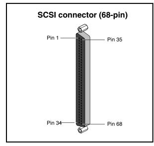
Figure 4-1768-Pin Single-Ended SCSI Connector
