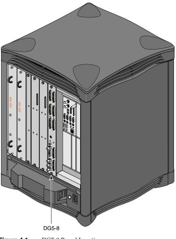
Figure 4-1 shows connectors on the DG5-8 option board with the VIO5H daughterboard.
