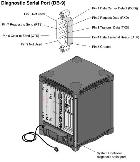
Figure 6-3 MSC Rear Serial Console Connector
