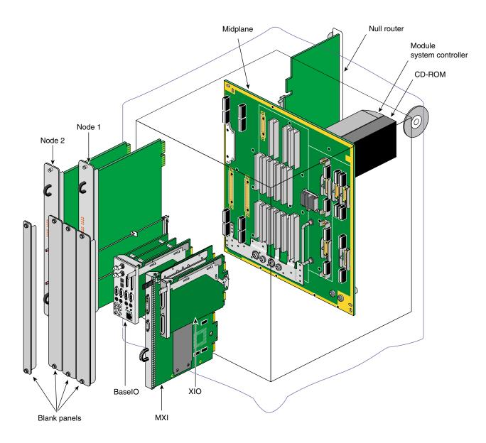
Figure 2-2 Rear View of MXI System Midplane and Boards
