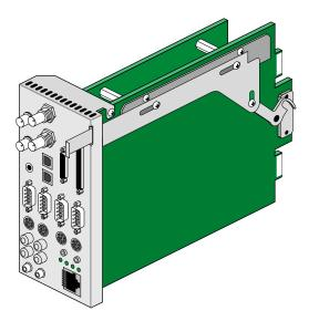
Figure 2-11 Graphics BaseIO Assembly (IO6G) Panel
