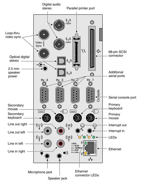
Figure 4-9 BaseIO (IO6G) Panel and Connectors
