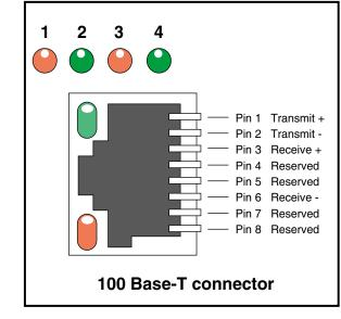
Figure 4-10 10/100 Base-T Ethernet Connector
