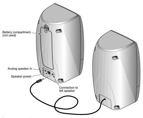
Figure 4-18 Cable Connection Locations on the Speakers
