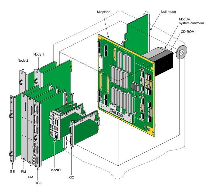
Figure 2-3 Rear View of Onyx2Reality and InfiniteReality System Midplane and Boards
