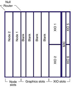
Figure 1-7 MXI System Board Locations Diagram
