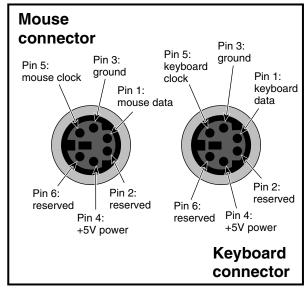
Figure 4-12Keyboard and Mouse Locations and Pinouts
