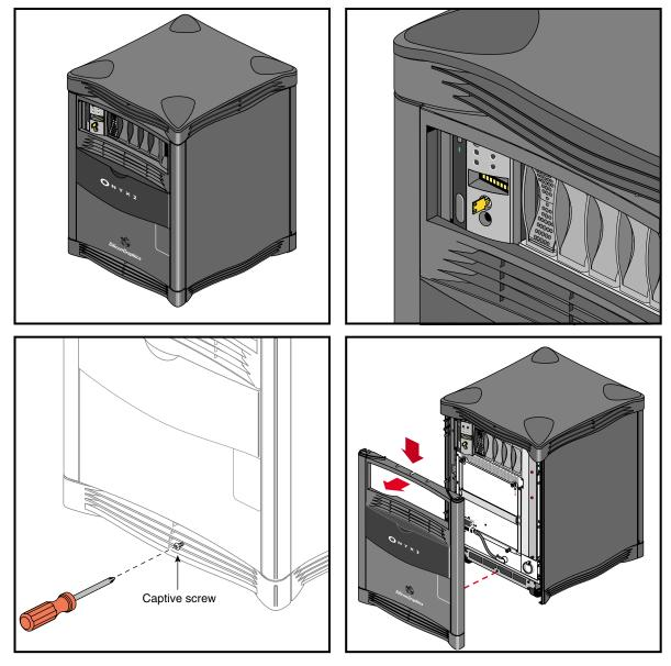
Figure 3-2Removing the Front Cover
