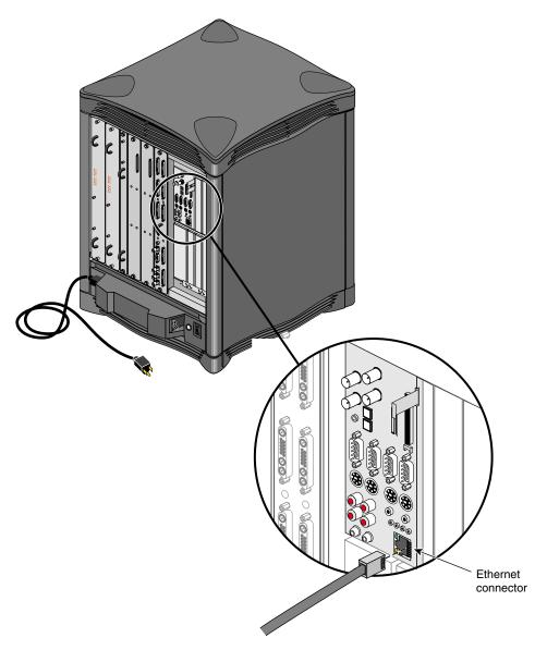
Figure 3-5Connecting an Ethernet Cable
