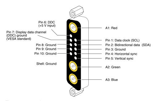
Figure 4-4 shows the 13W3 pinouts for the monitor connectors on the DG5/VIO2 I/O panel. Each 13W3 uses the same pinout pattern.
