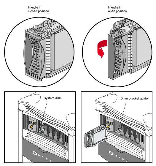
Figure 5-1Installing or Removing the System Disk
