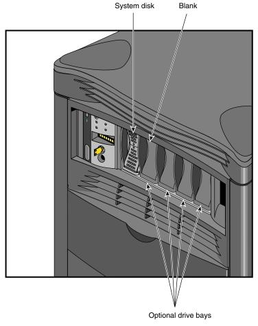
Figure 2-6 System Disk and Optional Drive Bays
