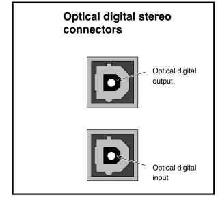
Figure 4-15 Optical Digital Audio Interface
