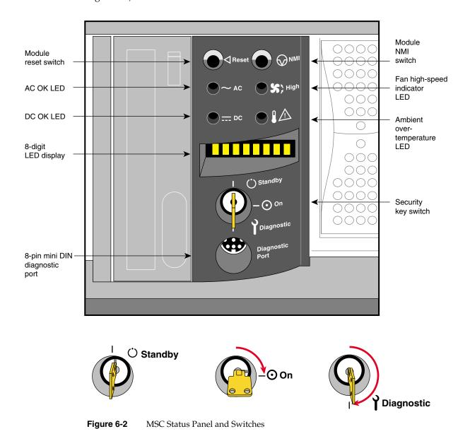
easy user access to switches and displays at the front of the deskside system (see Figure 6-2).
