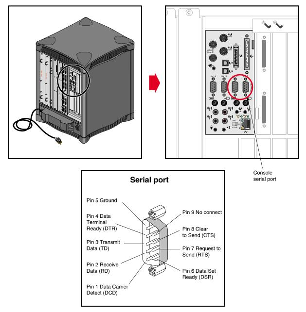
Figure 4-14 RS-232/RS-422 Serial Connectors
