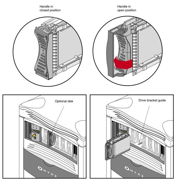
Figure 5-2Removing a Data Disk Drive Module
