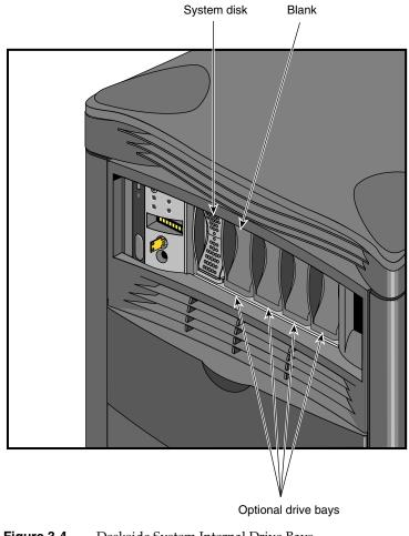
Figure 3-4 Deskside System Internal Drive Bays
