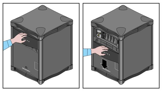
Figure 3-1 Opening and Closing the Sliding Front Panel
