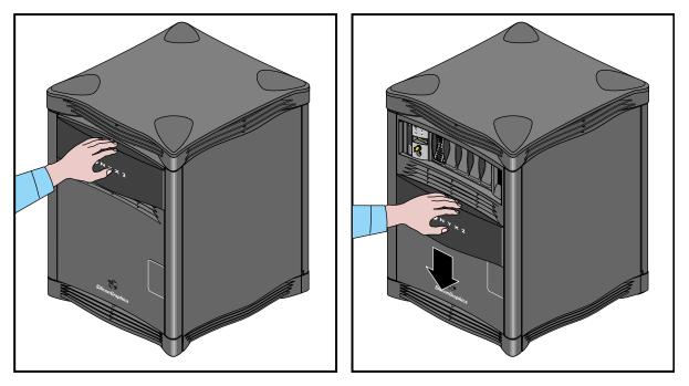
Figure 2-4 Opening the Front of the Onyx2 Deskside System
