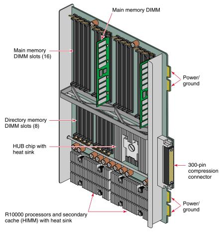
Figure 1-3 Node Board Example
