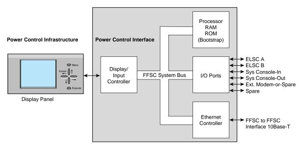
Figure 7-1 Multimodule Controller Functional Block Diagram
