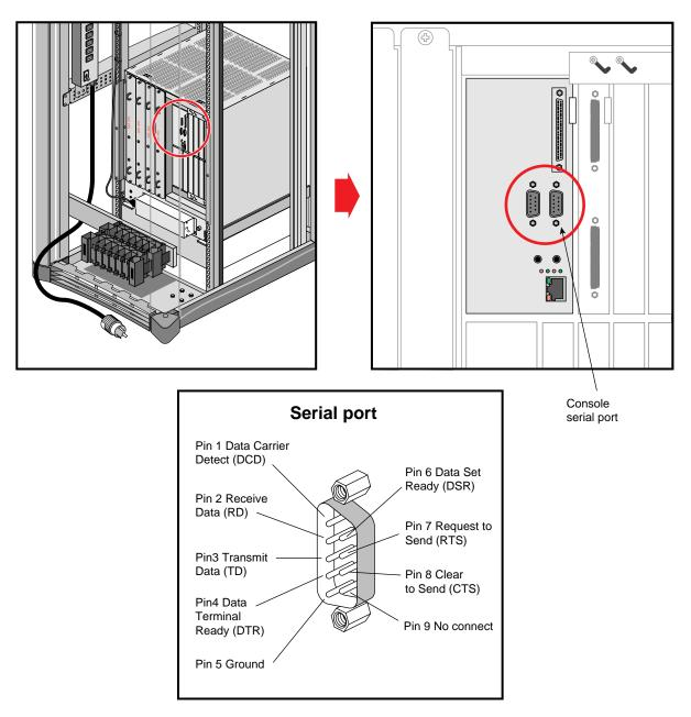
Figure 3-2 Serial Port Location and Pinouts
