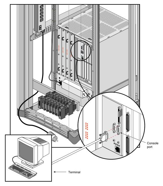
Figure 5-1Connecting a Terminal
