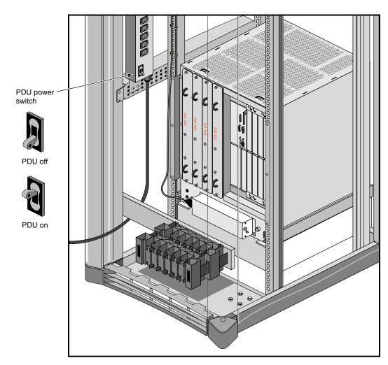
Figure 5-7Turning On the PDU
