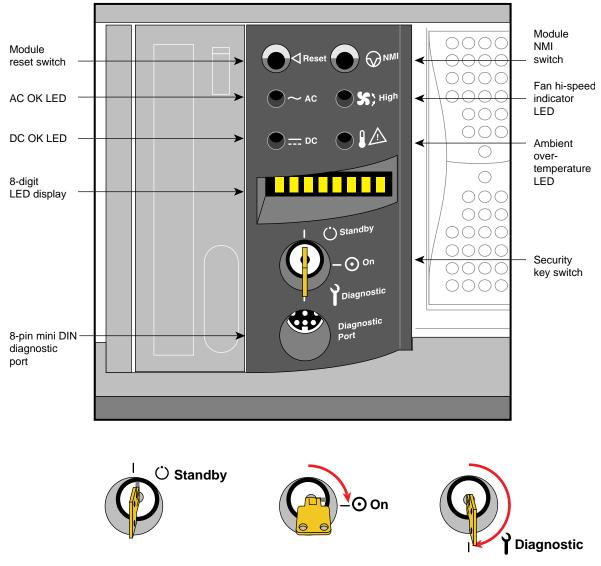
The System Controller front panel is shown in Figure 7-6.
