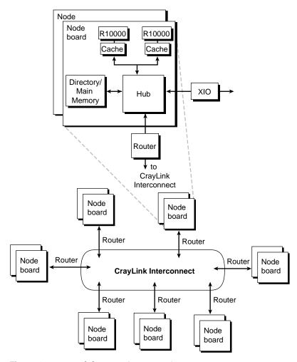
Figure 1-7 Modules in an Origin2000 System
