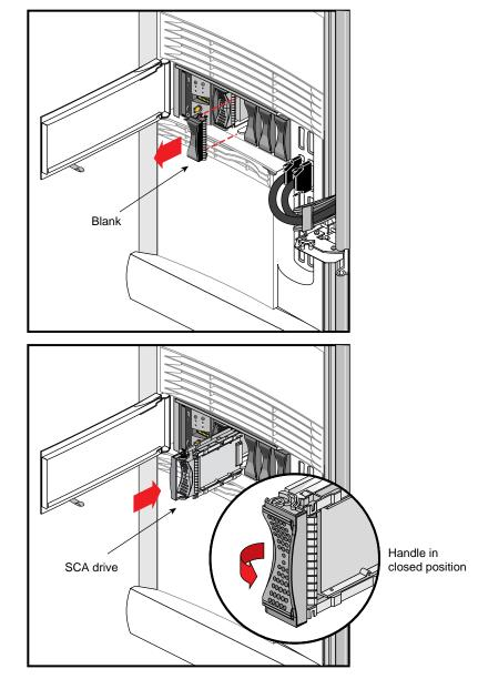
Figure 5-2Installing an SCA Drive
