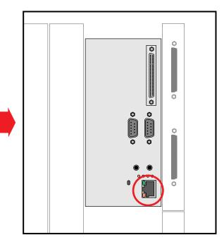
Figure 5-5 Connecting Ethernet to the Origin2000
