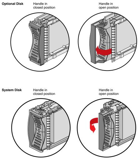
Figure 6-9 Opening the Disk Drive Unit Module
