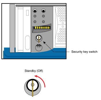
Figure 6-2Turning Off the Module Controller
