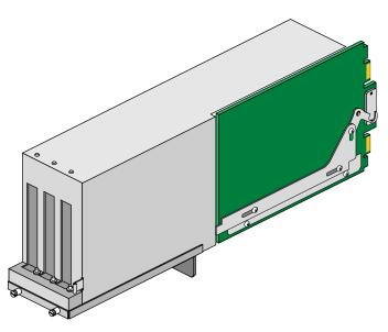
Figure 2-11 Optional PCI Carrier Assembly
