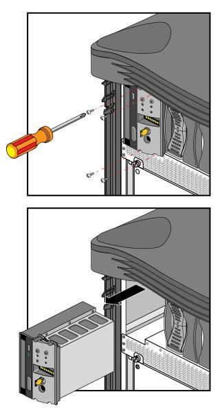
Figure 6-12Removing the System Controller and CD-ROM
