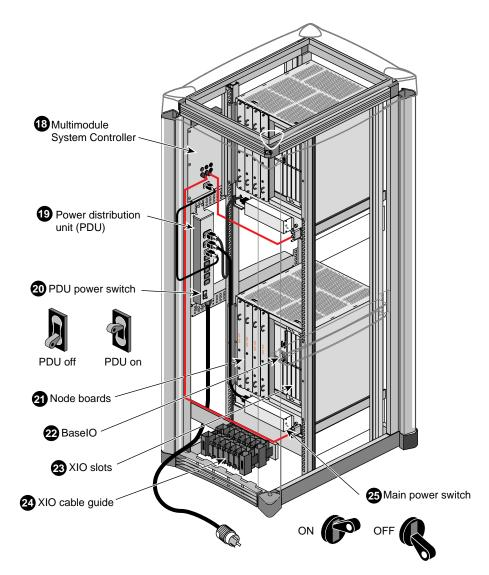
Figure 2-2 Origin2000 Rackmount Rear View
