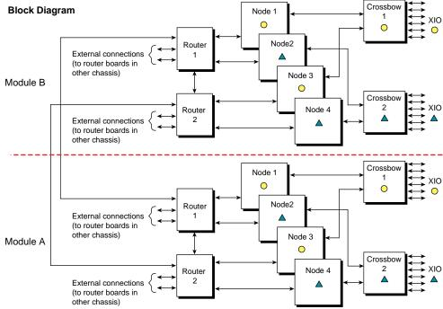
Figure 1-5 Origin2000 Overall Rackmount Block Diagram
