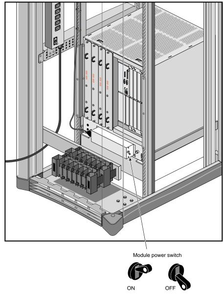
Figure 5-8Powering On the System (Rear View of Chassis)
