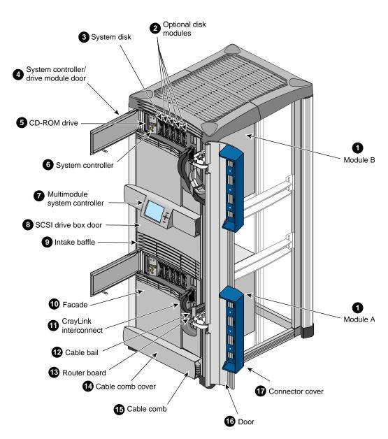
Figure 2-1 Origin2000 Rackmount System (Front View)
