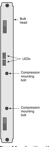
Figure 2-8 Front View of Node Board Showing Bulkhead
