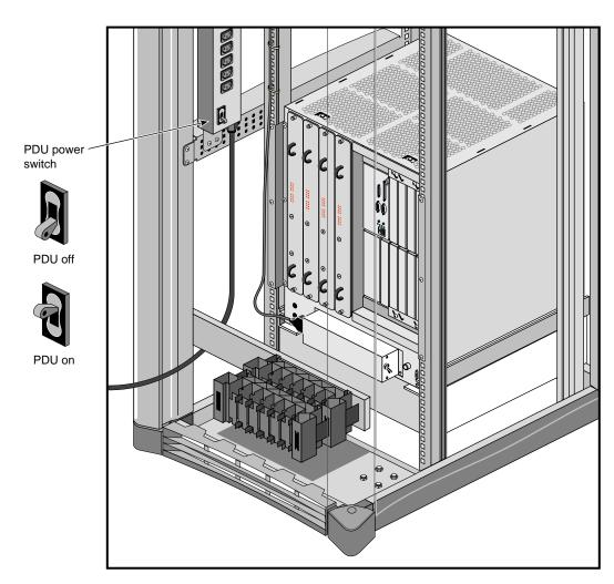
Figure 6-5Turning Off the PDU
