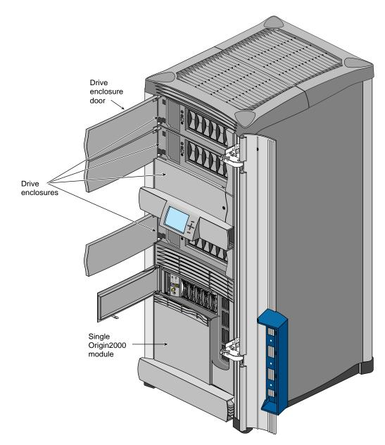
Figure 4-3Single Origin2000 Module in a Rack with Four Origin Vault Drive Boxes
