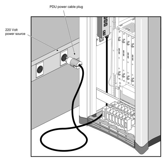
Figure 5-6Connecting the System Power Cable
