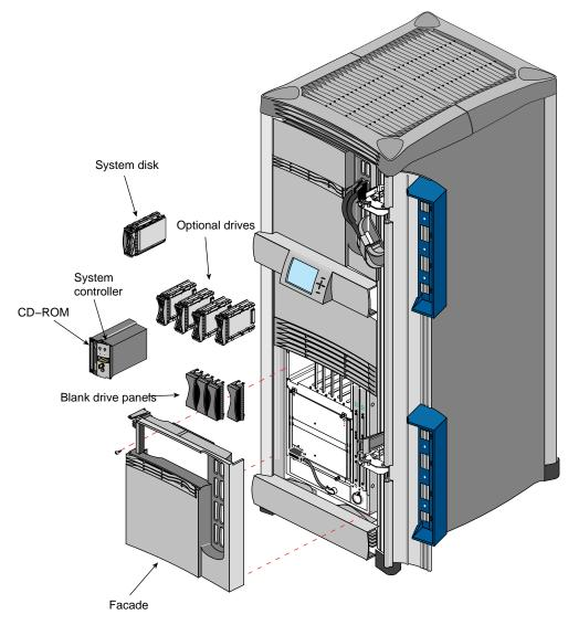
Figure 6-1 Customer-Replaceable Units (CRUs) for the Origin2000 Rackmount System
