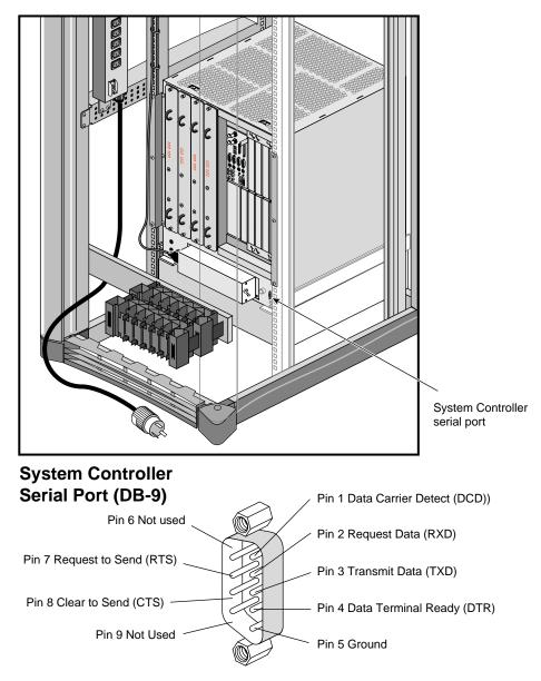
Figure 7-7 System Controller Rear Serial Connector
