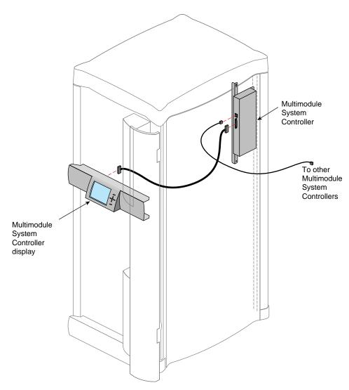
Figure 7-2 The MMSC and Front Panel
