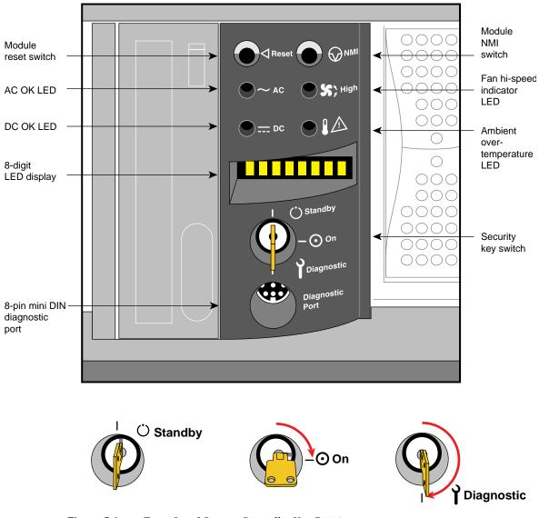
Figure 5-9 Entry-Level System Controller Key Positions
