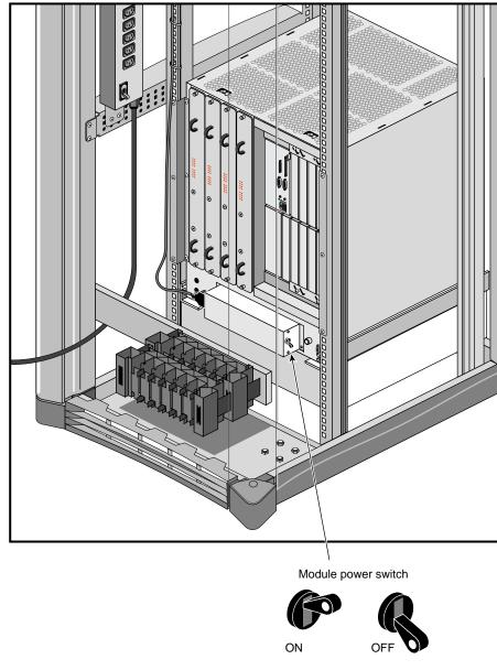
Figure 6-3Powering Off a Rackmount Module
