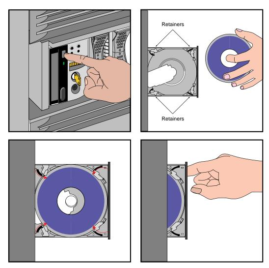
Figure 5-4 Installing a CD-ROM Into an Origin2000 Chassis
