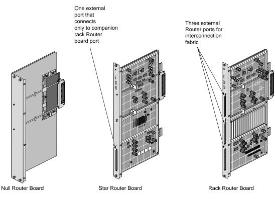
Figure 2-9 Origin2000 Router Boards
