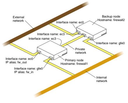
Figure 1-1 Example IRIS FailSafe Gauntlet Configuration
