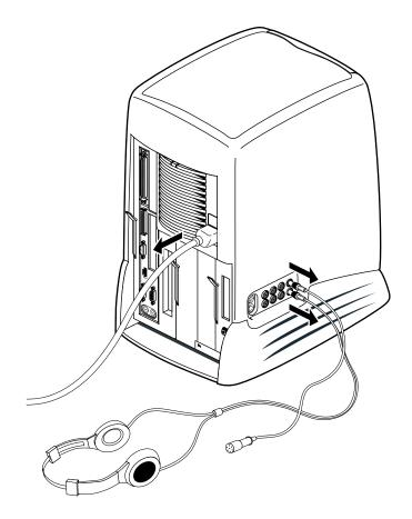
2. Remove the power cable and any cables that are connected to the side of the audio module. The audio module is on the extreme right as you face the rear of the workstation.
