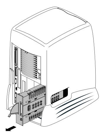
3. Remove the audio module by pulling down the lever and sliding it out of the chassis.
