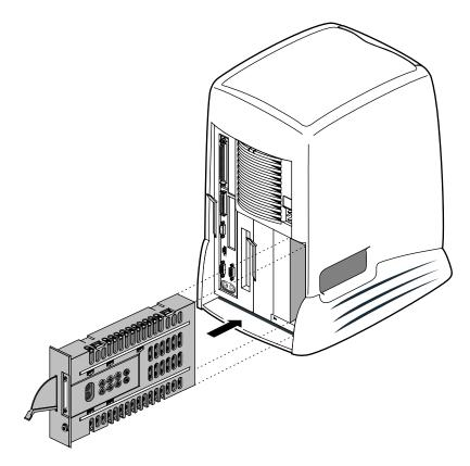
4. Slide the new audio-visual module into the chassis and push the lever up to lock the module in place.
