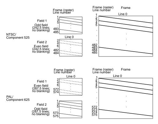
Figure 2-2 Fields and Frames for NTSC and PAL
