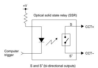
Typical OFF resistance: 5000 G ohms Typical ON resistance: 10 ohms
