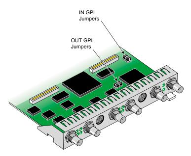
**Figure A-3** GPI Jumper Locations (Factory Setting)
