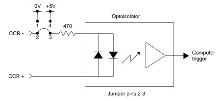
**Figure A-7** Jumpering for GPI Current Sense Mode
