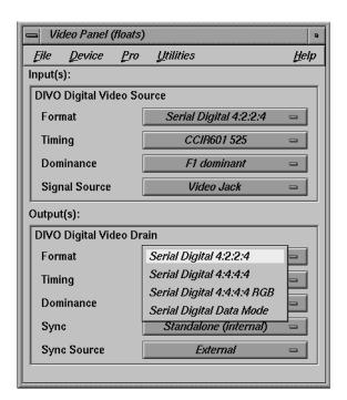
Figure C-3 Selecting Video Drain Format
