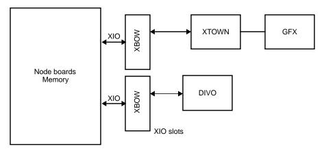
Figure 1-3 DIVO Video Top-Level System Diagram (Onyx2 System)
