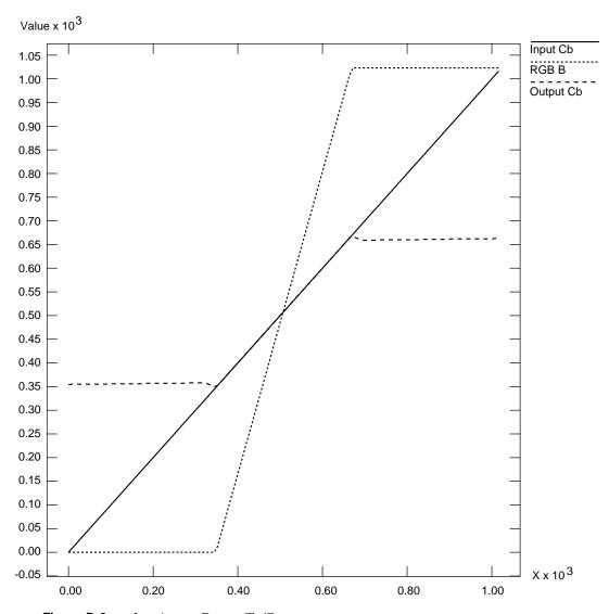
Figure D-8 Luminance Ramp: Cb/B
