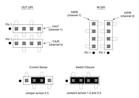
Figure A-4 Example GPI Interface
