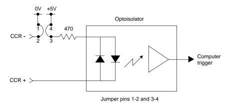
**Figure A-6** Jumpering for GPI Switch Closure (Factory Setting)
