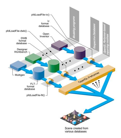
**Figure 2-3** Relationship of OpenGL Performer to Database Formats
