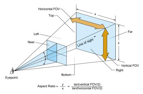
Figure 4-3 Camera with Viewing Volume
