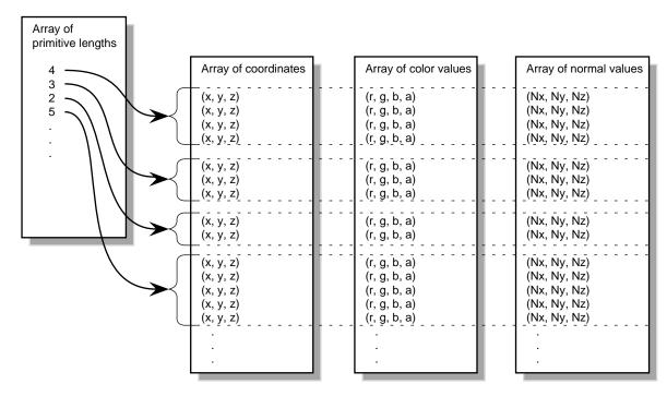
Figure 7-2 Arrays of Stripped Primitives
