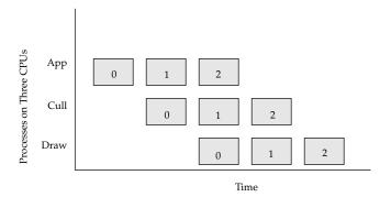
**Figure 4-4** Multiprocessing Frames in the Pipe
