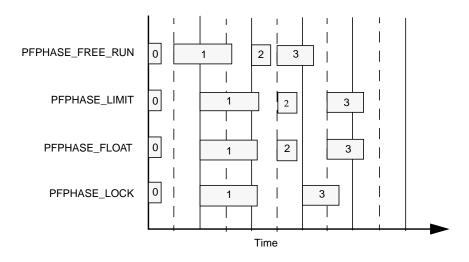
**Figure 10-3** Phase Control over Three Frames
