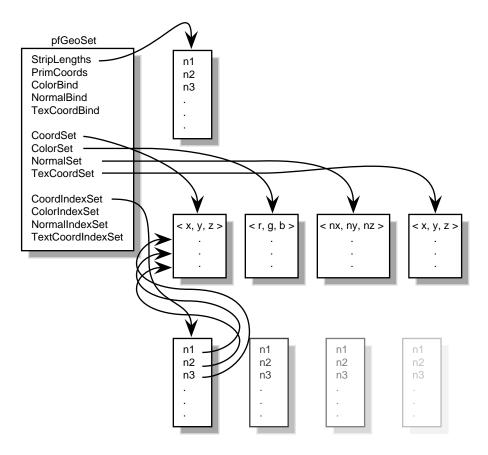
Figure 7-3 Indexing Arrays
