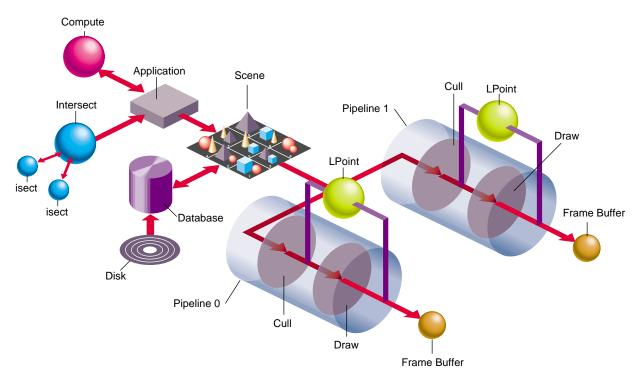
Figure 11-1 OpenGL Performer Stages
