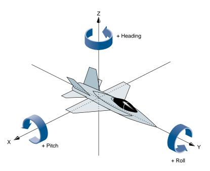
Figure 5-4 Heading, Pitch, and Roll Values
