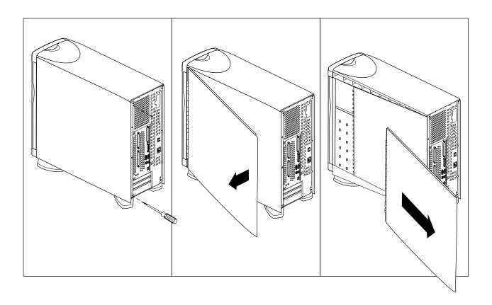
**Figure 1-4** Removing the System Cover
