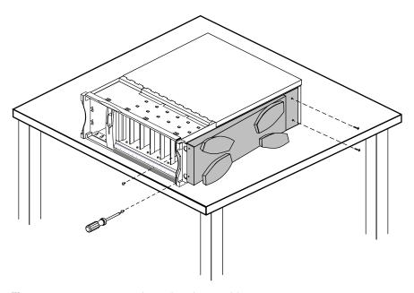
Figure 1-7 Removing the Pedestal Assembly
