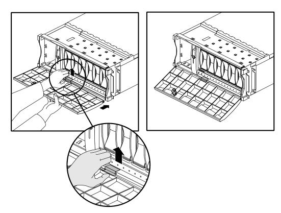
Figure 1-12 Replacing the Front Door
