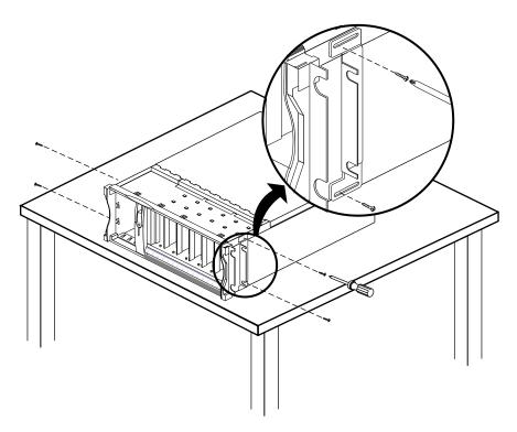
Figure 1-8 Attaching the Mounting Ears
