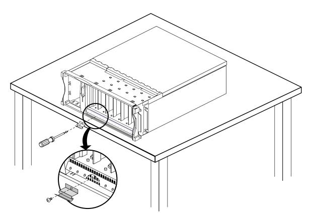
Figure 1-9 Installing the Door Assist Tab
