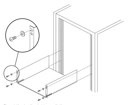
**Figure 1-10** Installing the Mounting Shelf
