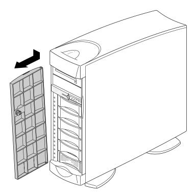
**Figure 1-2** Removing the Front Door
