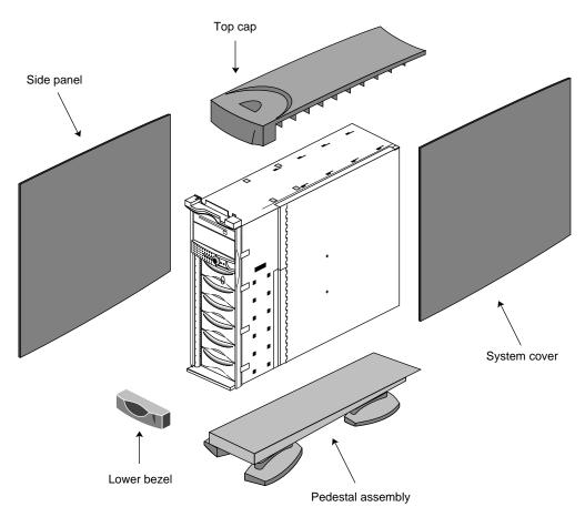
Figure 1-3 Components That Must Be Removed Before Installing the Rackmount Kit
