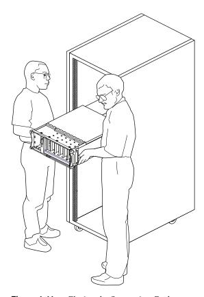
Figure 1-11 Placing the System in a Rack
