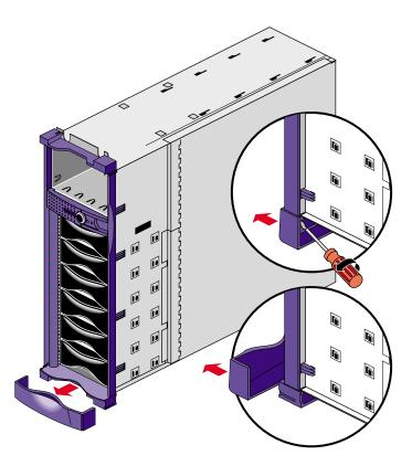
Figure 1-6 Removing the Lower Bezel
