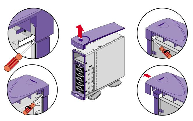
**Figure 1-5** Removing the Top Cap
