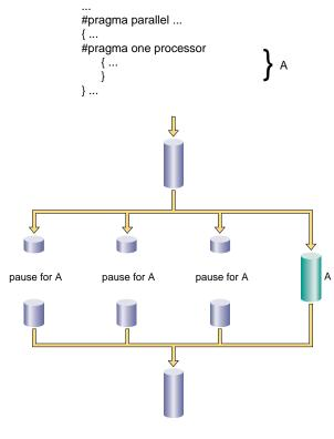
Figure 9-4 One Processor Segment
