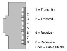
Figure 1-2 PCI Board Style-2 Cable Connector Pin Assignments
