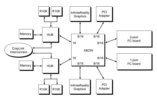
Figure 2-1 Fibre Channel in the Origin 2000 and Onyx2 I/O Structure
