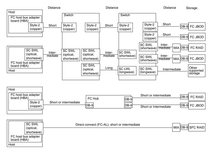
Figure 3-1 Example Connections for SGI Fibre Channel Options
