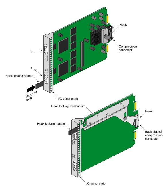
Figure 1-5 Dual-Channel XIO Board and Features (Origin 2000/Onyx2 Version)
