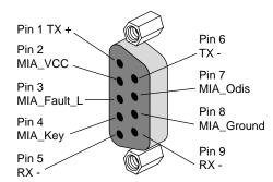
Figure 1-6 Dual-Channel Board Connector Pin Assignments
