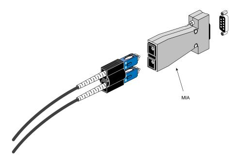
Figure 1-7 Media Interface Adapter (MIA) for Optical Cables
