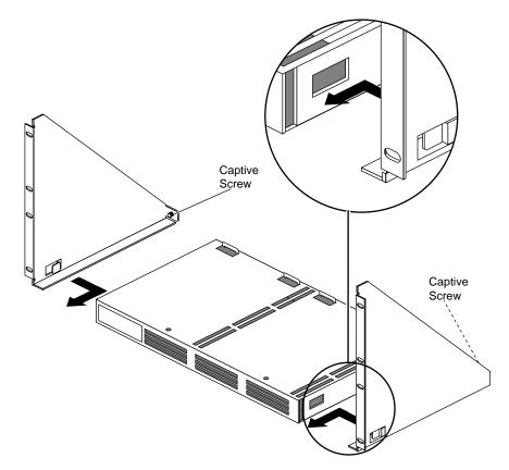
1. Insert each end piece into the appropriate slot on the base.
