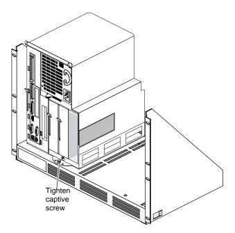
5. Tighten the captive screw on the rear of the workstation to secure it.
