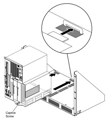
4. Lower the skinless O2 workstation on to the shelf, and slide it toward the rear until the tabs on the workstation engage in the slots.
