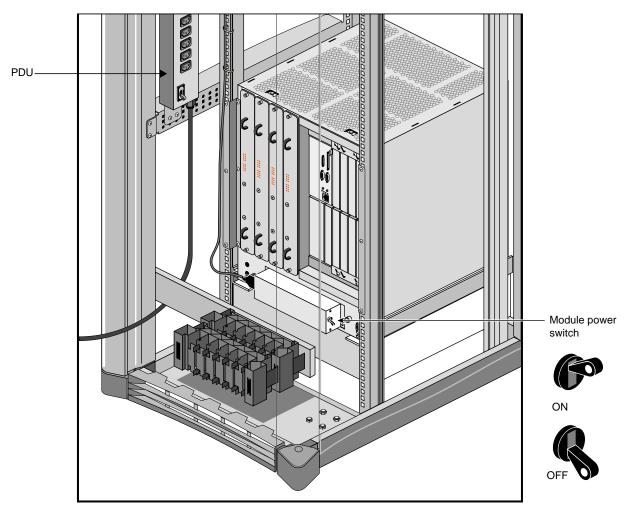
Figure 1-2 Module Main Power Switch
