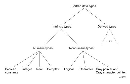
programmer-specified types are built of (or derived from) the intrinsic types and thus are called *derived types*. The Fortran data types are categorized in Figure 4.
