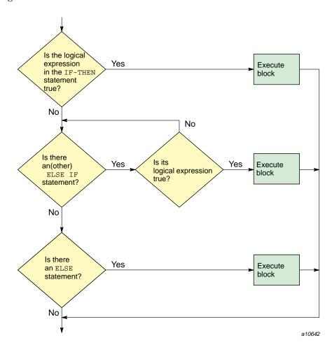
Figure 17. Execution flow for an IF construct
