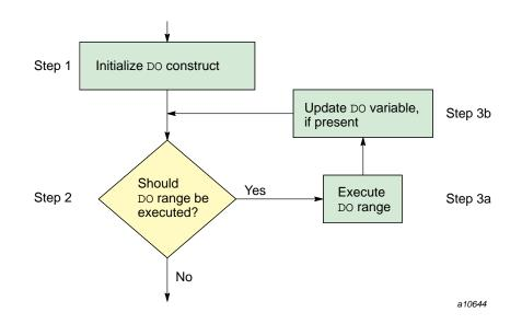
Figure 19. Execution flow for a DO construct
