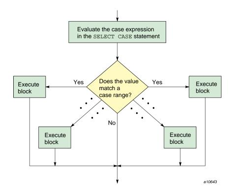
Figure 18. Execution flow for a CASE construct
