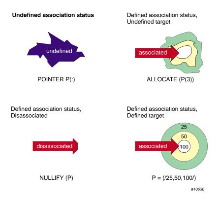
Figure 13. States in the lifetime of a pointer
