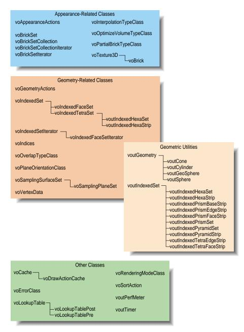
Figure 5-1 Volumizer Class Hierarchy Divided By Function
