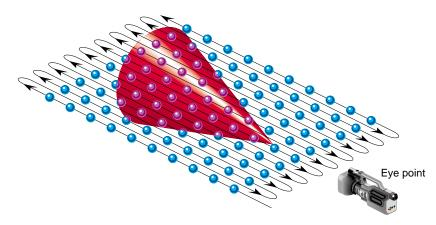
Figure 2-14 Ray Casting Processing order
