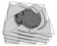
Figure 2-13 Volume Rendering as Texture Mapping
