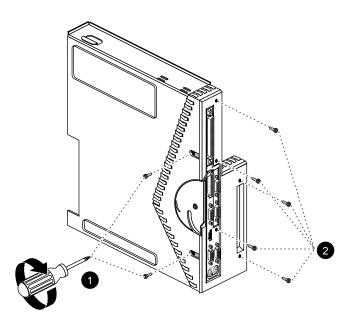
**Figure 1-23** Replacing Screws on the Face Plate
