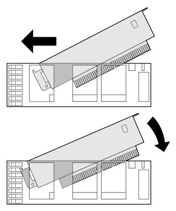
**Figure 1-18** Replacing the PCI Tray in the System Module Viewed From the Side
