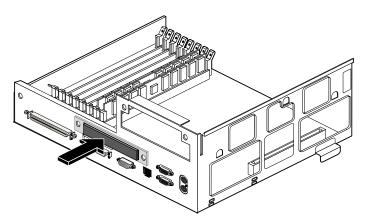
**Figure 1-11** Removing the I/O Slot Panel from the R10000
