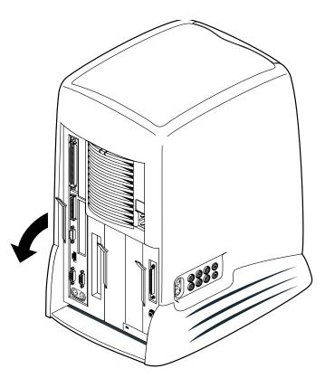
Figure 1-3 Releasing the System Module
