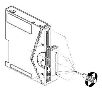
**Figure 1-9** Removing the Screws From the Face Plate
