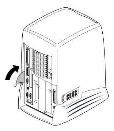
**Figure 1-25** Securing the System Module in Place
