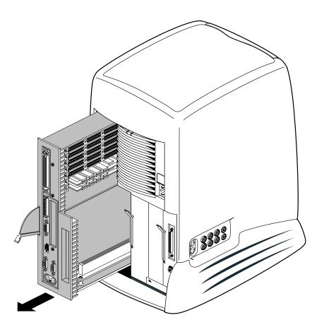
Figure 1-4 Removing the System Module From the Chassis
