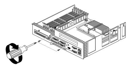
**Figure 1-20** Securing the Option Board
