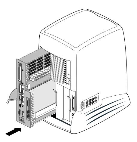
**Figure 1-24** Reinstalling the System Module in the Chassis
