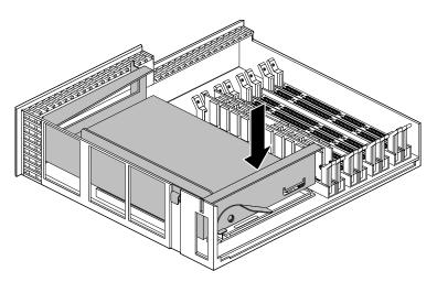
Figure 1-19 PCI Tray Seated Correctly
