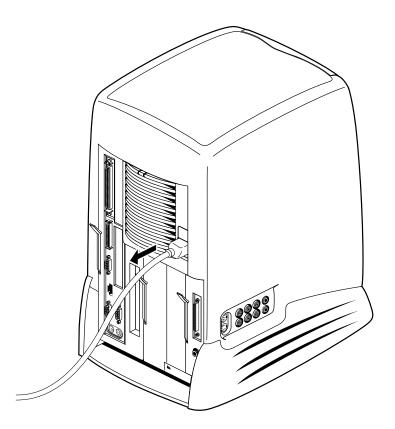
**Figure 1-2** Removing the Power Cable
