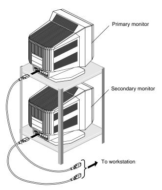
Figure 2-3 Placing the Primary Monitor Above the Secondary Monitor
