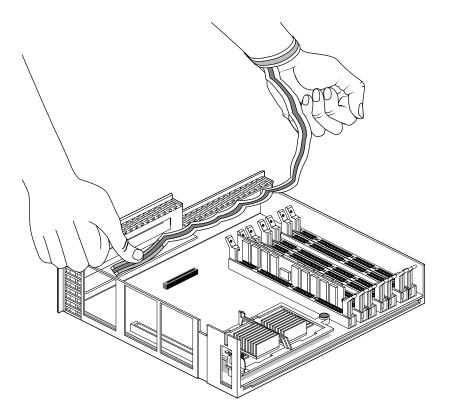
Figure 1-13 Attaching the Wrist Strap
