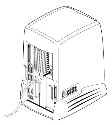
**Figure 1-26** Connecting the Power Cable
