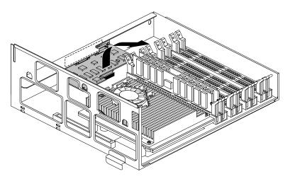
Figure 1-27 Removing the Dual Channel Display Board
