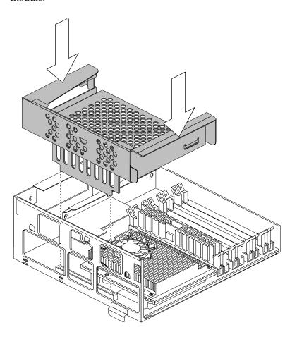
**Figure 1-21** Replacing the R10000 PCI Tray in the System Module
