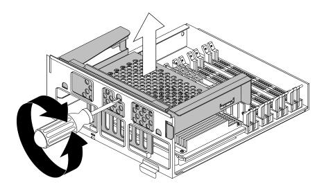
Figure 1-12 Removing the PCI Tray
