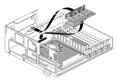
Figure 1-14 Positioning the Option Board
