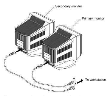
Figure 2-2 Placing the Monitors Side by Side
