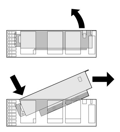
**Figure 1-7** Removing the PCI Tray From the System Module Viewed From the Side
