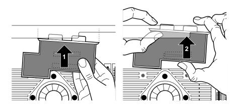
Figure 1-15 Aligning the Option Board
