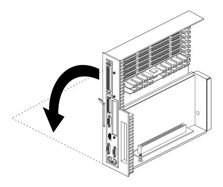
**Figure 1-5** Laying the System Module Flat
