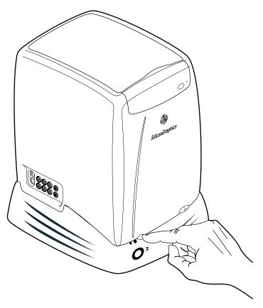
Figure 2-6 Turning On the O2 Workstation
