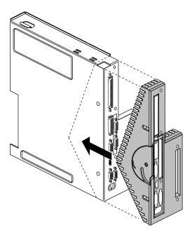
Figure 1-22 Replacing the Face Plate
