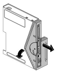
**Figure 1-10** Removing the Face Plate from the R10000
