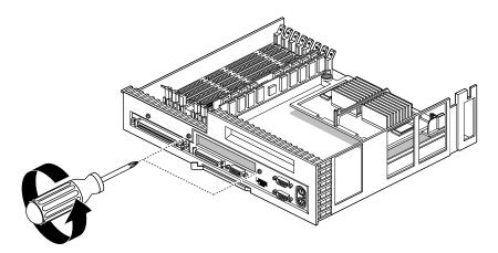
**Figure 1-8** Removing the I/O Slot Panel from the R5000
