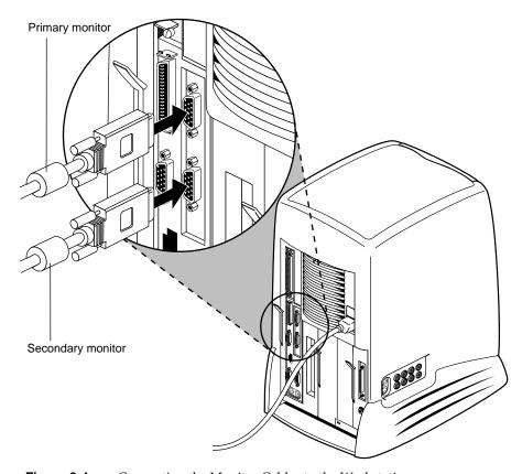
**Figure 2-4** Connecting the Monitor Cables to the Workstation
