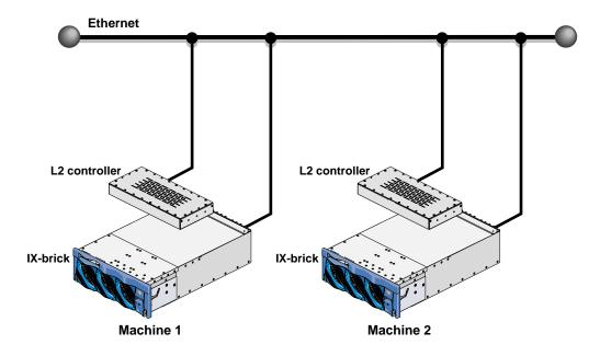
Figure 2-1 Altix 3700 L2 with an Ethernet Connection
