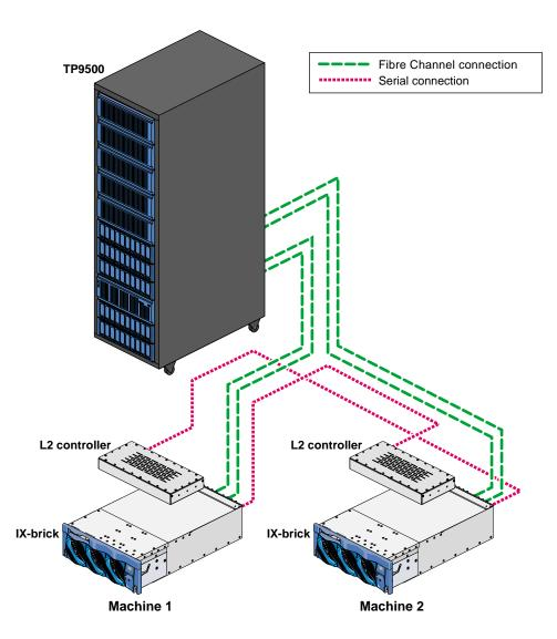
Figure 2-5 Altix 3700 L2 with Serial Cable Connection
