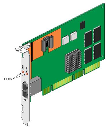
Figure 1-1 Gigabit Ethernet Board (PCI Version)
