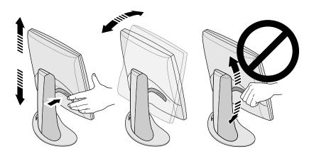
**Figure 1-3** Adjusting the Height and Tilt
