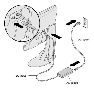
**Figure 1-2** Connecting the Power Cable and AC Adapter
