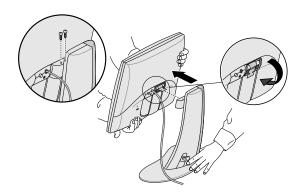
Figure 1-4 Removing the Monitor From Its Base
