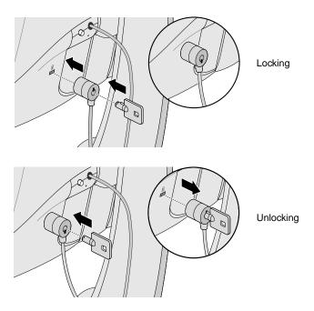
Figure 1-6 Locking and Unlocking the Monitor
