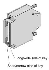
Figure 3-1 GSN Loopback Device
