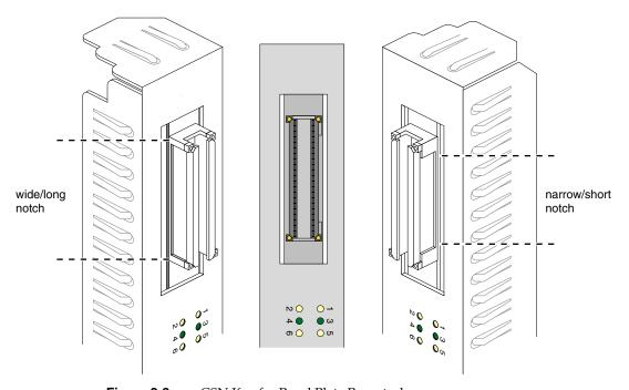
**Figure 2-3** GSN Key for Panel Plate Receptacle
