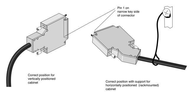
Figure 2-5 GSN Cable Connectors for Origin 200 Gigachannel Expansion Cabinet
