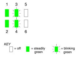
**Figure 1-4** LED Behavior on Main SGI GSN Board During Normal Operation
