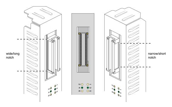
Figure 1-2 GSN Key in Panel Plate Receptacle
