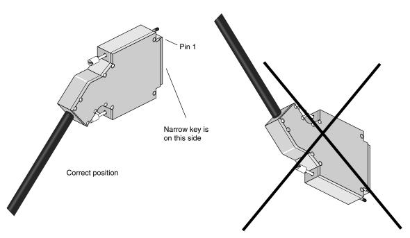
Figure 2-4 GSN Cable Connector for Origin 2000 and Onyx2 Modules
