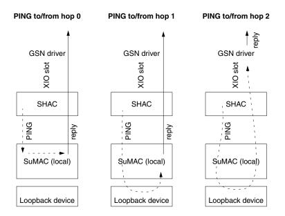
**Figure 3-2** Hops Involved in *gsntest* With External Loopback Device
