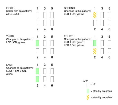
Figure 1-3 LED Behavior on Main SGI GSN Board During Normal Power-on
