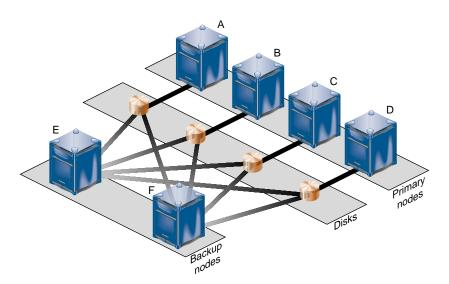
**Figure 4-2** *N*+2 Configuration Concept
