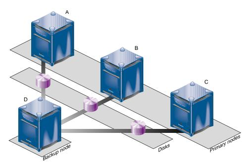
**Figure 4-1** *N*+1 Configuration Concept
