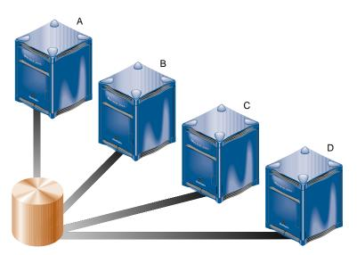
**Figure 4-3** *N+M* Configuration Concept
