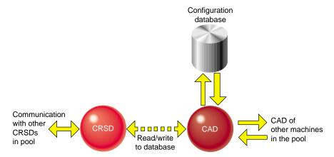
Figure 1-4 Communication Path for a Node that is Not in a Cluster
