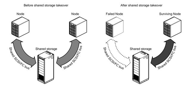
Figure 1-8 Disk Storage Failover on a Two-Node System
