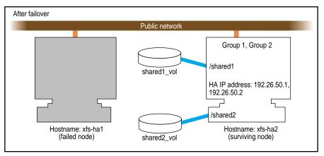
Figure 2-4 Shared Disk Configuration For Dual-Active Use
