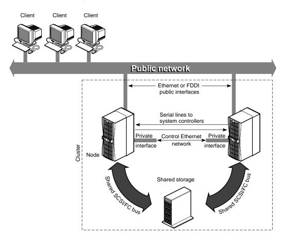
Figure 1-5 Sample System Components
