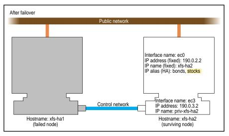
Figure 3-1 Example Interface Configuration
