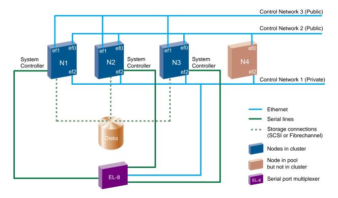
Figure 6-1 FailSafe Configuration Example
