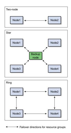
Figure 1-6 Configuration Types
