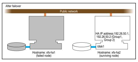
Figure 2-2 Non-Shared Disk Configuration and Failover
