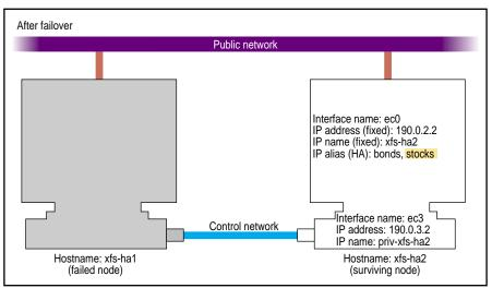
Figure 4-1 Example Interface Configuration
