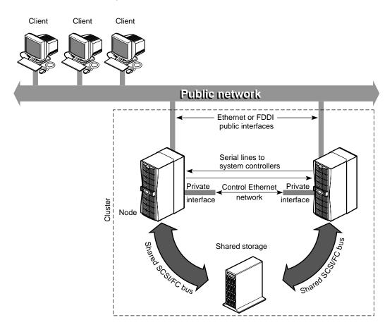
Figure 1-5 Sample System Components
