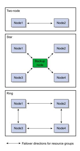
Figure 1-6 Configuration Types
