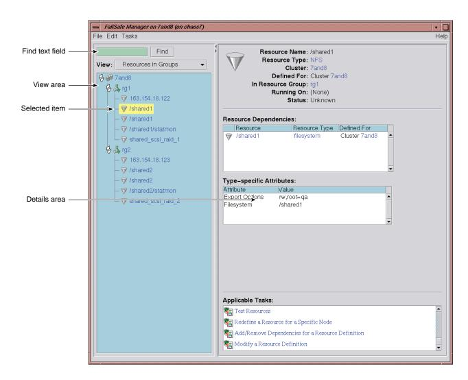
Figure 5-1 GUI Showing Details for a Resource
