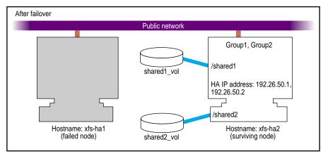
Figure 2-4 Shared Disk Configuration for Dual-Active Use
