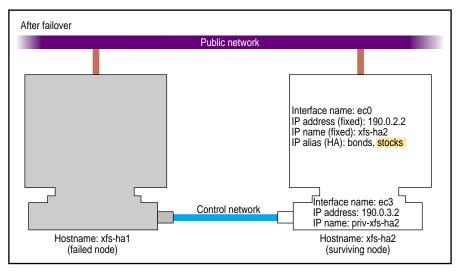
Figure 4-1 Example Interface Configuration
