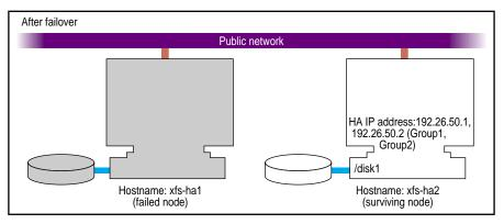
Figure 2-2 Non-Shared Disk Configuration and Failover
