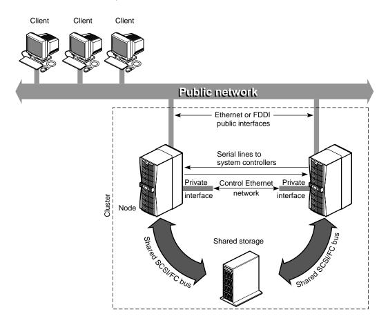
Figure 1-5 Sample System Components
