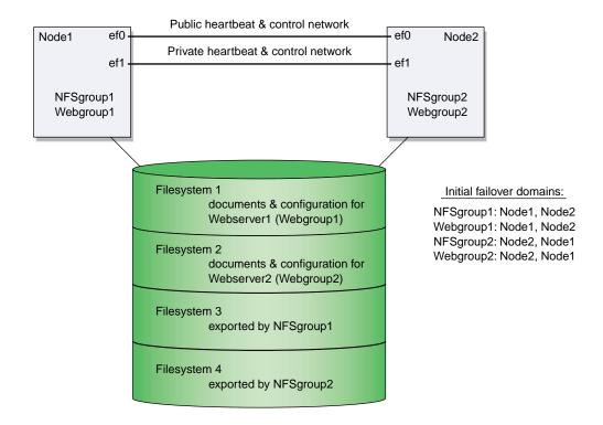
Figure 2-1 Example Configuration with Four Resource Groups
