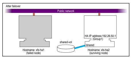
Figure 2-3 Shared Disk Configuration for Active/Backup Use
