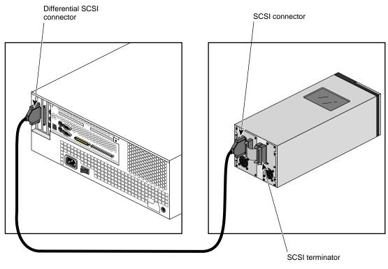
Figure 3 shows an example of a DLT 7000 eight-slot autoloader connected to an optional differential PCI SCSI board on the back of an Origin200 server.
