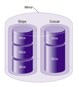
Figure 1-17 shows a mirror composed of a stripe and a concat.
