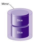
Figure 1-15 shows a mirror that is composed of two slices.
