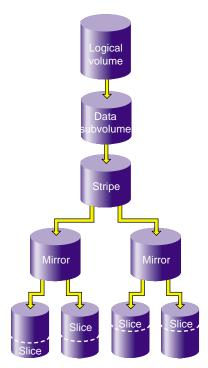
Figure 6-29 XVM Logical Volume after Mirroring Slices
