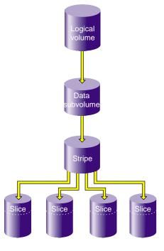
Figure 6-2 Striping a Portion of a Disk
