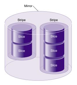
Figure 1-16 Mirror Composed of Two Stripes
