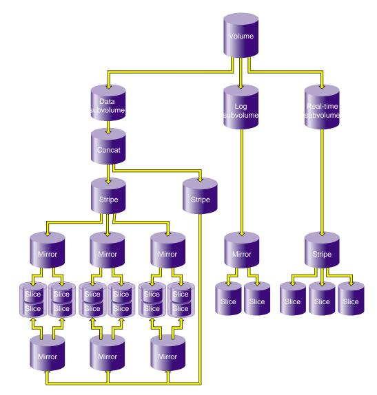
Figure 1-7 XVM Logical Volume after Insertion of Concat
