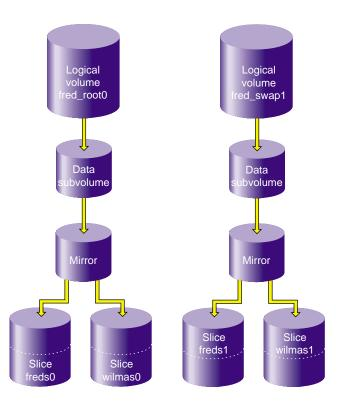
The slices that are created on physvolwilma are inserted as mirrors into the existing root and swap logical volumes, as shown in Figure 4-4.
