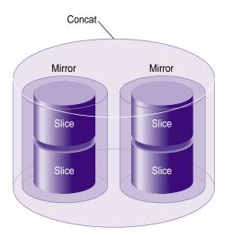
Figure 1-12 shows a concat that is composed of two mirrors.
