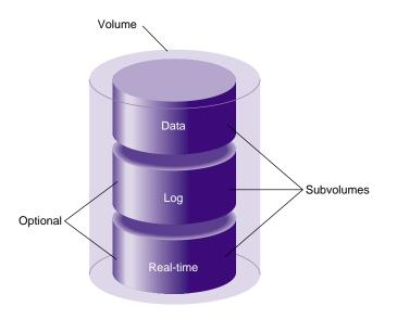
Figure 1-8 shows an XVM volume with system-defined subvolume types.
