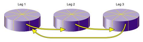
Figure 2-3 Reading Data from a Mirror with a Round-Robin Read Policy
