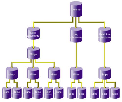
Figure 1-6 shows an XVM logical volume with three subvolumes and a mirrored stripe in the data subvolume.
