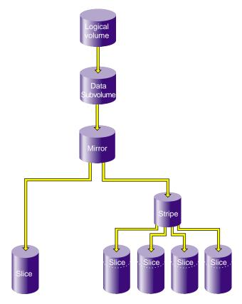
Figure 6-21 Filesystem after Attaching Stripe to Mirror
