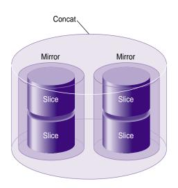
Figure 1-13 shows a concat that is composed of two mirrors.
