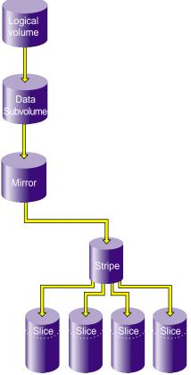
Figure 7-22 Filesystem after Detaching Original Slice
