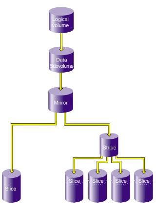
Figure 7-21 shows the configuration of the filesystem myfs after the stripe has been attached to the mirror.
