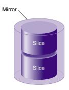
Figure 1-16 Mirror Composed of Two Slices
