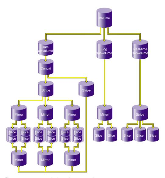
**Figure 1-8** XVM Logical Volume after Insertion of Concat
