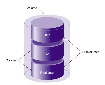
Figure 1-9 shows an XVM volume with system-defined subvolume types.
