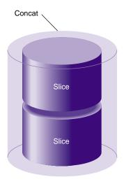
Figure 1-12 Concat Composed of Two Slices
