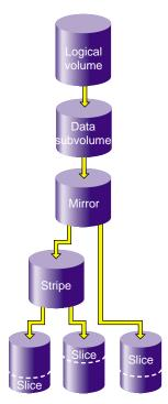
Figure 7-27 XVM Logical Volume after Conversion from Concat to Mirror
