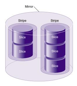
Figure 1-17 Mirror Composed of Two Stripes
