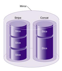
**Figure 1-18** Mirror Composed of a Stripe and a Concat
