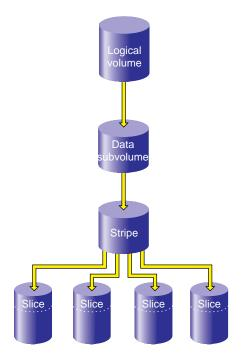
Figure 7-2 Striping a Portion of a Disk
