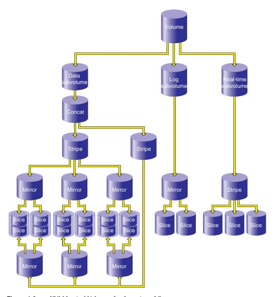
Figure 1-9 XVM Logical Volume after Insertion of Concat
