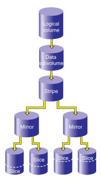
Figure 7-29 XVM Logical Volume after Mirroring Slices
