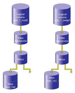
Figure 7-10 XVM Disk Logical Volumes after Insertion of Mirror Components
