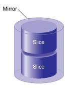
**Figure 1-17** Mirror Composed of Two Slices
