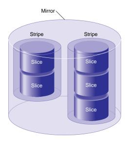
**Figure 1-18** Mirror Composed of Two Stripes
